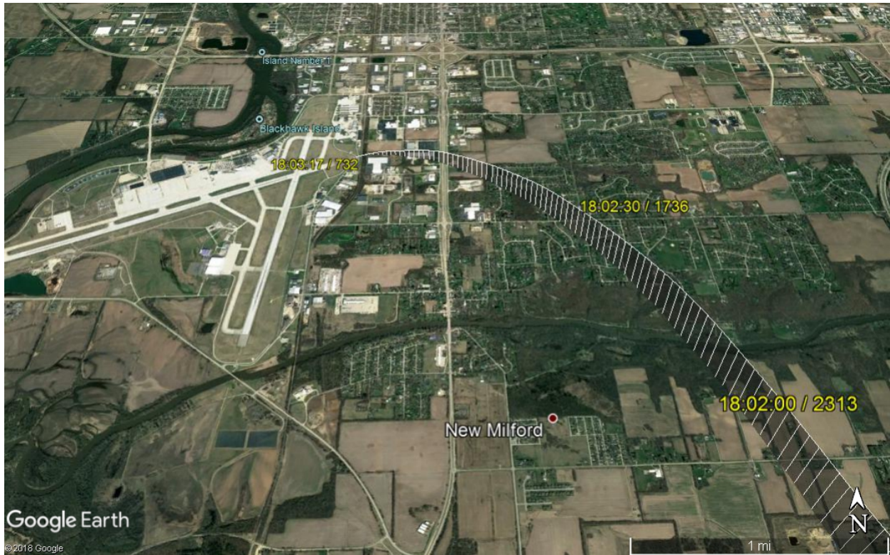
Figure 4: Google Earth overlay of December 4, 2017 flight to Chicago/Rockford International Airport in Rockford, Illinois. Times are shown in CST, recorded altitude in feet. Data has been down-sampled to once per second.
