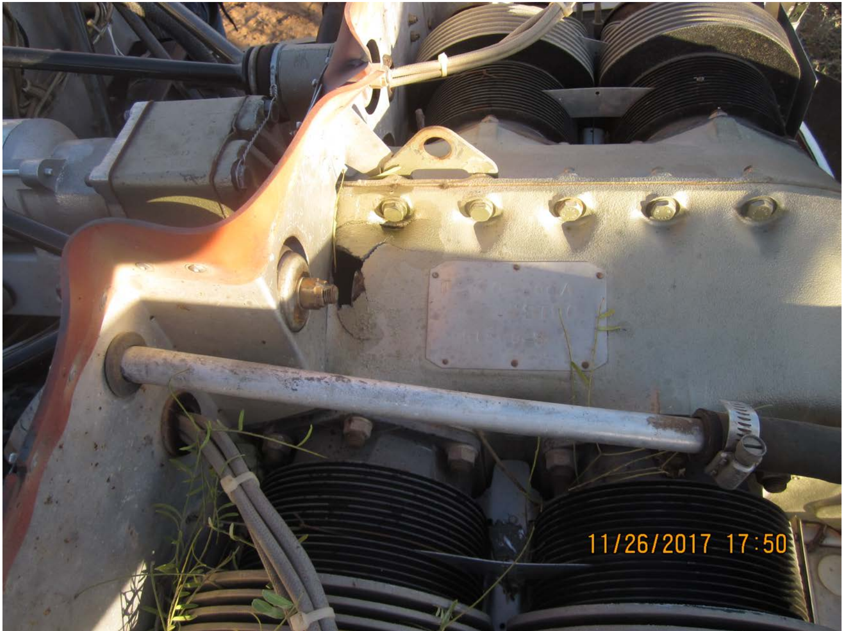
Photo 5 – Hole above #1 cylinder
