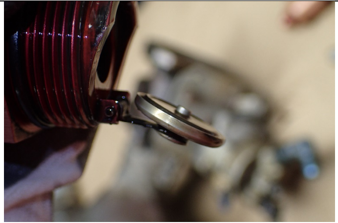
Scavenge oil check valve not closing automatically
