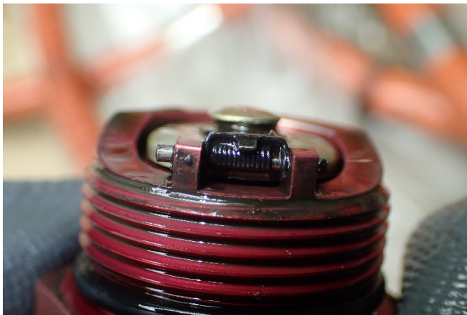
Broken oil scavenge check valve spring
