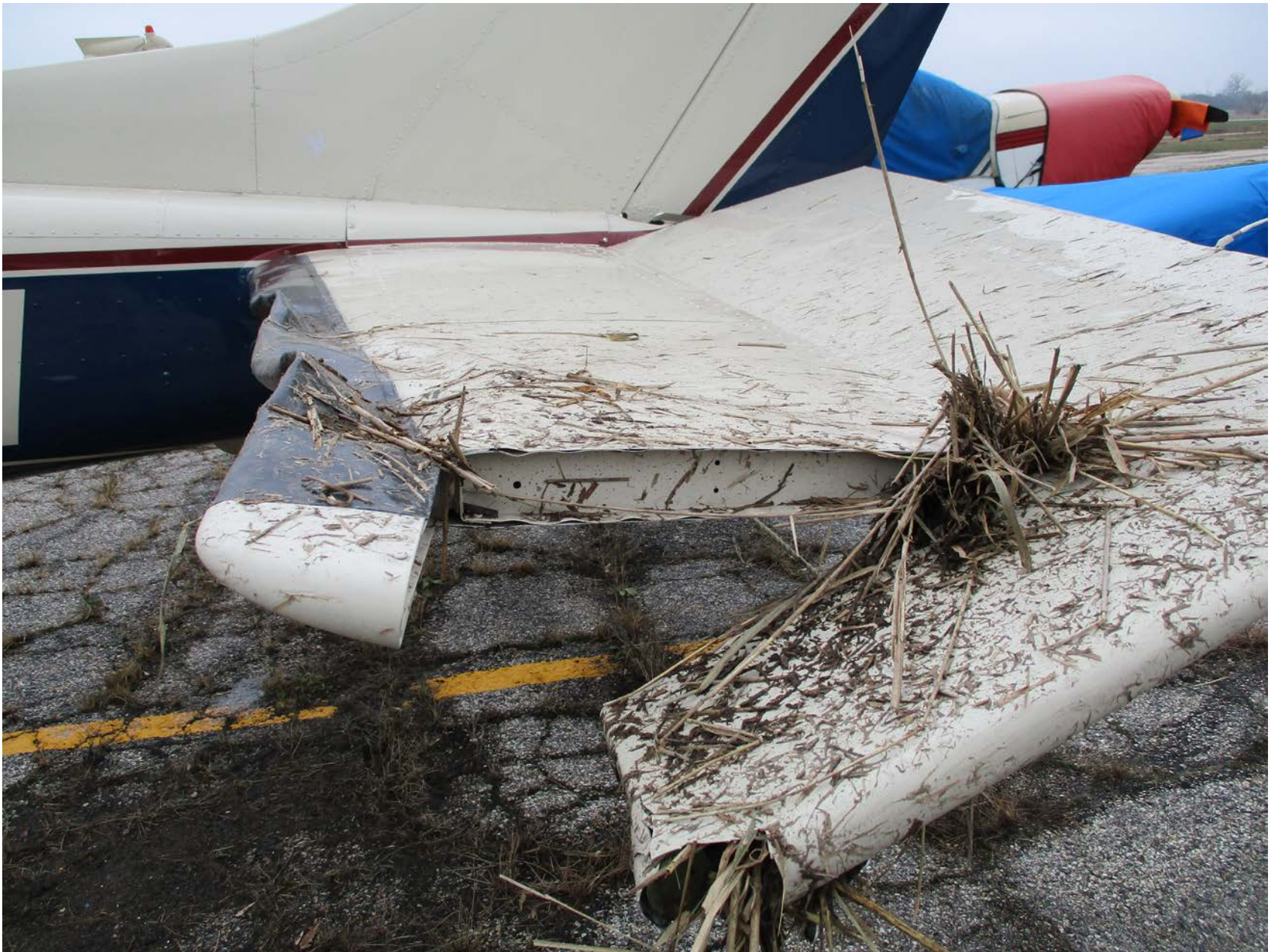
Photo 3 – Damaged left elevator
