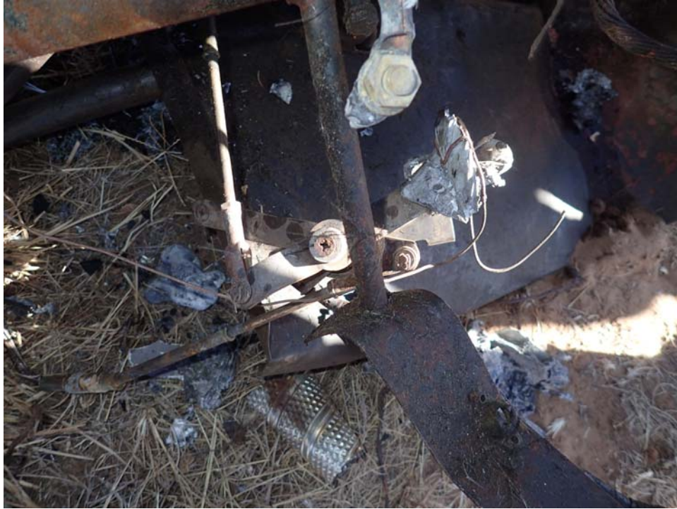
Remaining Portion of the Cockpit Engine Controls with Cables Attached
