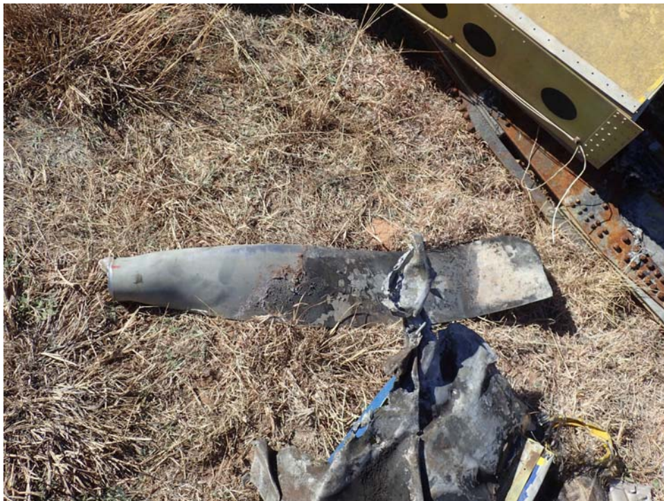
Separated Propeller Blade
