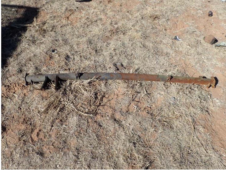
Flap Torque Tube with Hardware Intact
