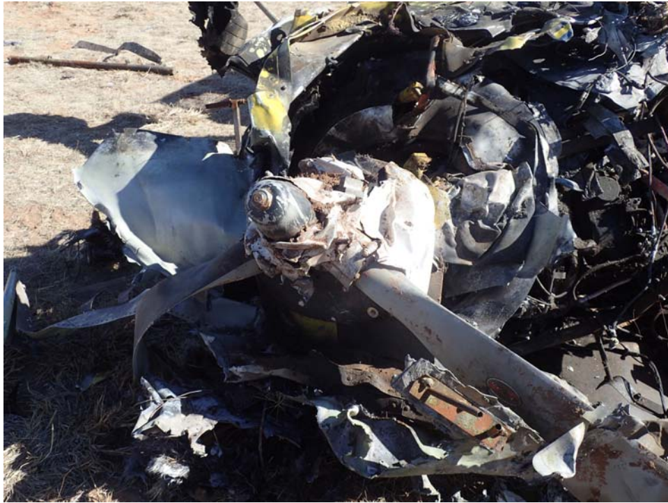
Propeller and Engine Wreckage
