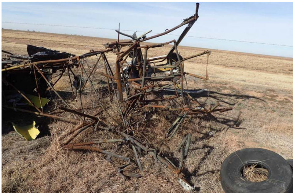
Fuselage Wreckage with Aileron Controls
