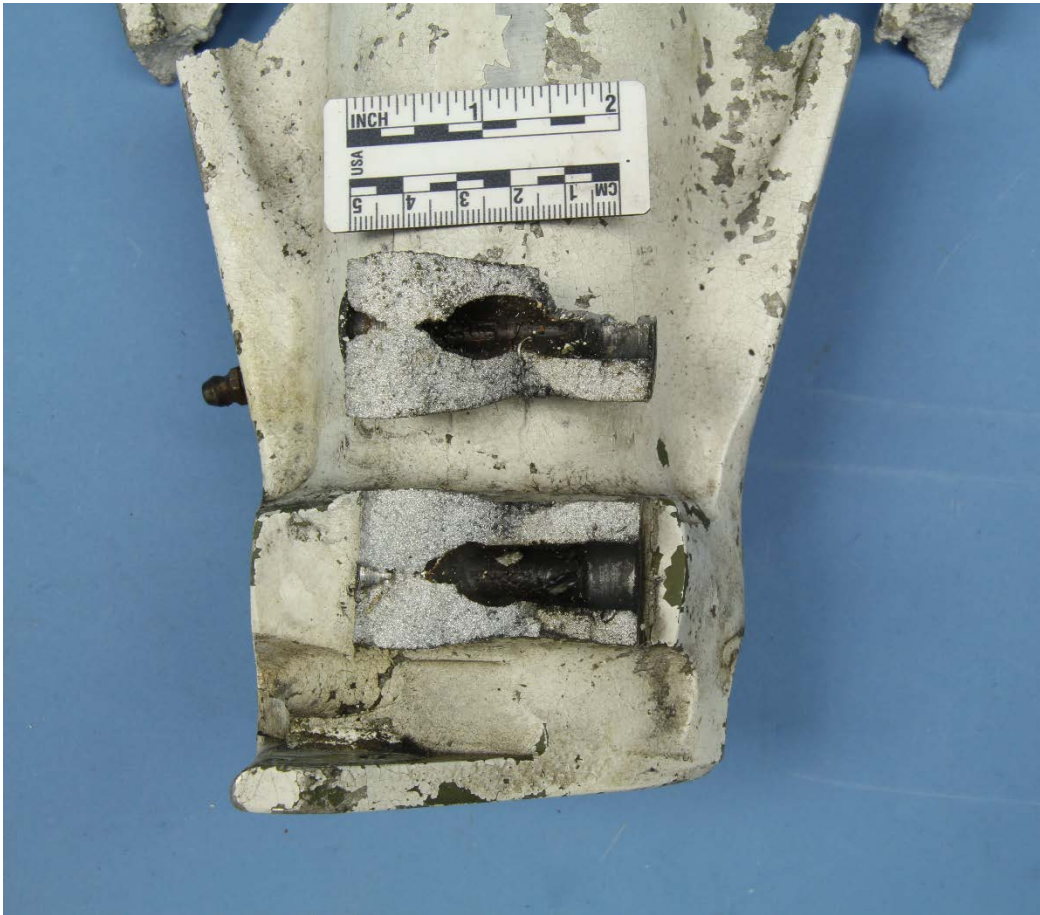
Figure 2: Both halves of bolt hole fracture on trunnion casting.
