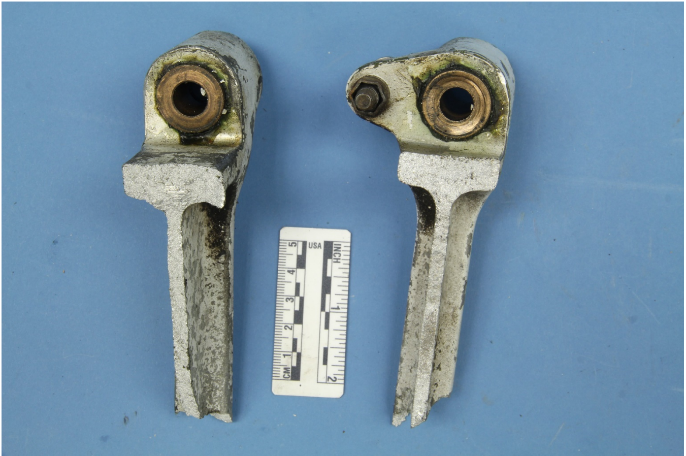
Figure 3: Fractures pivot arms of trunnion casting.
