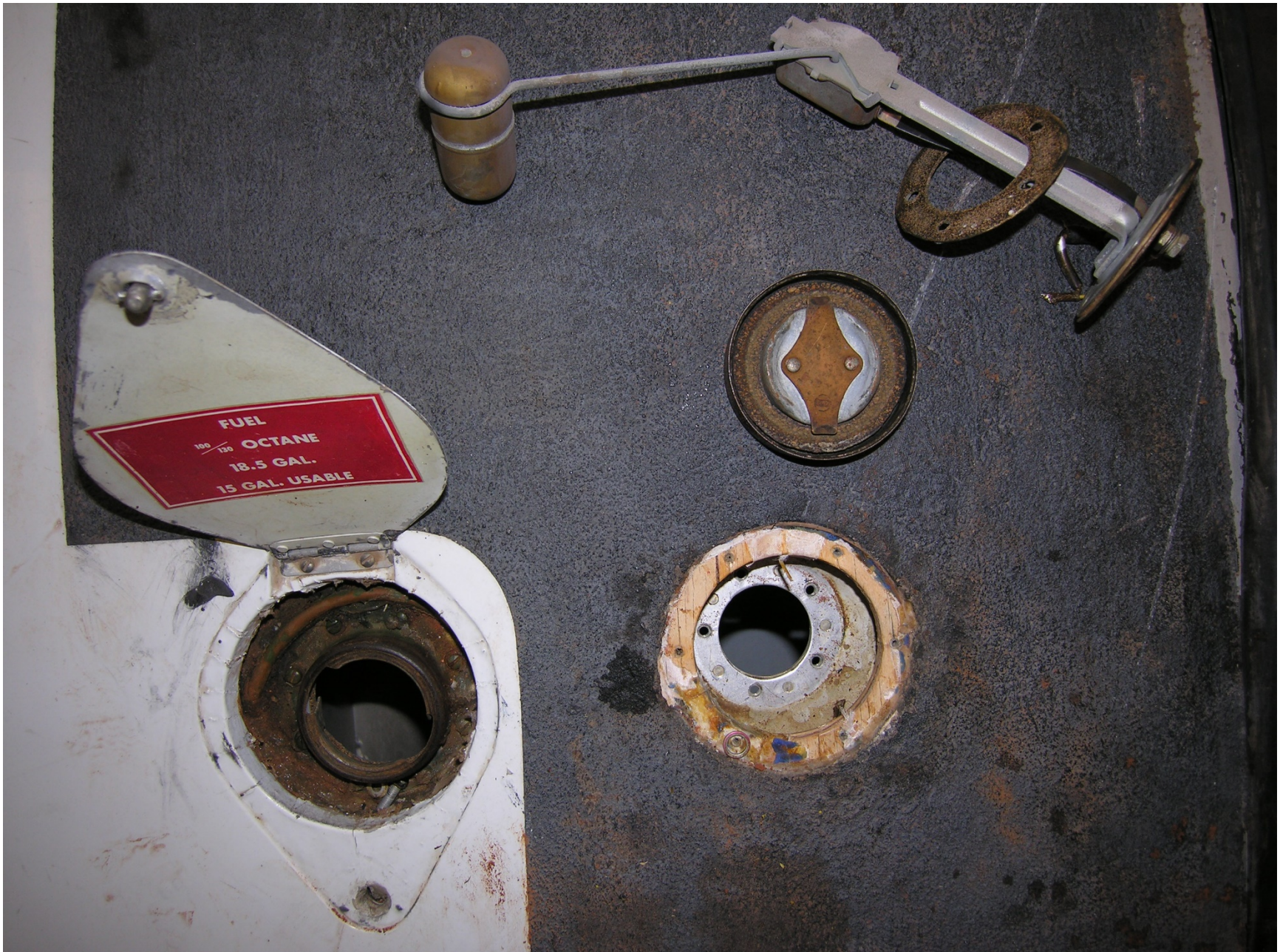
Photo 3 – Corrosion of Wing Tank Filler Neck, Cap, and Fuel Sender
