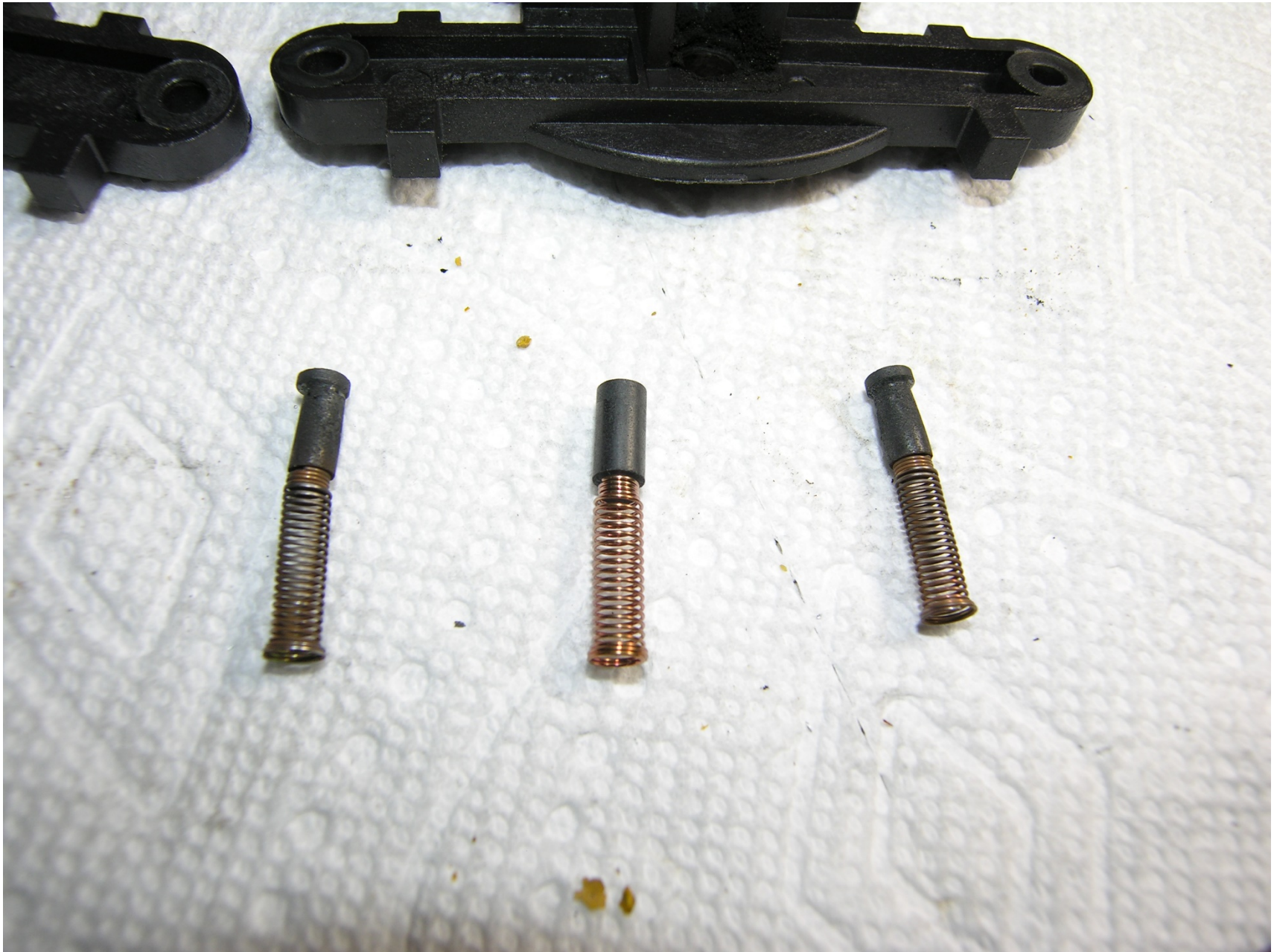
Photo 2 – Left, New, and Right Magneto Brushes
