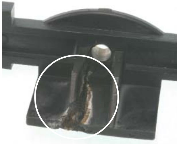
Unacceptable (Developing bearing bar failure)
