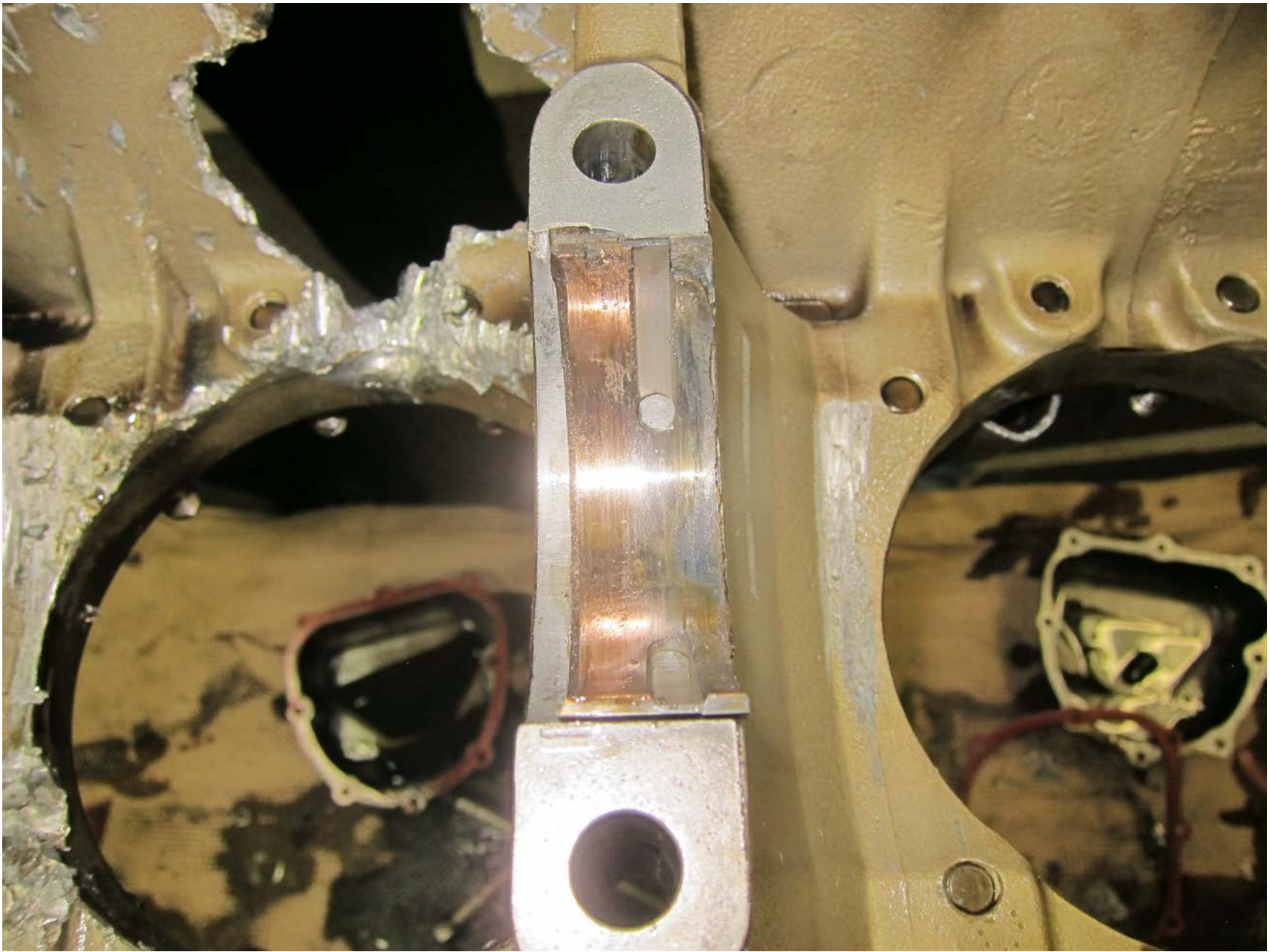
Photo 5 – View of No. 2 main bearing (CM Photo)
