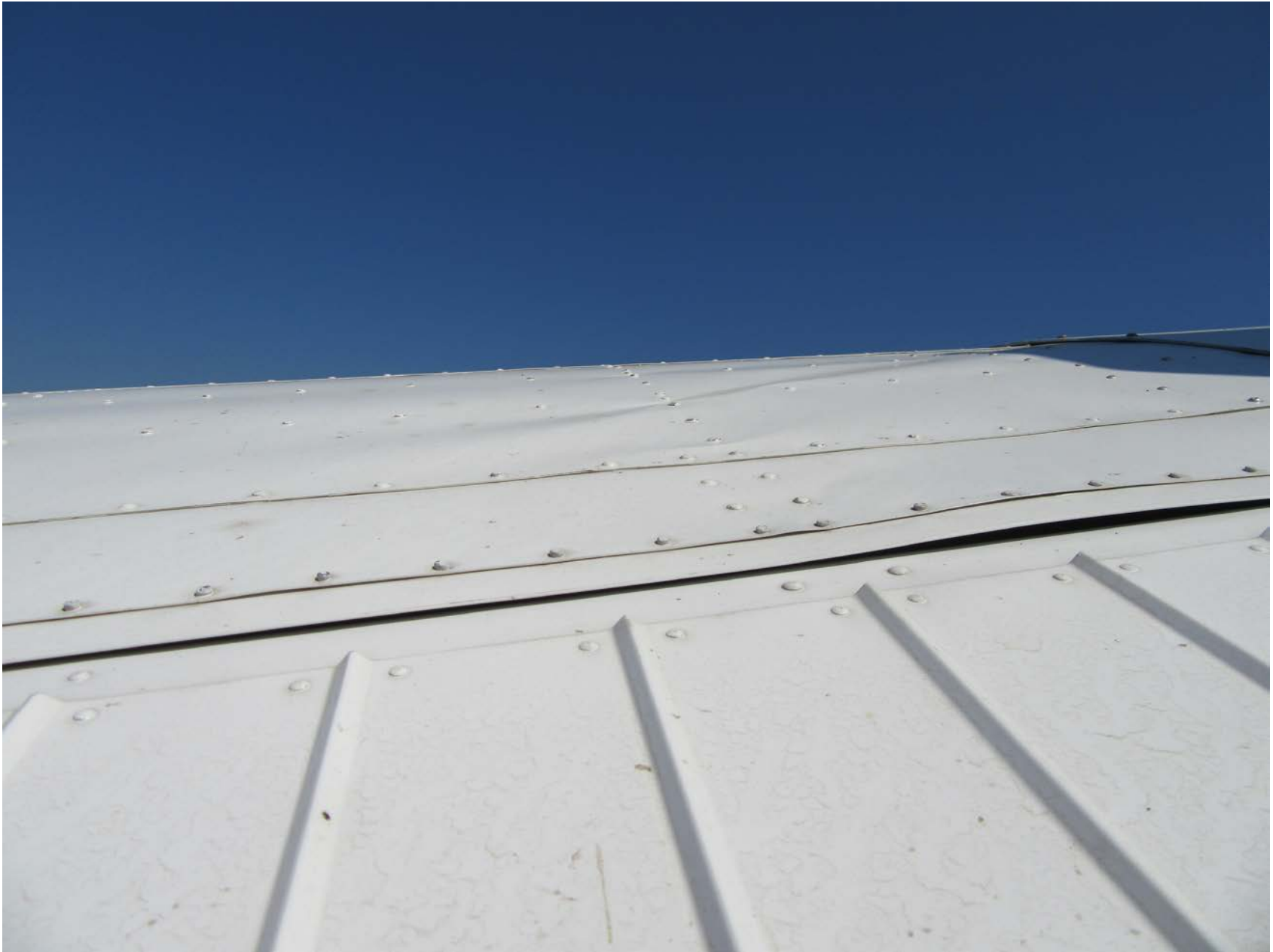
Photo 2 – View of minor damage to the right wing (FAA Photo)
