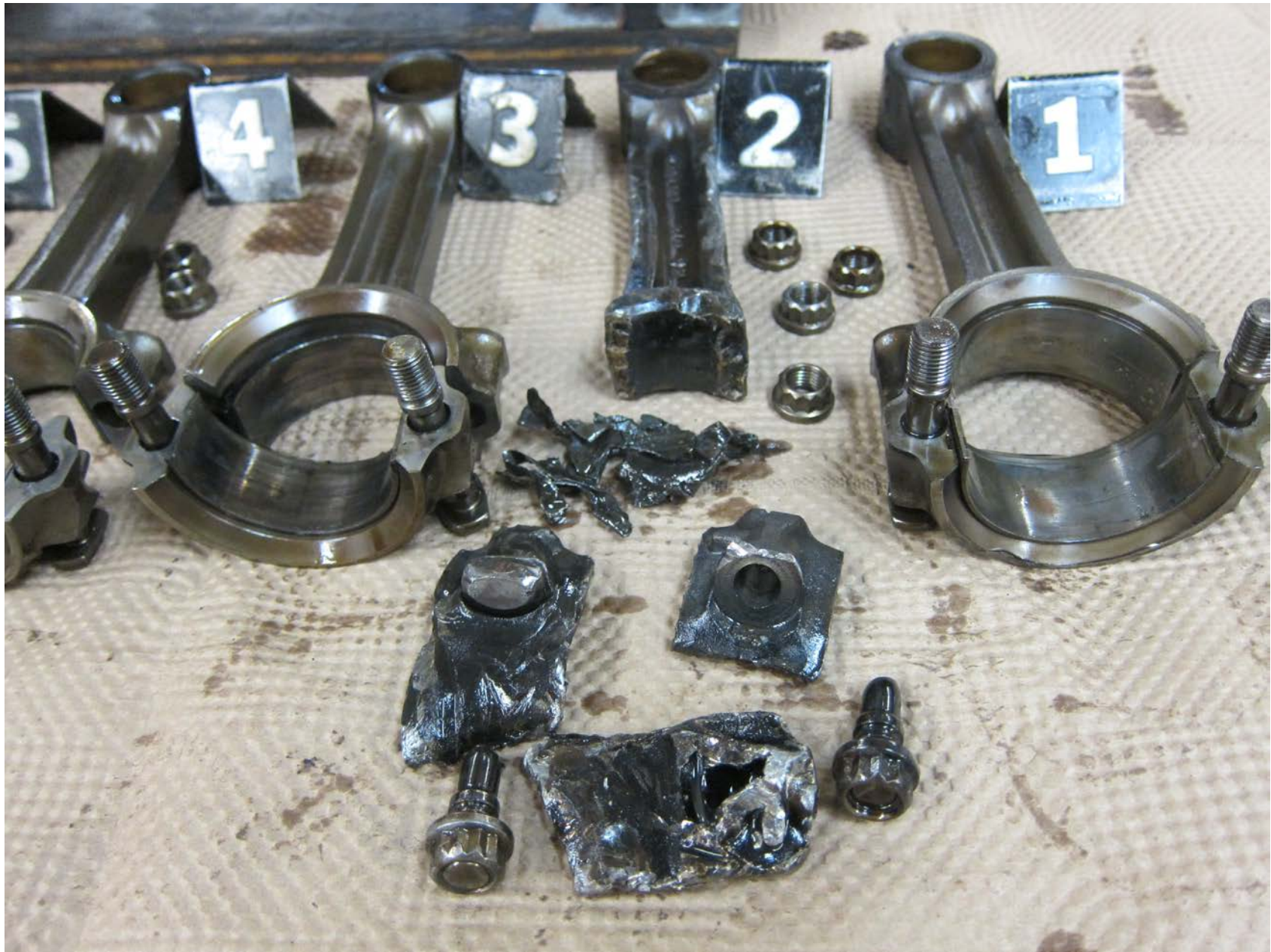
Photo 4 – View of damage to the No. 2 piston connecting rod (CM Photo)
