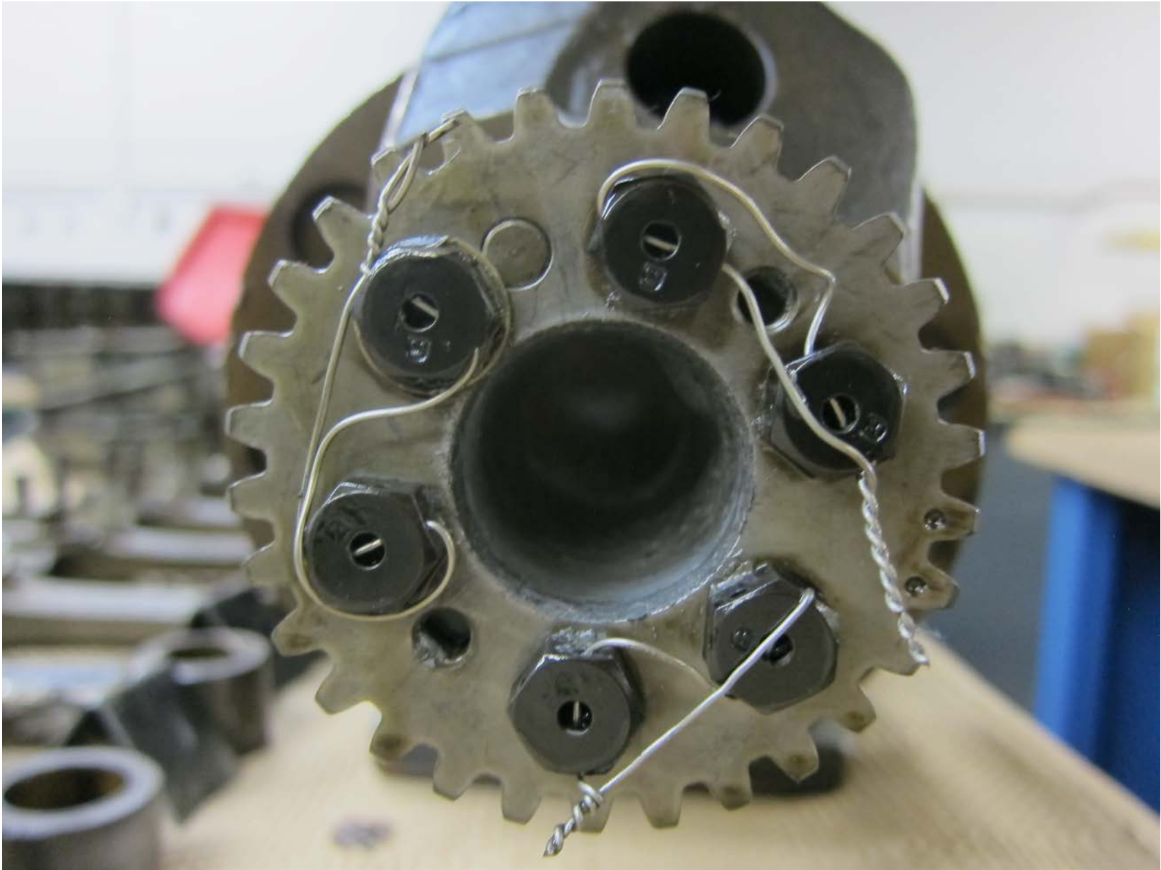
Photo 11 – View of the crankshaft gear and the safety wire (CM Photo)
