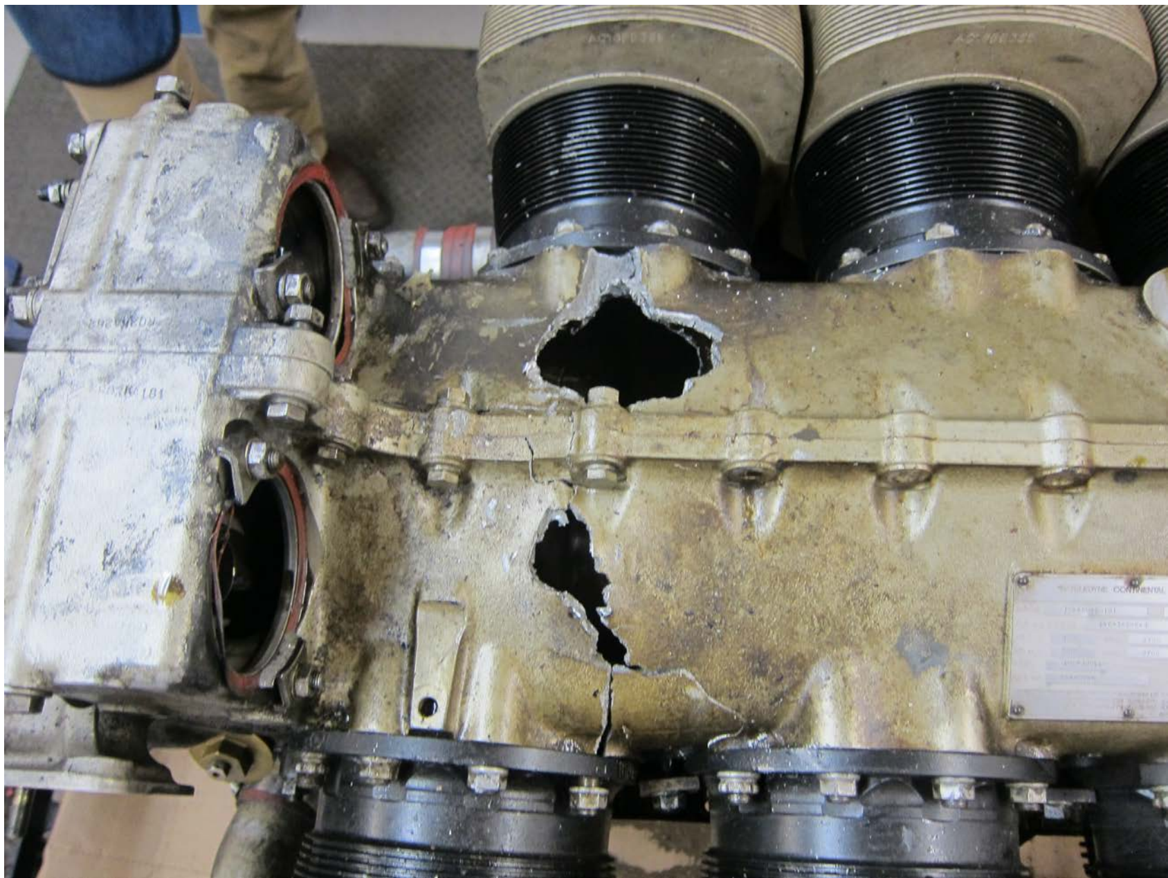
Photo 3 – View of the hole in the crankcase (CM Photo)
