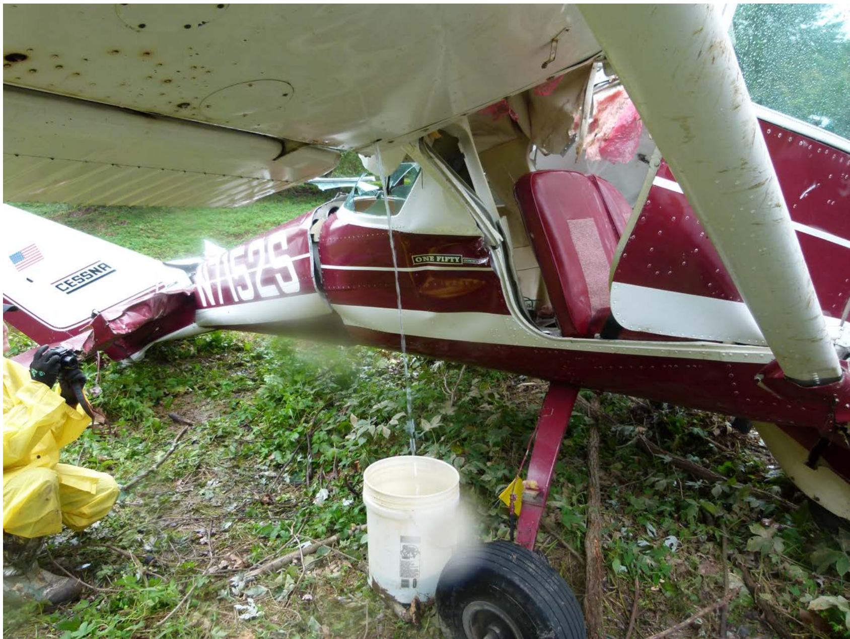
Photo 6 – View of the fuel being extracted to a five-gallon plastic bucket (courtesy of Continental Motors).
