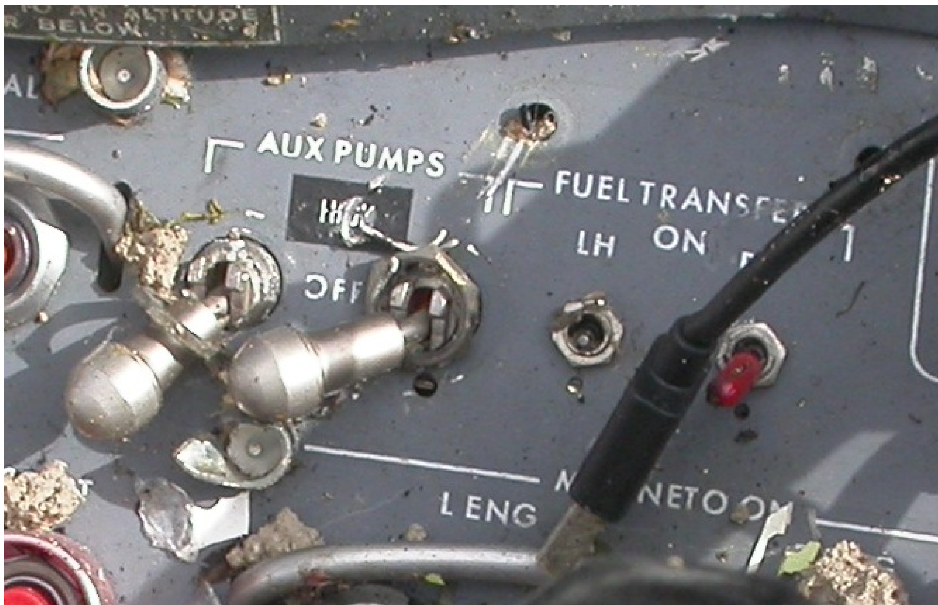
Photo 1 – View of Aux Pump and Fuel Transfer Switches (Cessna Photo)
