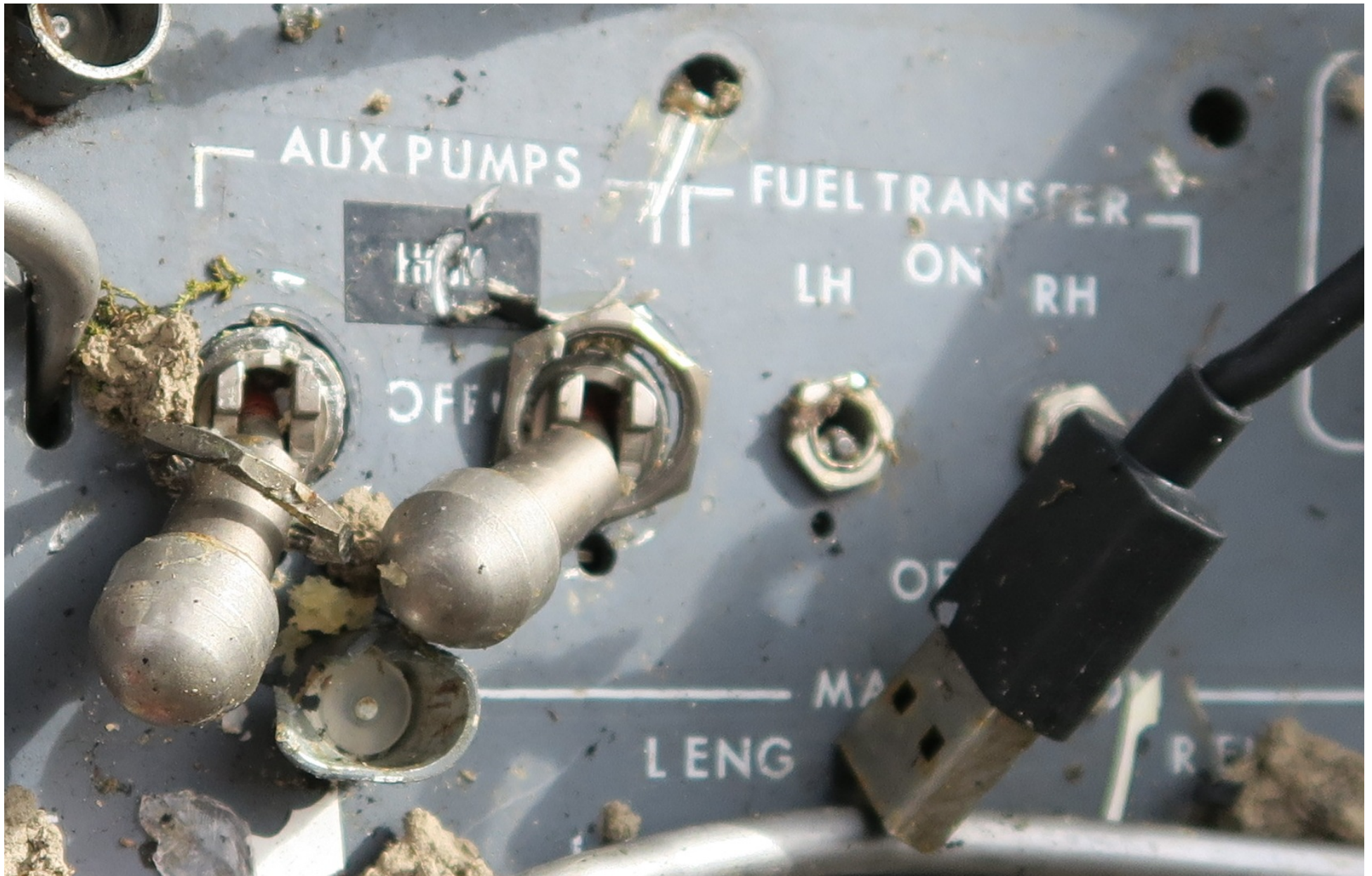
Photo 2 - View of Aux Pump and Fuel Transfer Switches (Cessna Photo)
