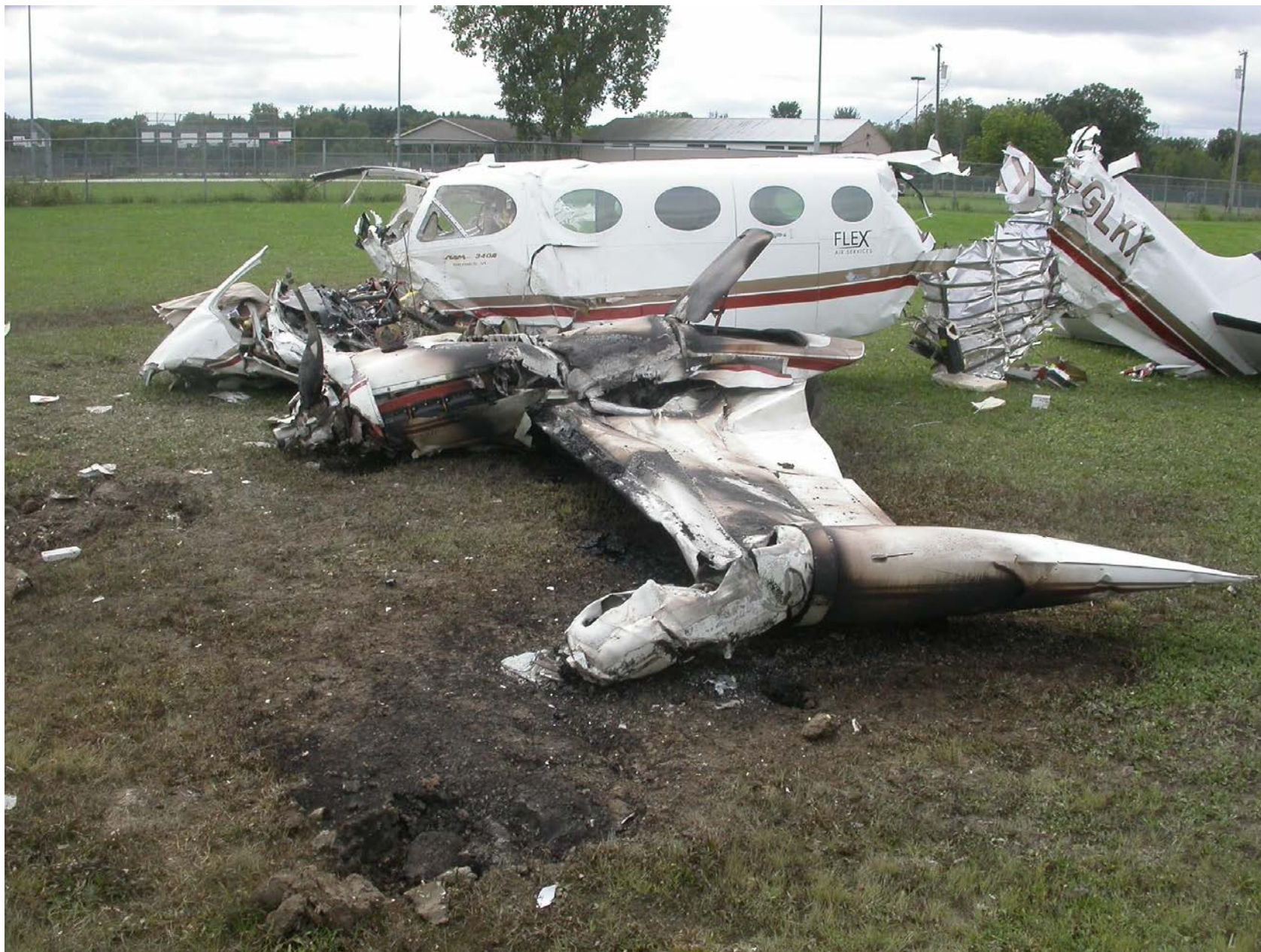
Photo 12 – View of the right wing that had fire damage
