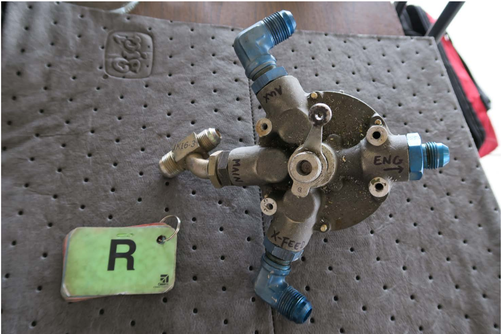
Photo 18 – Cockpit right engine fuel selector valve (Textron photo)
