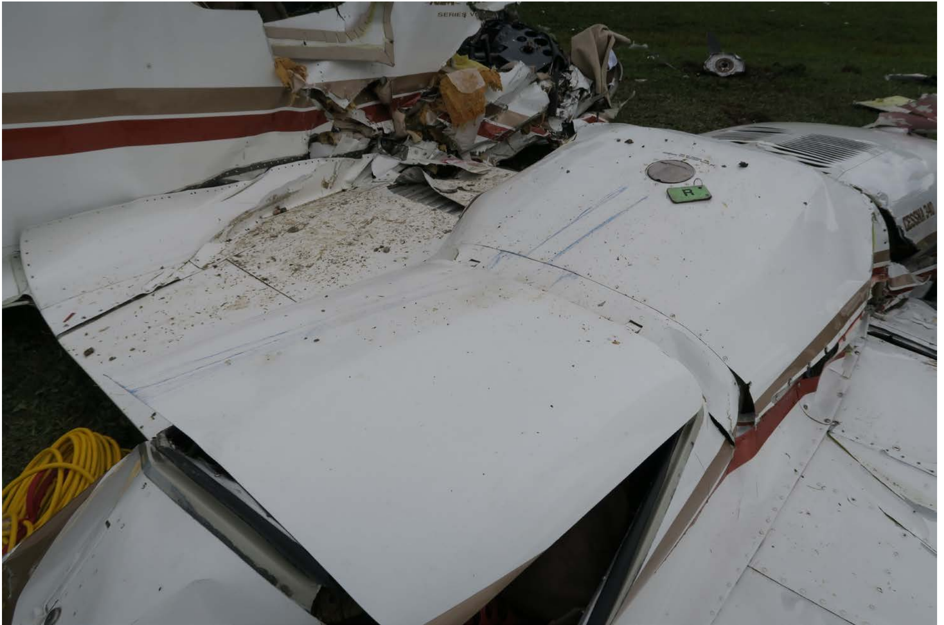
Photo 7 – View of the top of the right nacelle fuel tank and cargo locker (Textron photo)
