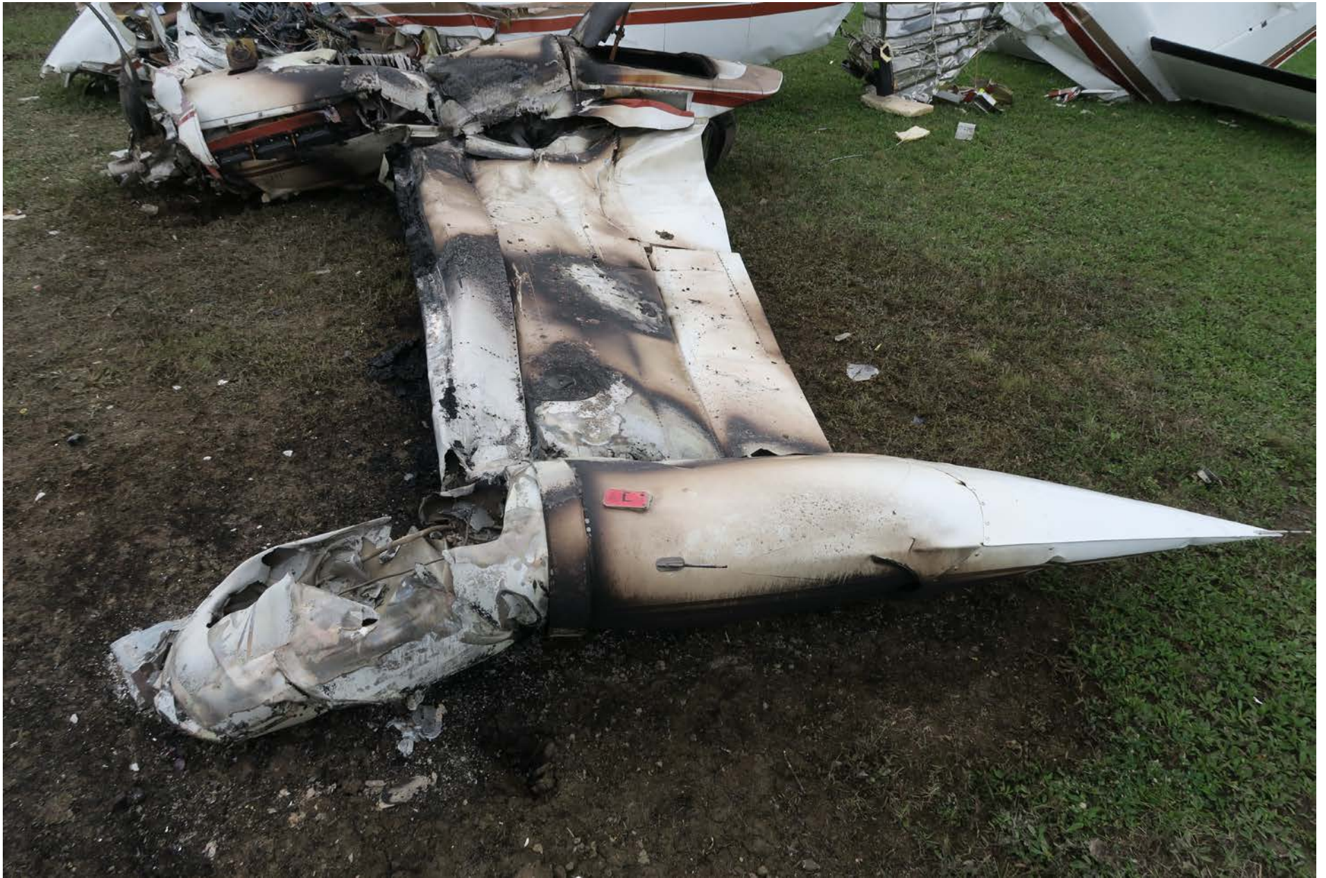
Photo 13 – View of fire damage to the left wing
