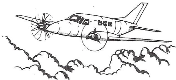
Figure 16-6 Windmilling Propeller Creates Drag
