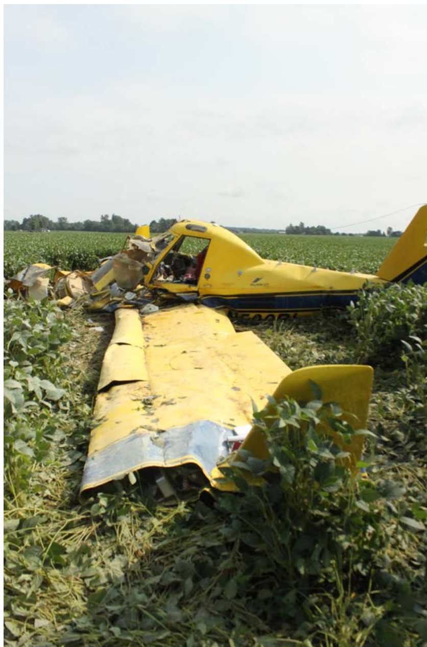
Photo 3 – Left Wing Leading Edge Crushing
