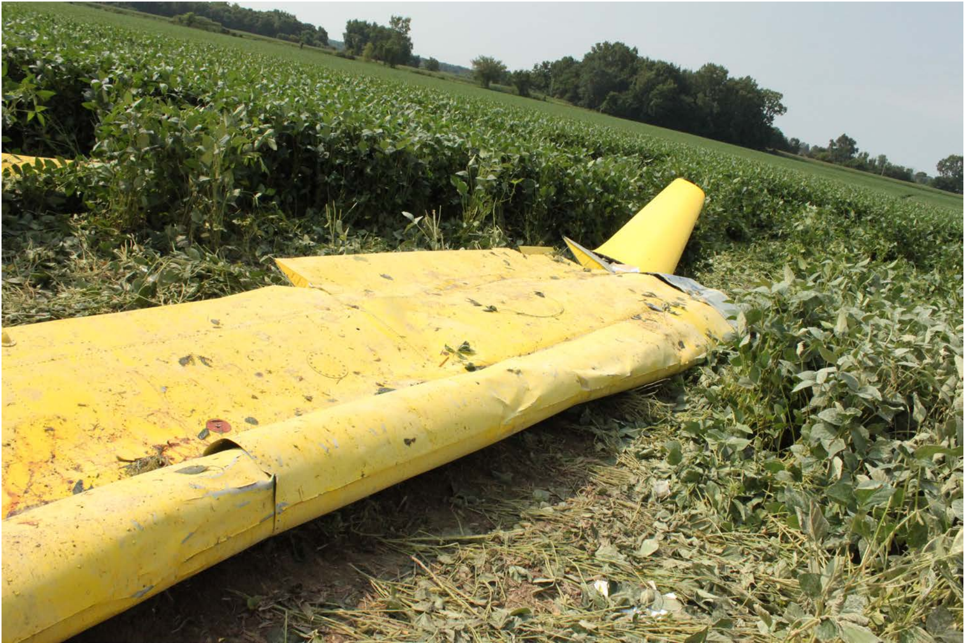
Photo 6 – Left Wing Leading Edge Crushing
