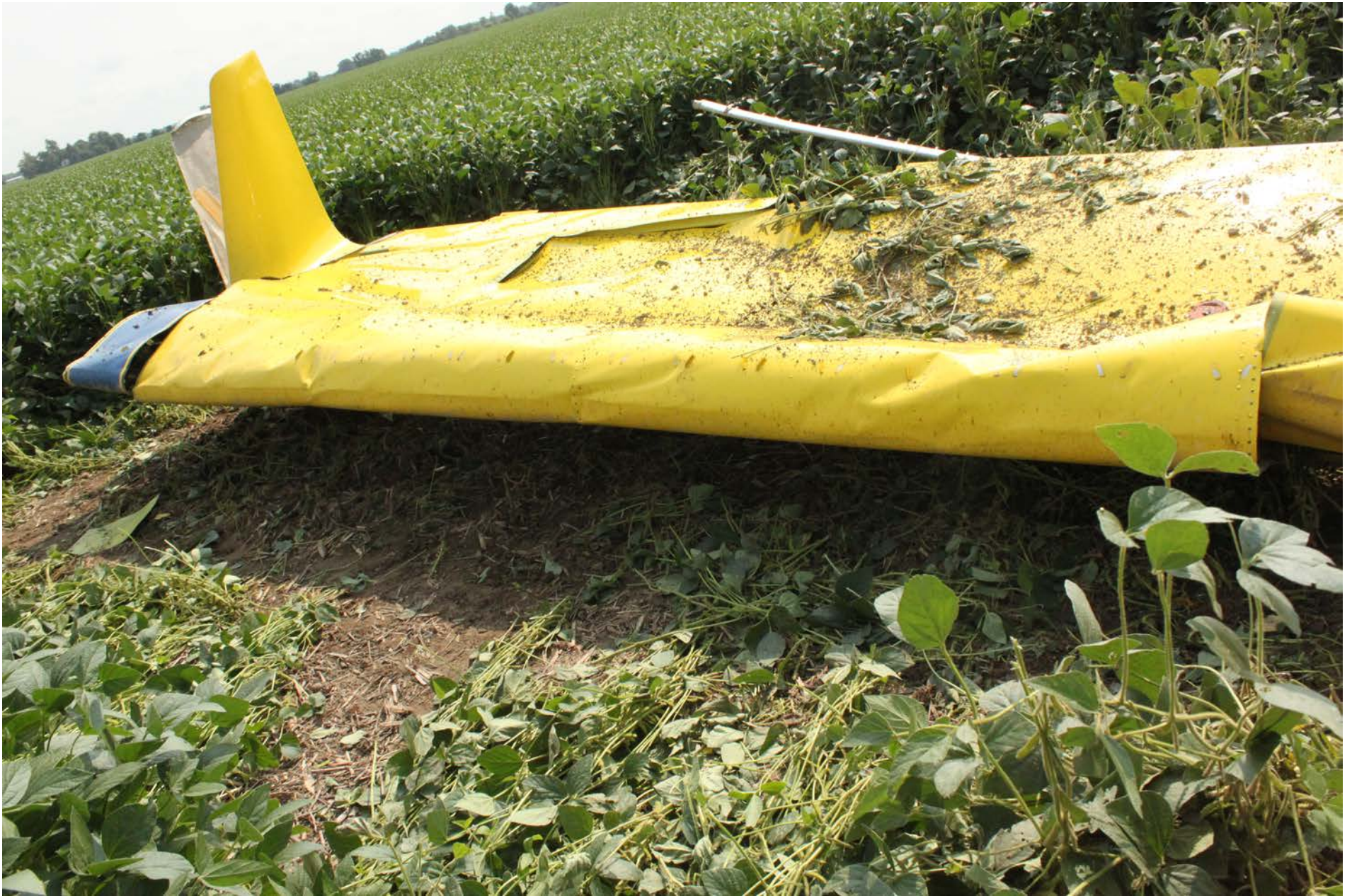
Photo 5 – Right Wing Leading Edge Crushing
