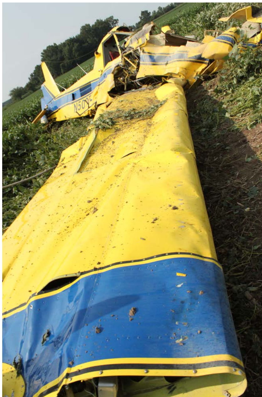
Photo 4 – Right Wing Leading Edge Crushing
