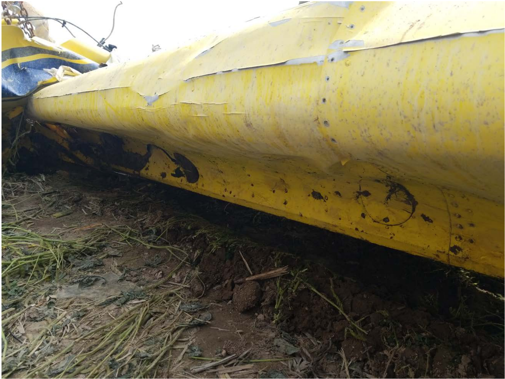
Photo 7 – Left Wing Leading Edge Crushing
