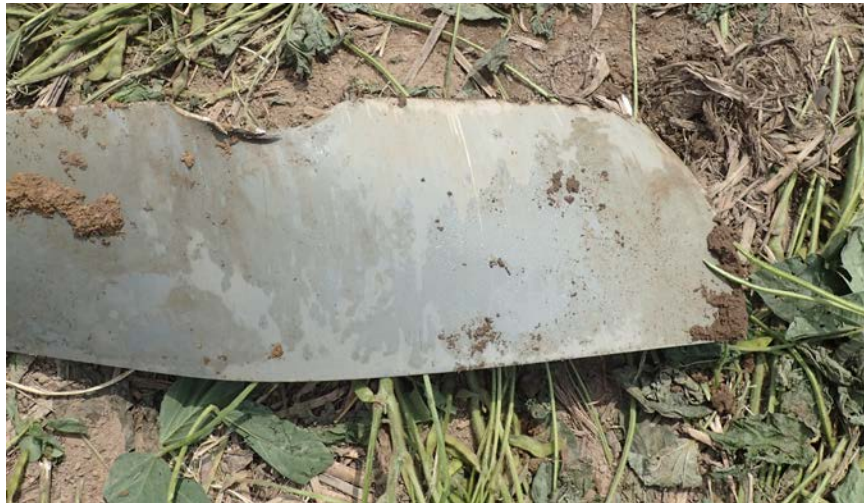
Detail of Separated Propeller Blade
