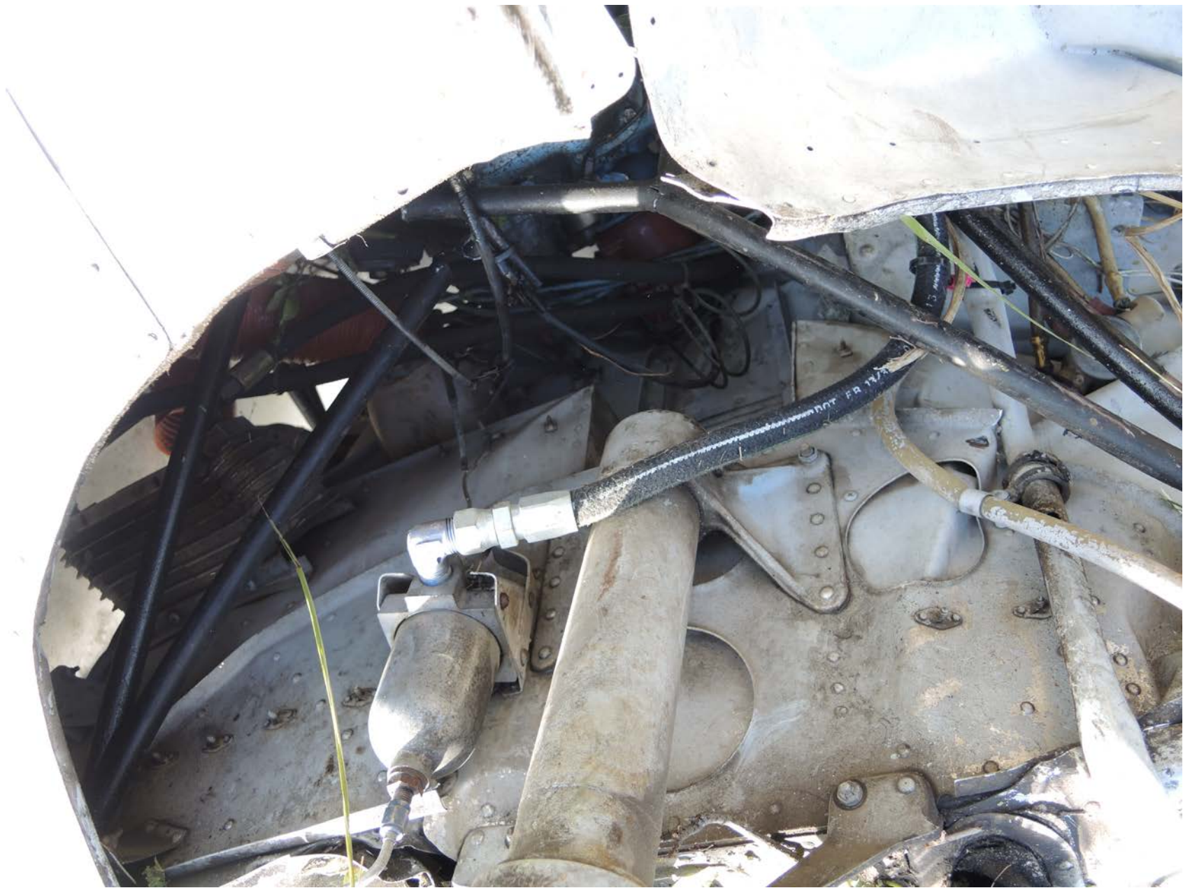
Photo 8 – Gascolator and Hydraulic Line
