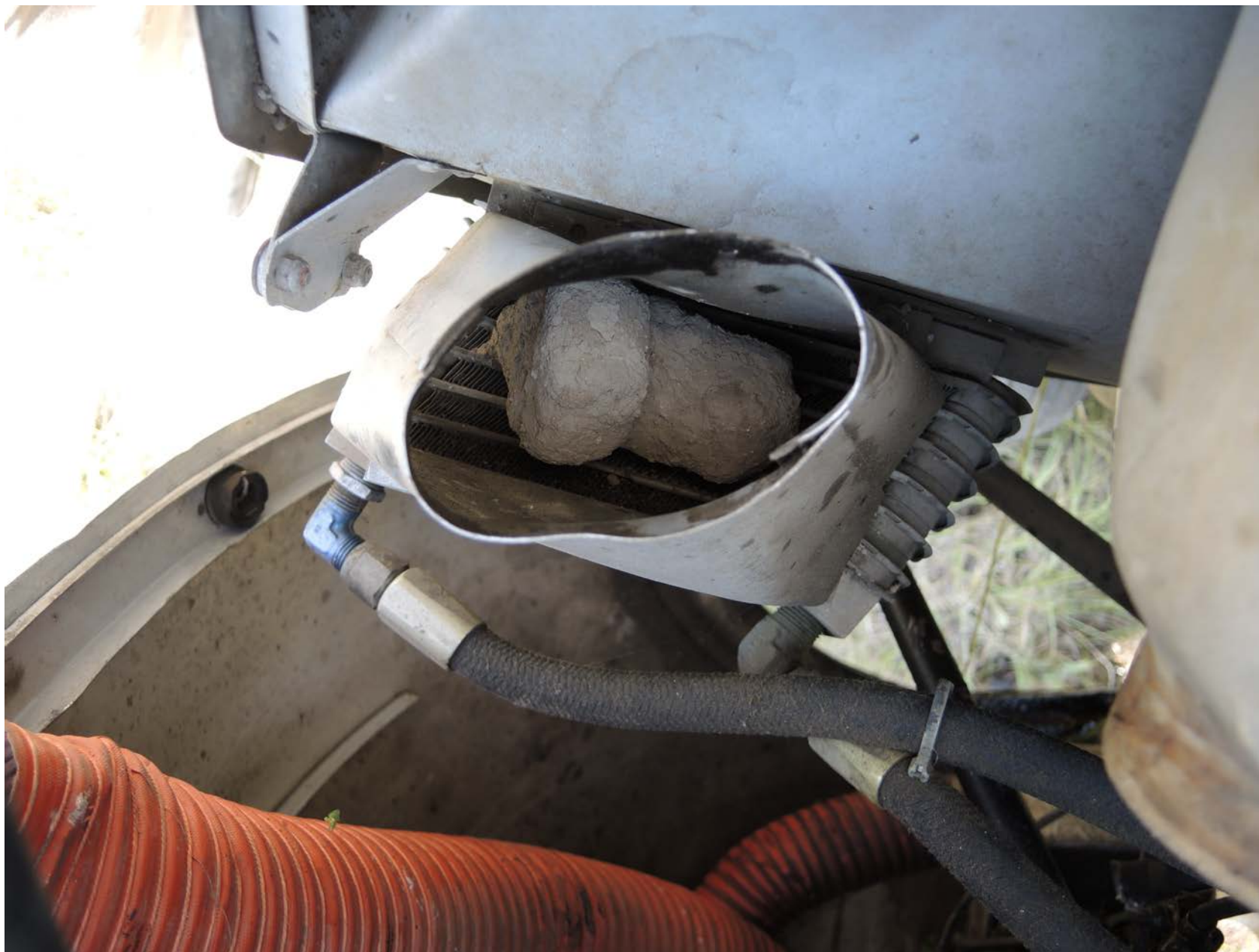
Photo 11 – Mud Dauber Nest In Oil Cooler
