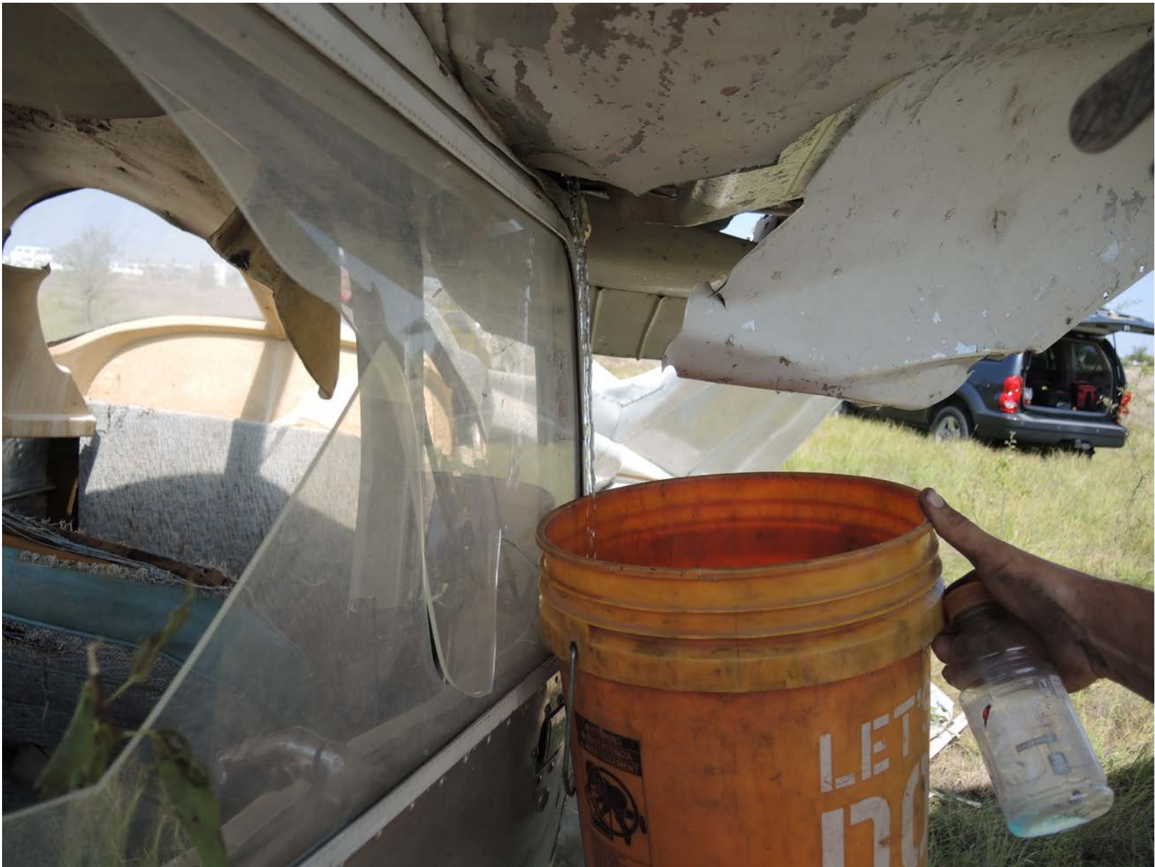
Photo 12 – Fuel Drained From Left Wing Tank
