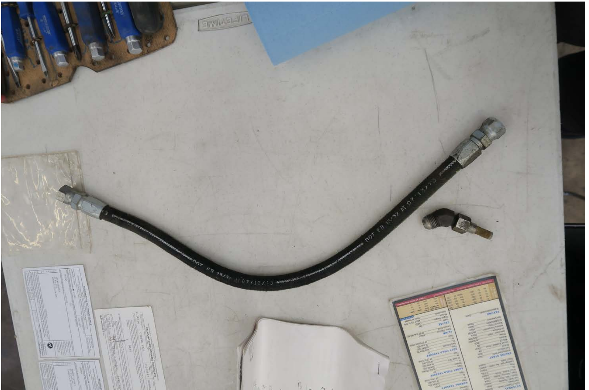
Photo 15 – Automotive Hydraulic Hose Used As Main Fuel Line
