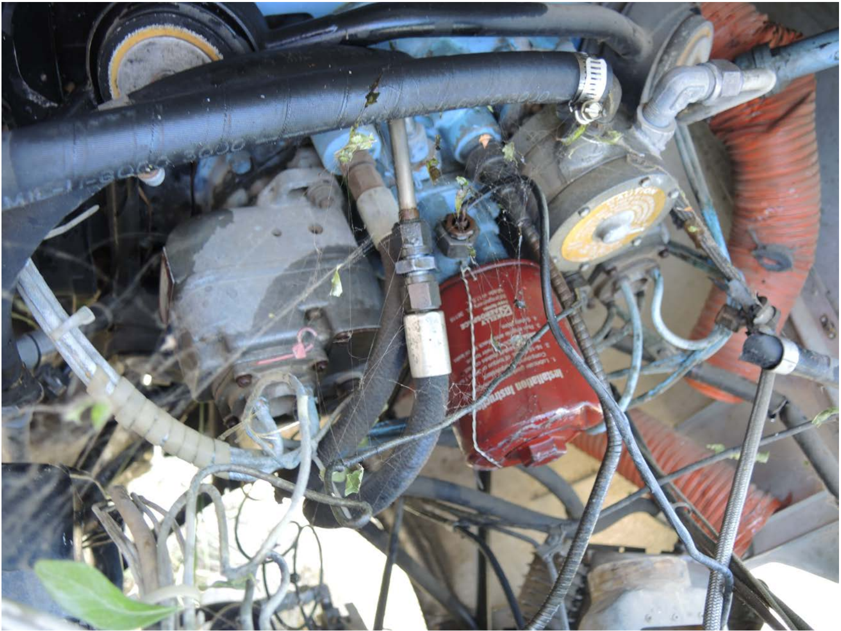
Photo 5 – Engine Compartment Cob Webs
