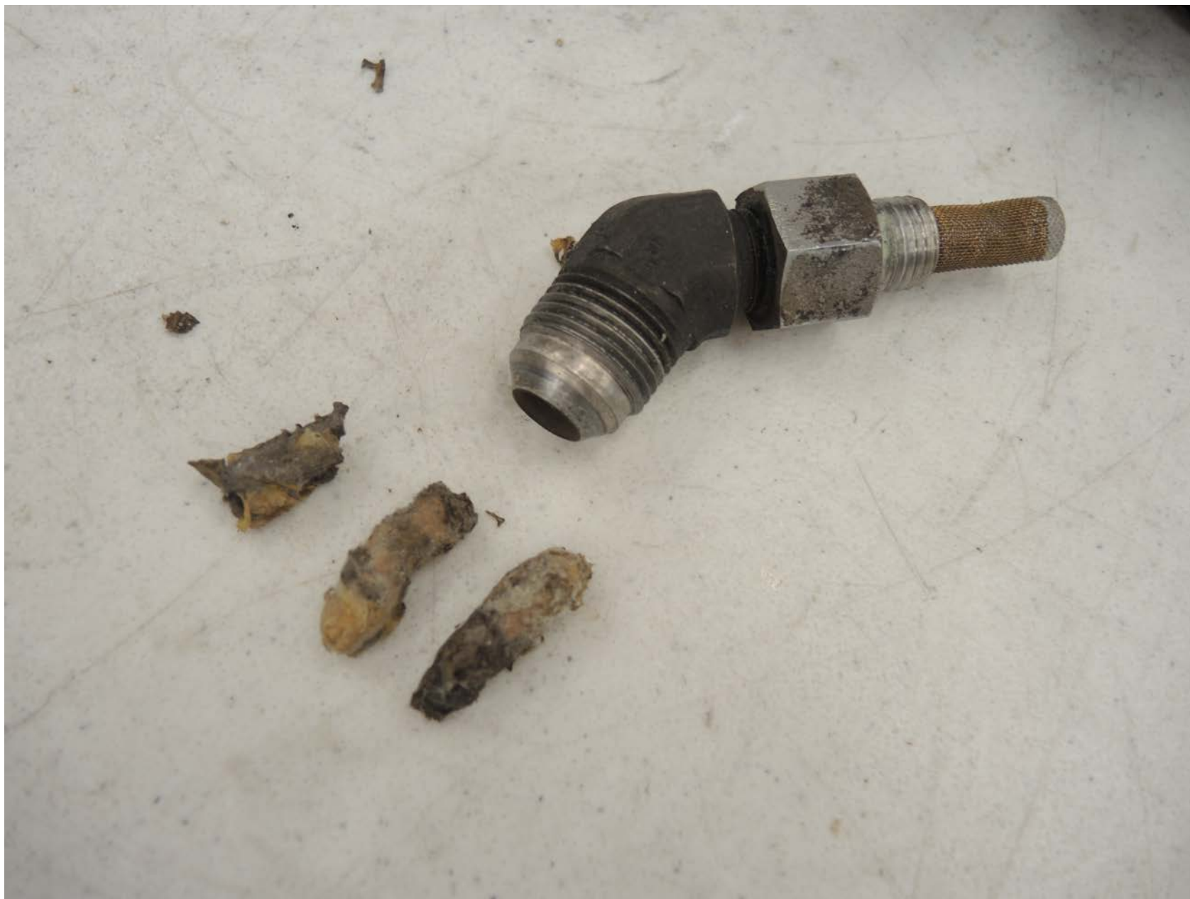
Photo 16 – Organic Debris In Fuel Line Fitting
