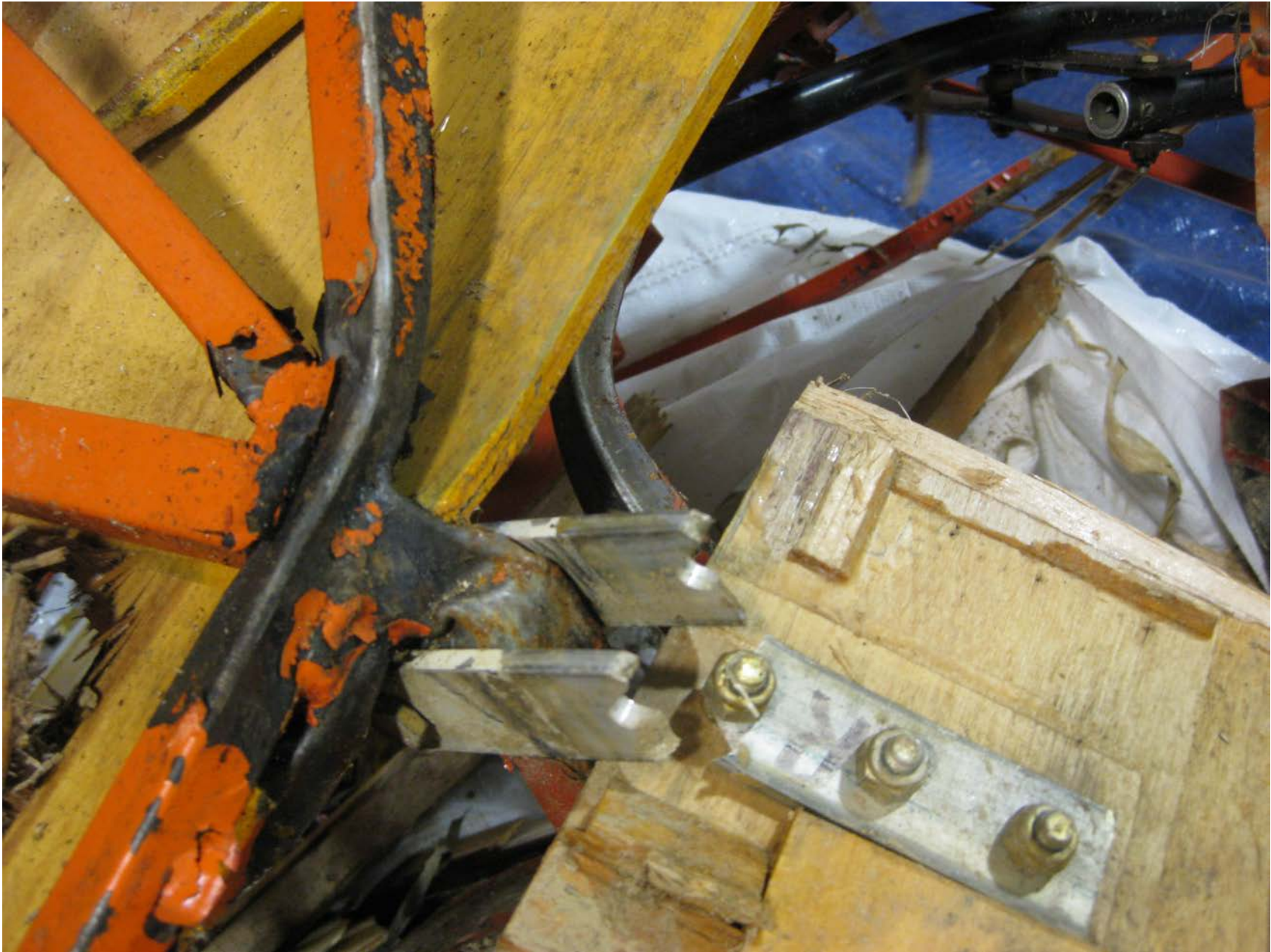
Photo 7 – Lower right wing main spar bracket and attachment fitting bore signatures consistent with overload.
