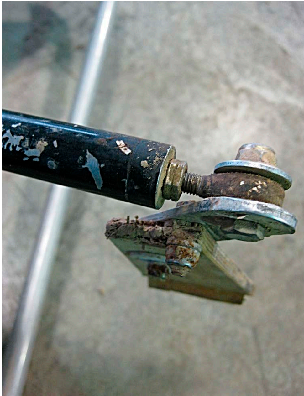
Photo 13 – Right aileron torque tube and attachment fitting where it attaches to the aileron.
