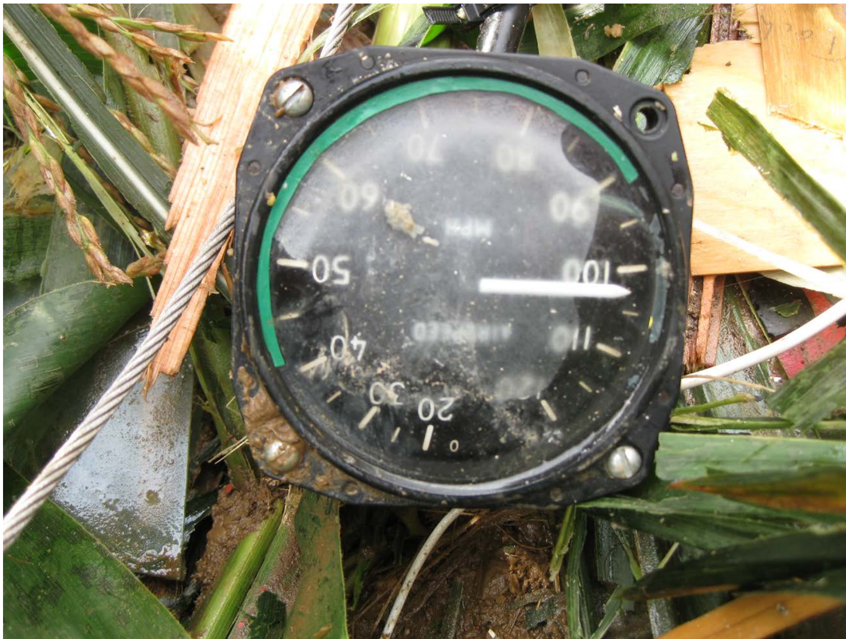
Photo 5 – The airspeed indicator, as found at the accident site, indicated 103 mph.
