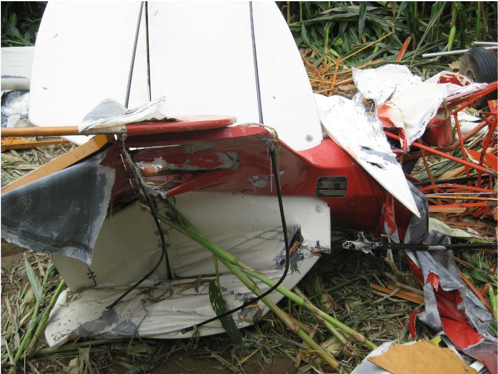
Photo 4 – The empennage. The right horizontal stabilizer was crushed. The left horizontal stabilizer was undamaged.
