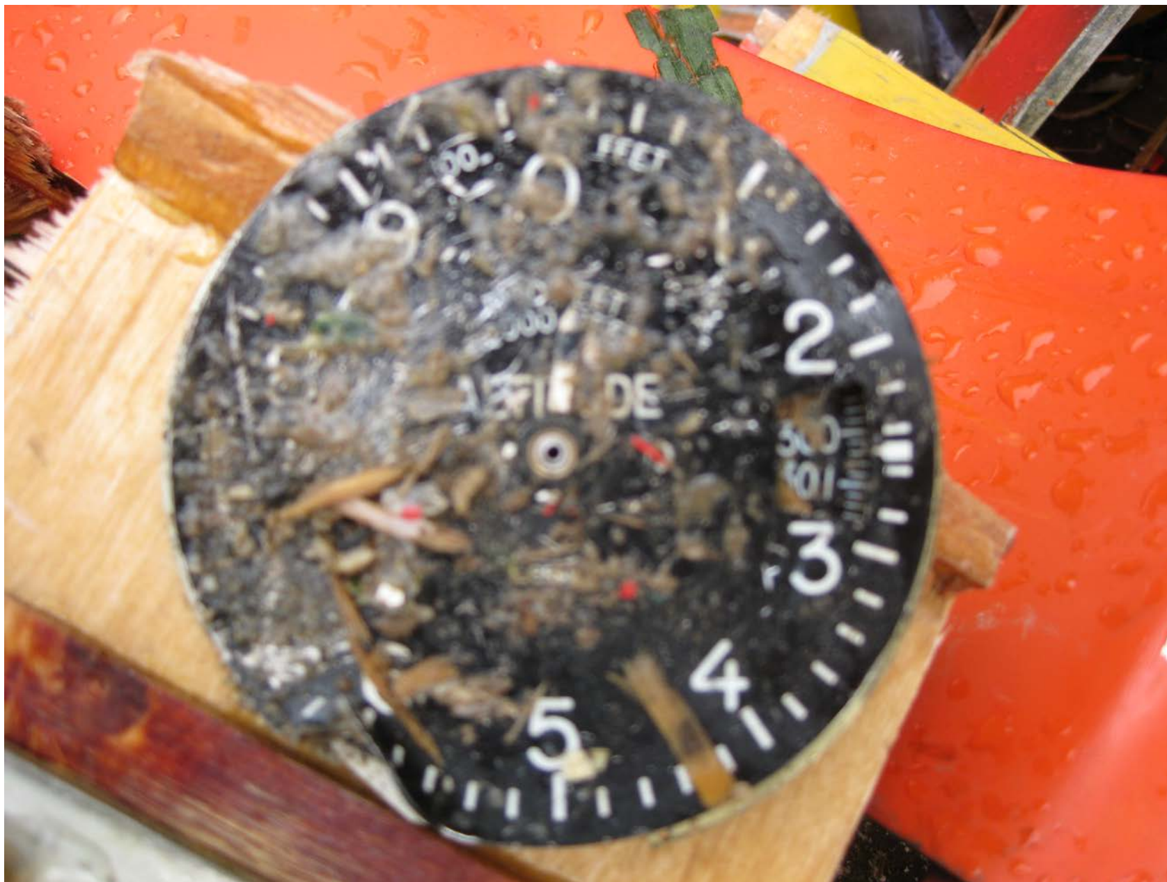
Photo 6 – The altimeter’s faceplate, as found at the accident site. The barometric pressure was set at 30.04 inches of mercury in the Kollsman window.
