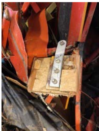
Image 4: Main Spar Severed Just Outboard of the Attach Bracket
