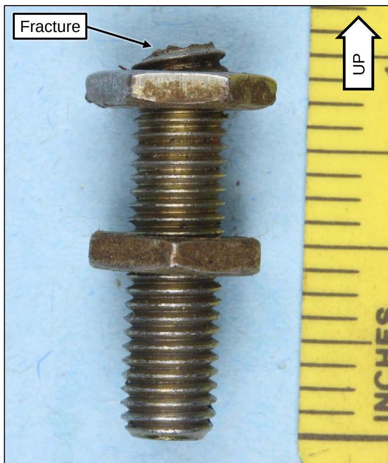
Figure 3. Right aileron control rod threaded shank with attached jam nuts.
