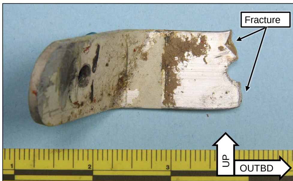
Figure 2. Inboard portion of the fractured aft spar attachment fitting.
