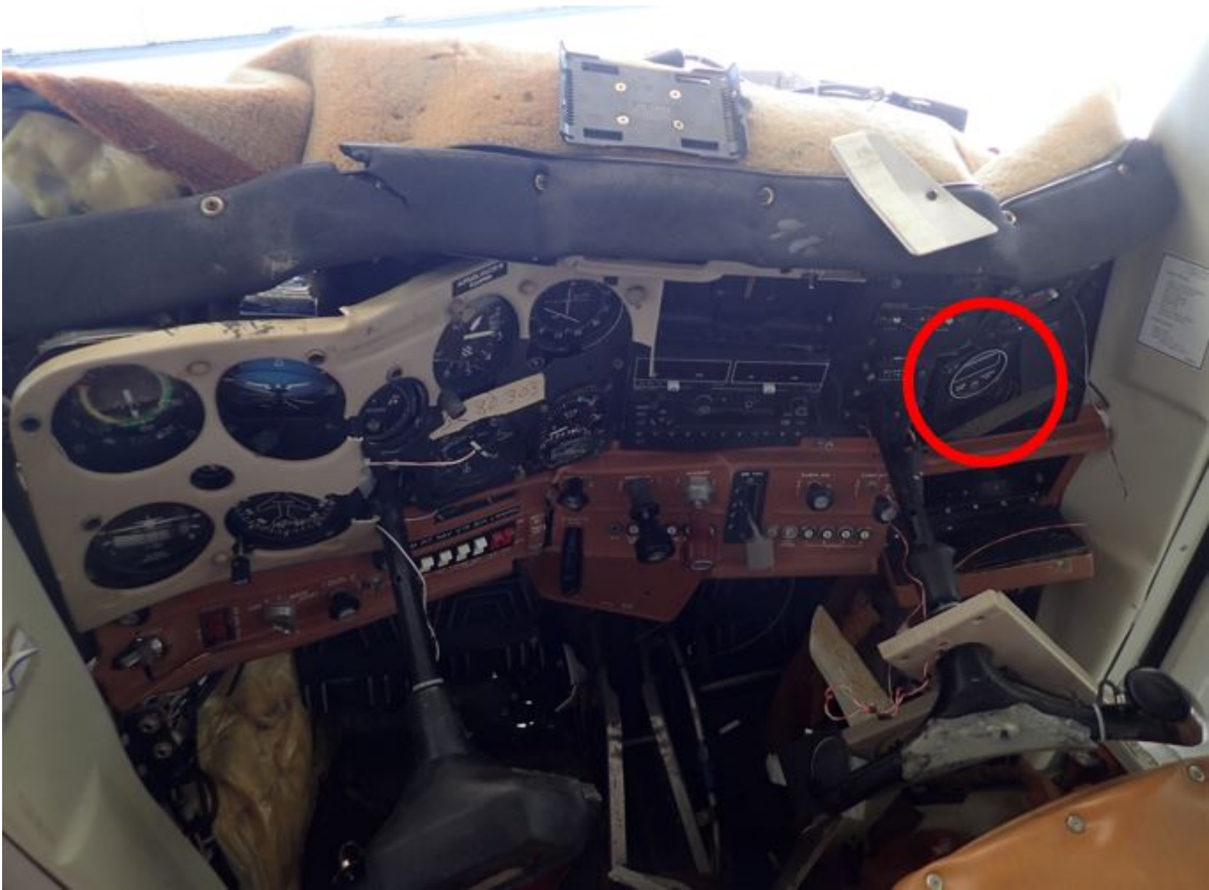
Photo 6 – Left seat view of the cockpit. The carburetor temperature system, installed on the right side of the cockpit, is highlighted with a red circle.
