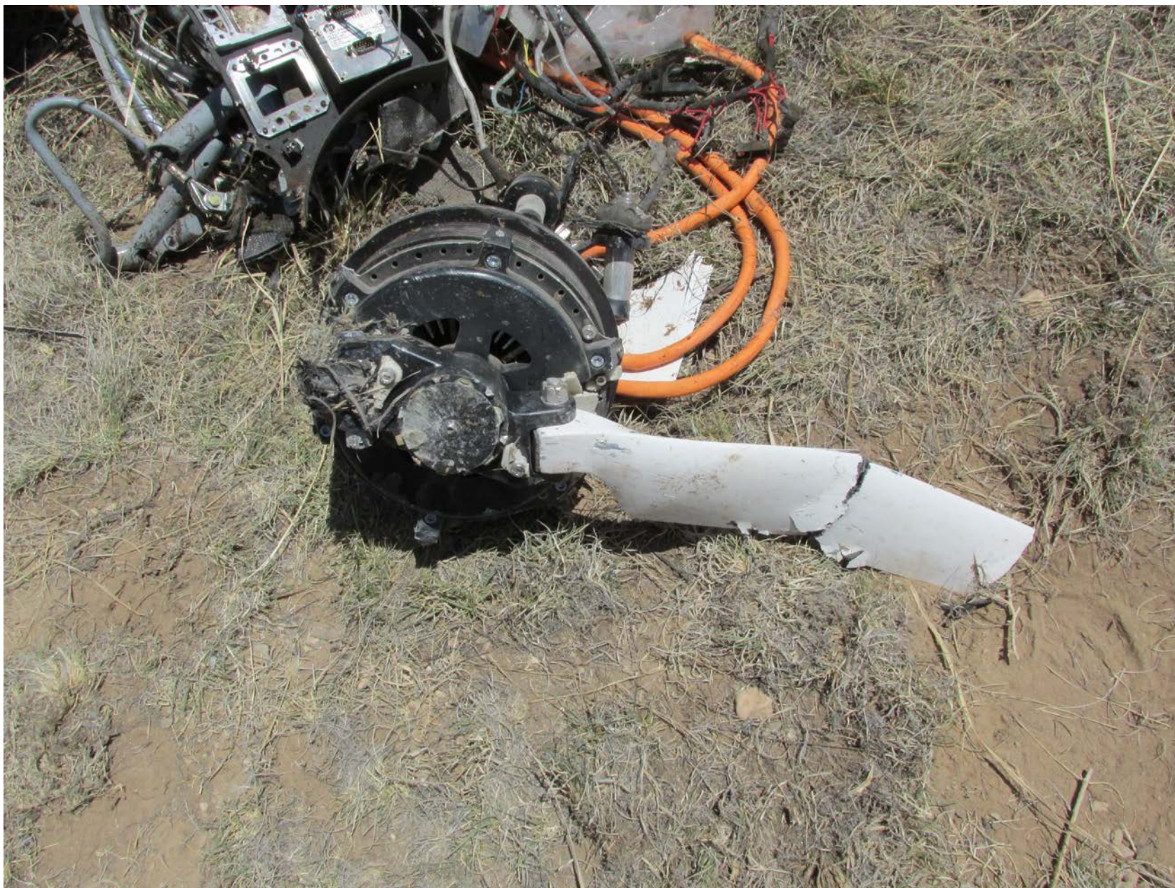
Photo 6 – Electric Motor and inboard 2/3rds of one of two Propeller Blades
