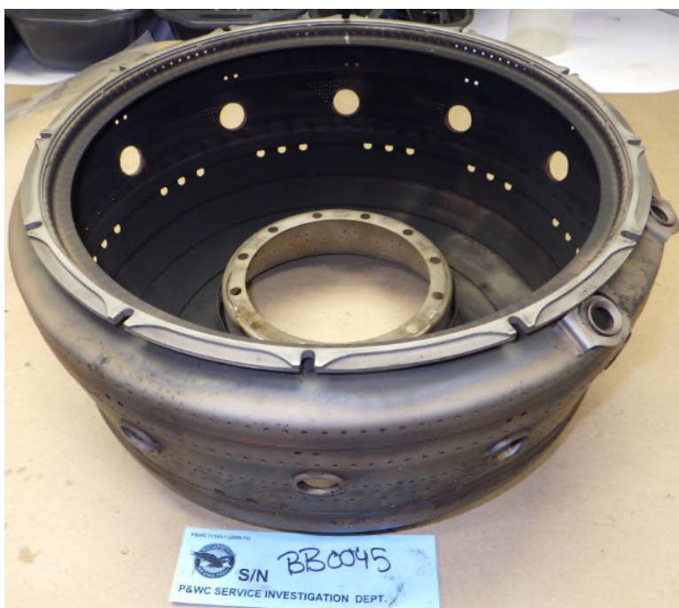
Photo No. 64: Outer liner
