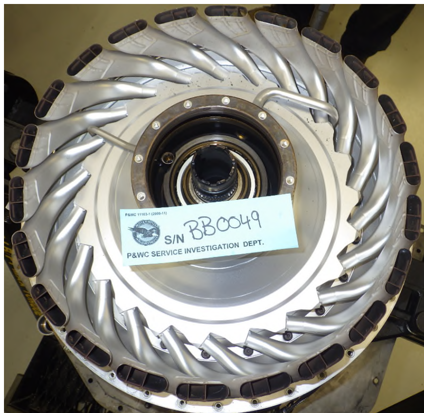
Photo No. 12: Diffuser pipes
