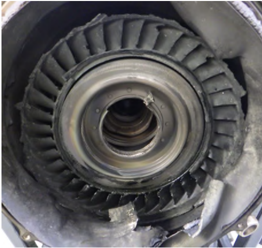
Photo No. 77: PT stator trailing edges
