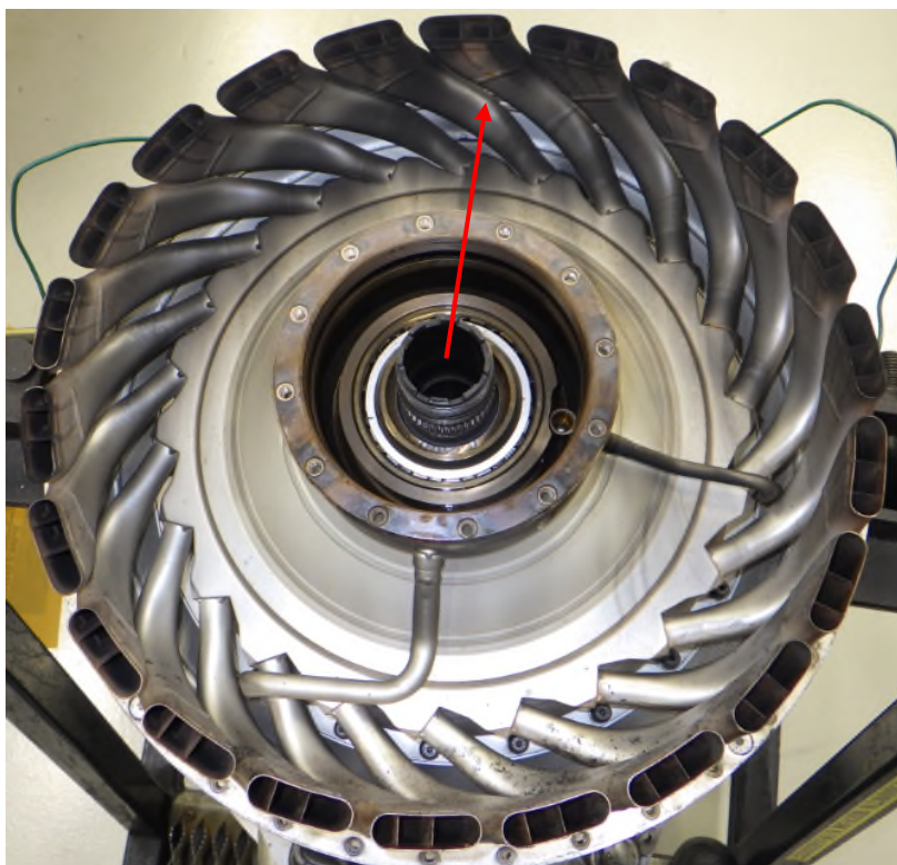
Photo No. 61: Soot build up on the diffuser tubes at the 12 O'clock position
