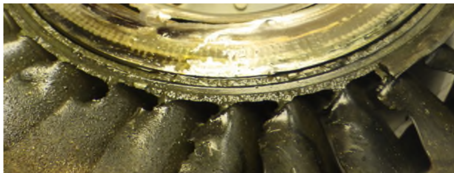
Photo No. 76: Grooved TE of PT stator vanes
