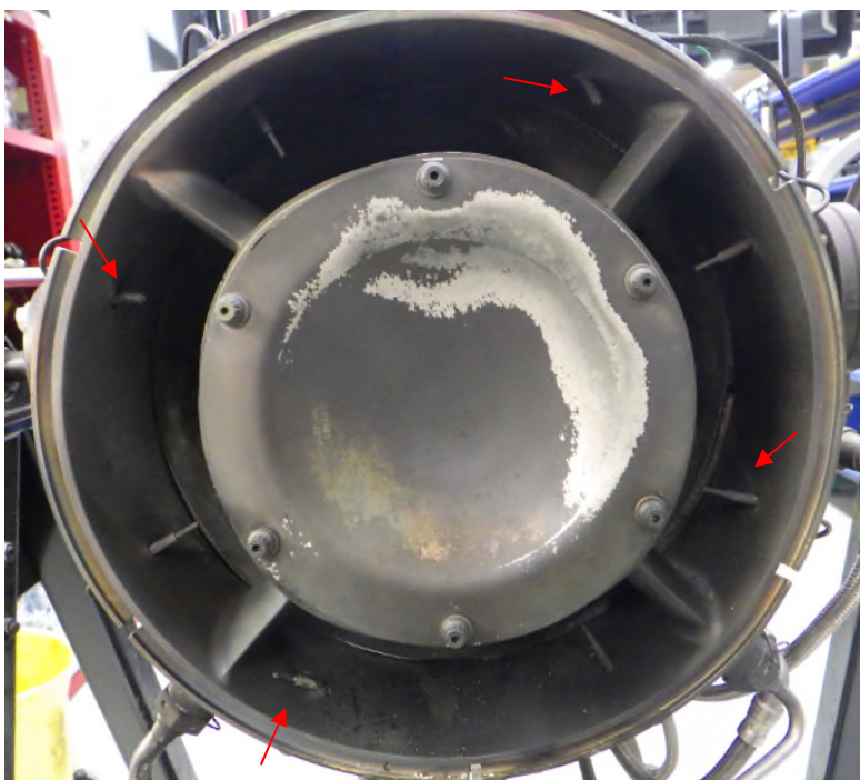
Photo No. 74: Exhaust with damaged T6 probes.
