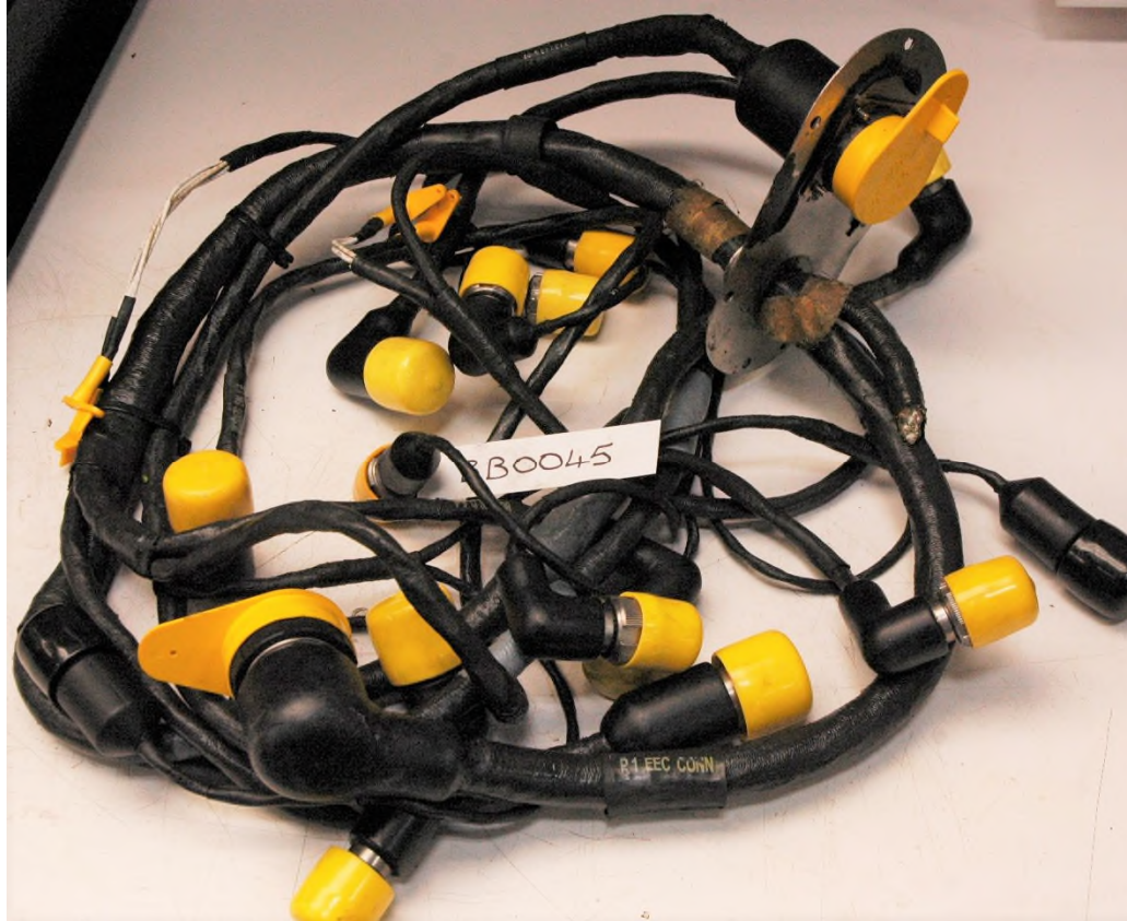
Figure 13 No. 2 engine wiring harnesses as received
