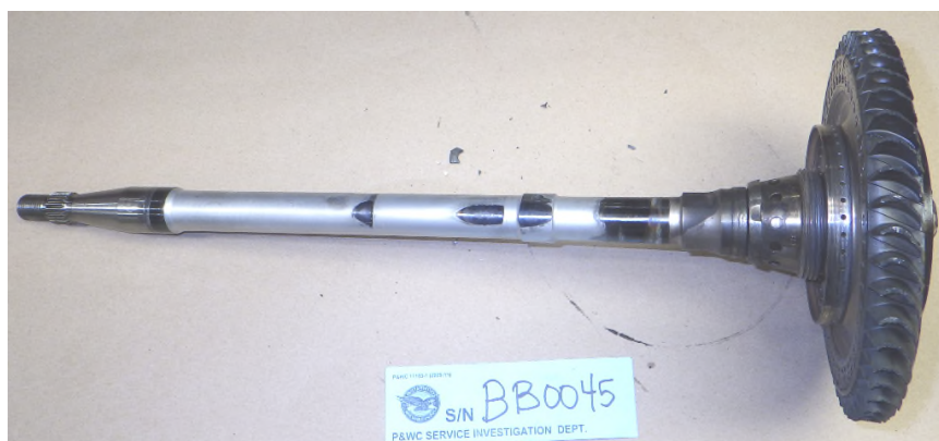
Photo No. 85: Power Turbine Shaft
