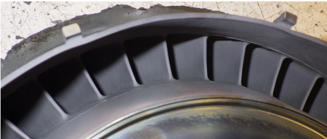
Photo No. 27: Leading edge of PT stator vanes
