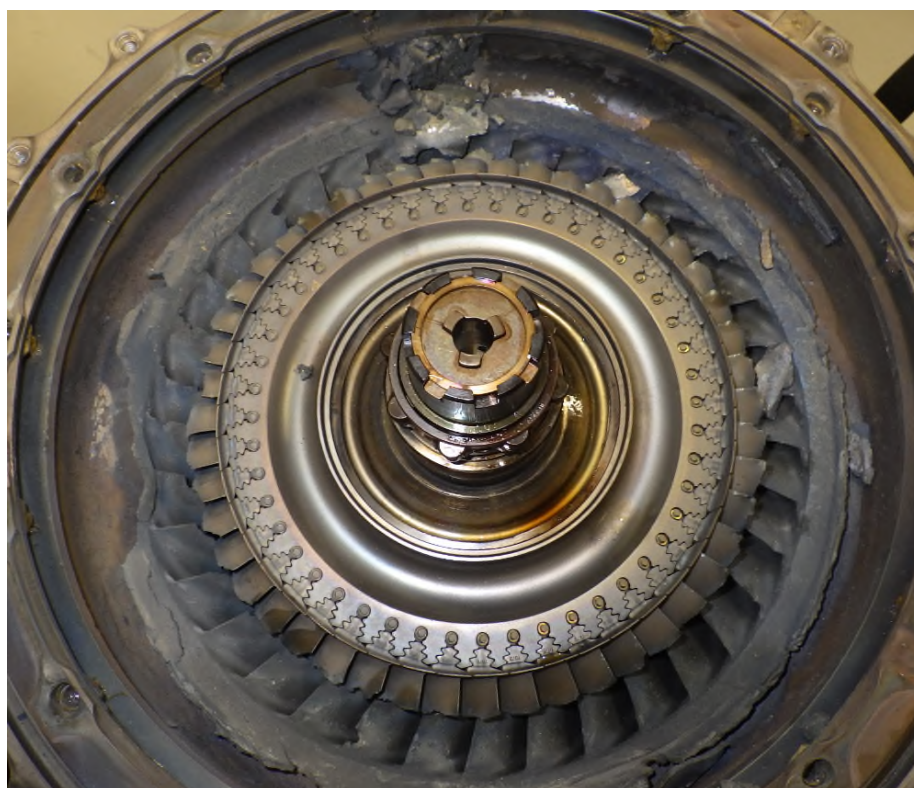
Photo No. 30: PT blades all missing at 1/3 span
