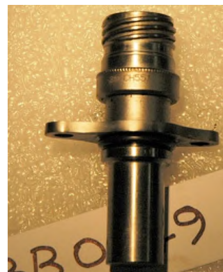
Photo No. 45: NPT sensor
