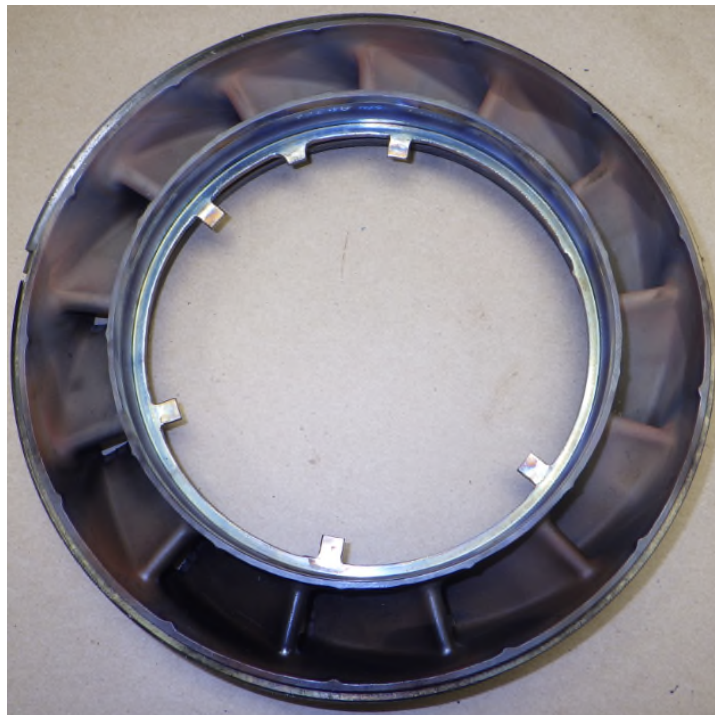
Photo No. 68: CT stator leading edges
