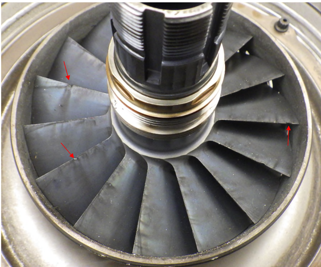
Photo No. 8: Centrifugal impeller leading edge
