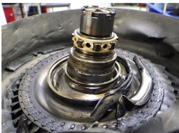
Photo No. 83: PT shaft off-center
