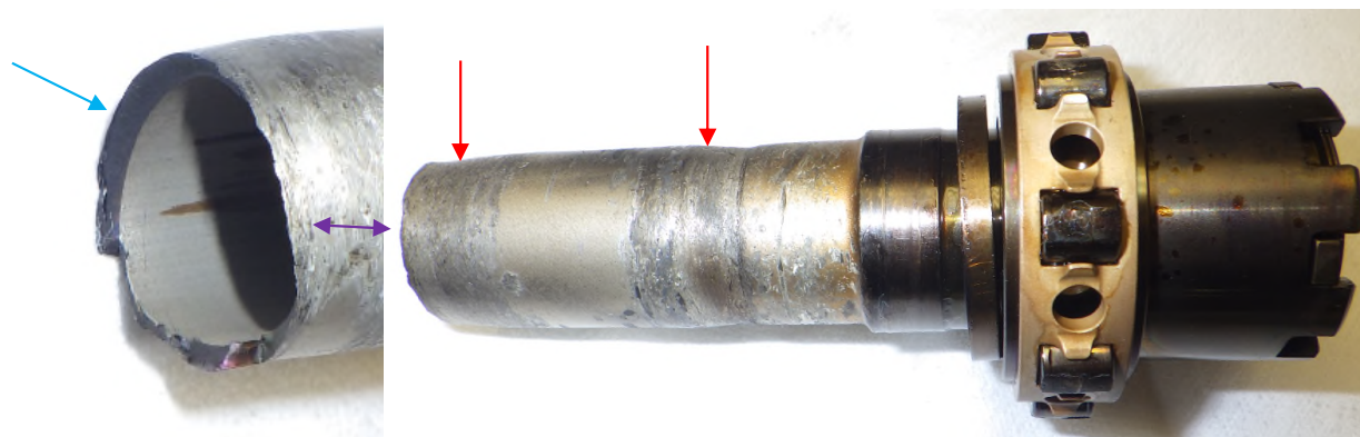
Photo No. 84: Sheared section of PT shaft
