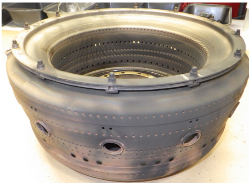
Photo No. 63: Combustion chamber
