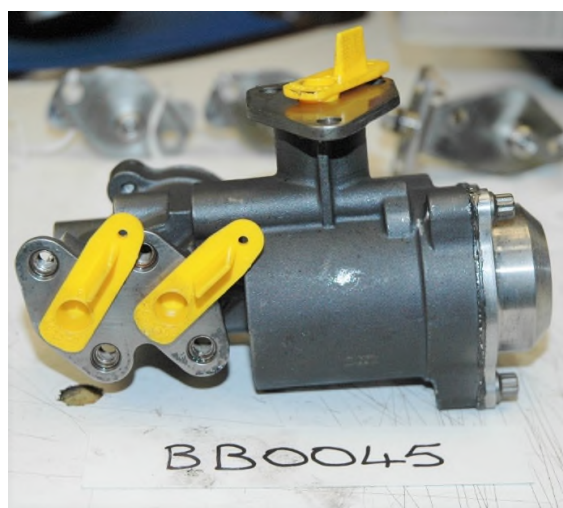
Photo No. 98: Flow divider valve
