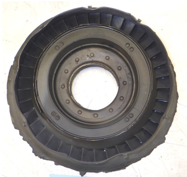
Photo No. 79: PT stator leading edges
