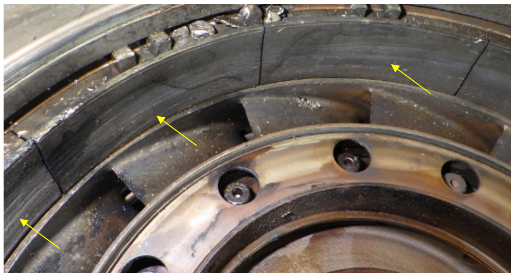
Photo No. 71: CT shroud with rubbing marks
