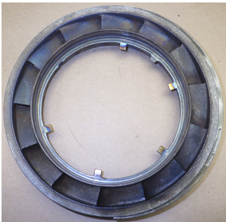
Photo No. 69: CT stator trailing edge
