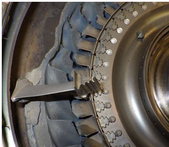
Photo No. 31: Broken PT blades and a new PT blade
