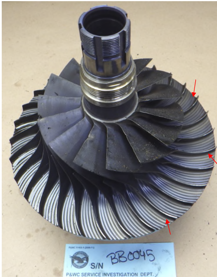
Photo No. 58: Impeller with rub marks
