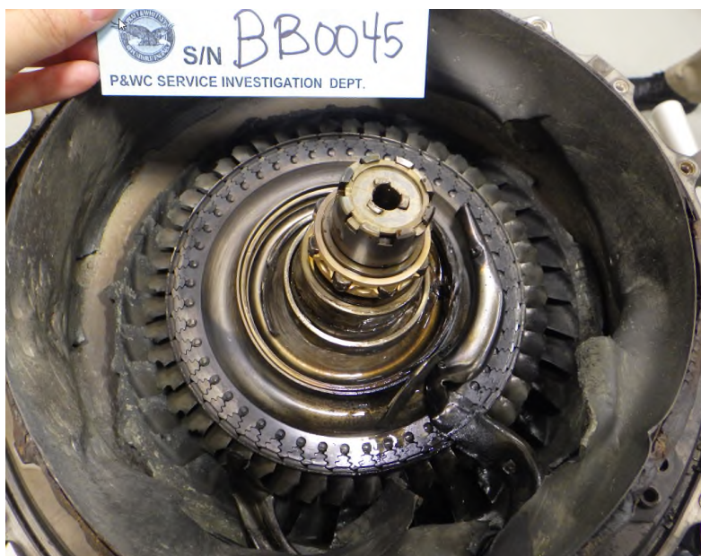
Photo No. 75: PT exhaust cone deformation
