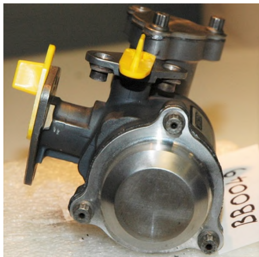
Photo No. 42: Flow Divider Valve
