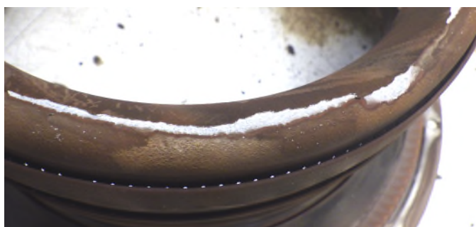
Photo No. 15: Coating loss on the inner liner exit lip
