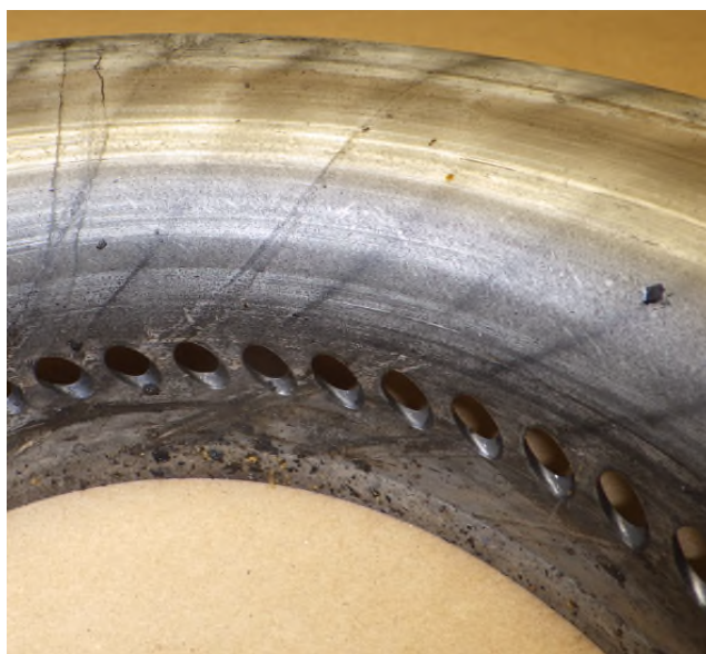
Photo No. 60: Close up of scoring
