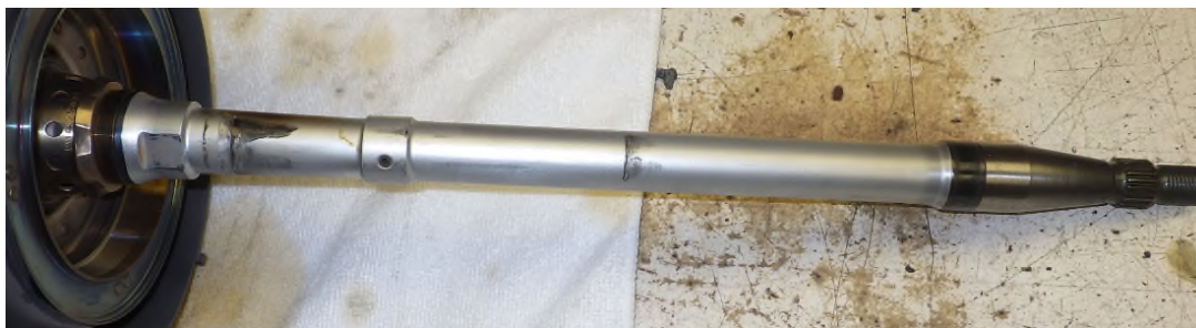
Photo No. 32: PT shaft
