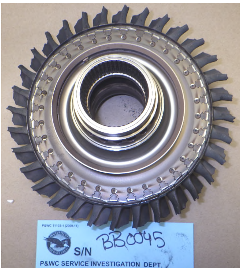
Photo No. 73: CT blades leading edges
