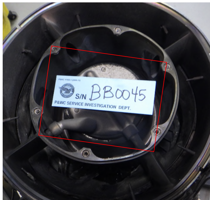
Photo No. 52: BB0045 No. 5 bearing support
