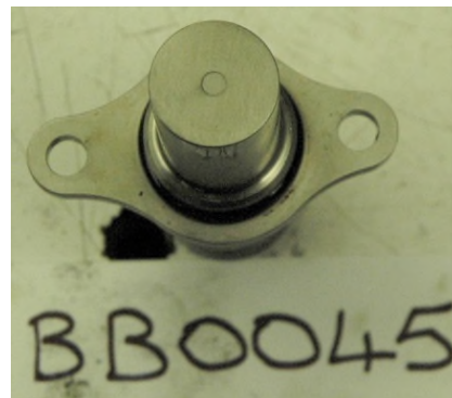
Photo No. 101: NPT sensor
