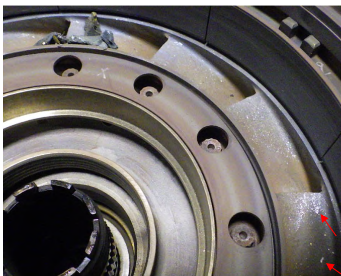
Photo No. 20: Metal spray on backside of CT stator
