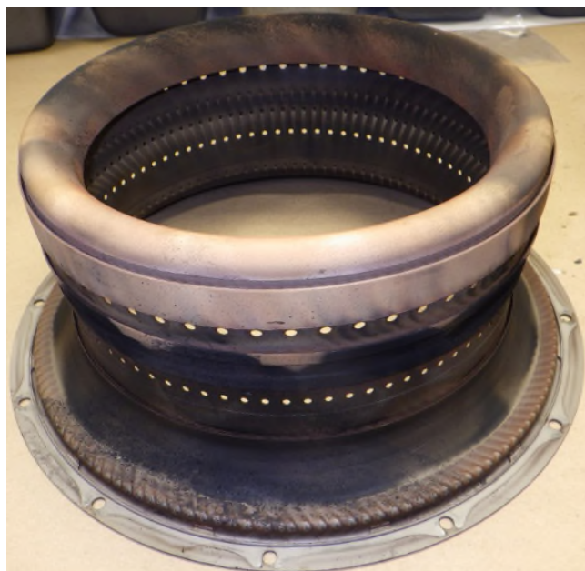
Photo No. 66: Inner liner soot build up
