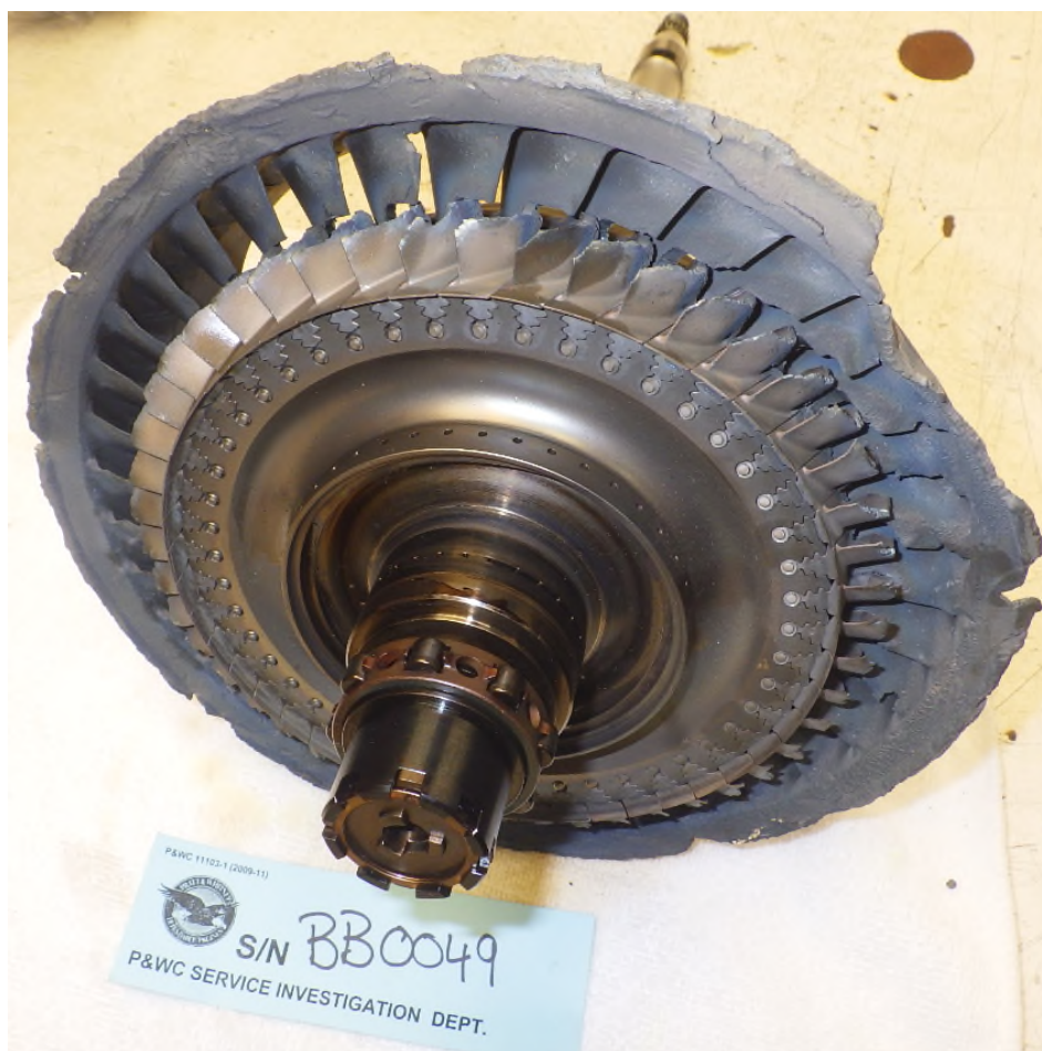
Photo No. 25: PT stator vane ring and PT disc assembly removed together
