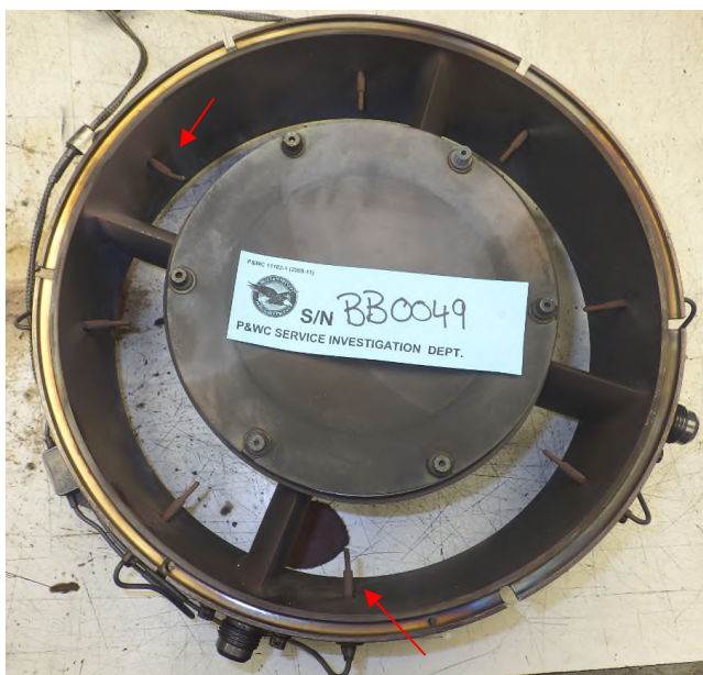
Photo No. 24: Damaged T6 probes
