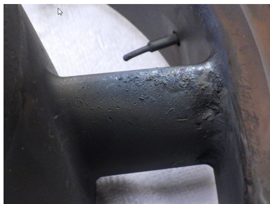
Photo No. 35: Impact damage to exhaust strut
