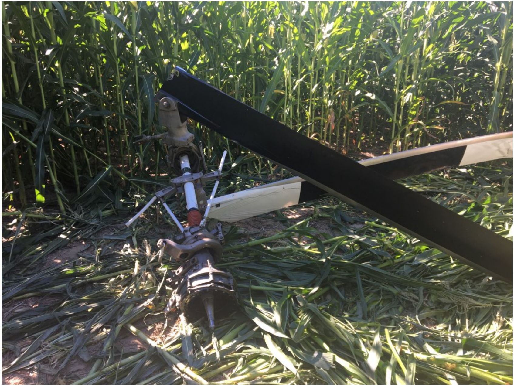
Photograph 9 - Main Rotor and Upper Transmission
