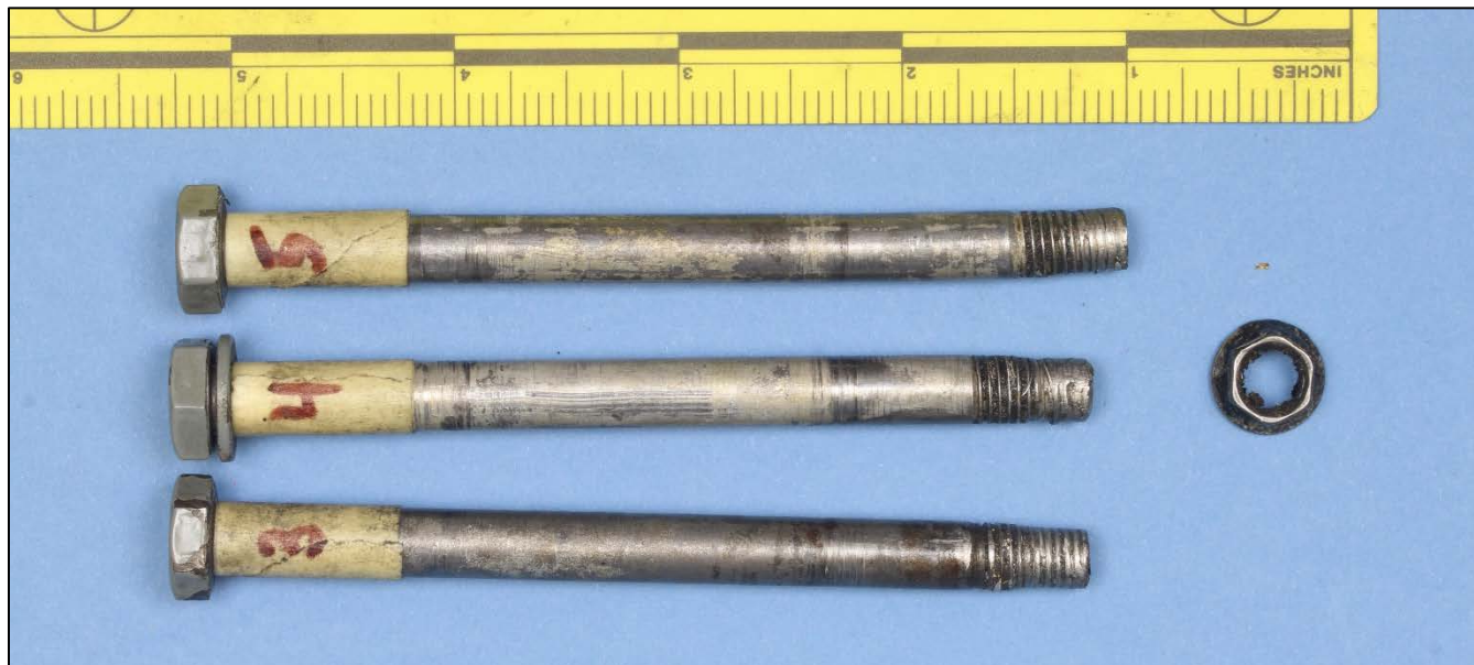
Figure 2. Overall view of main rotor housing assembly attachment bolts, washer (on bolt 4), and nut received separately.
