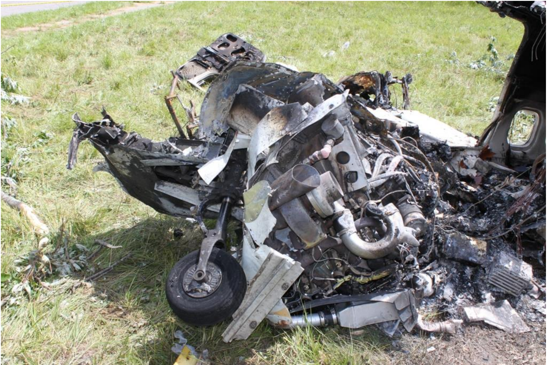
Photo 5 – Engine Compartment and Nose Landing Gear
