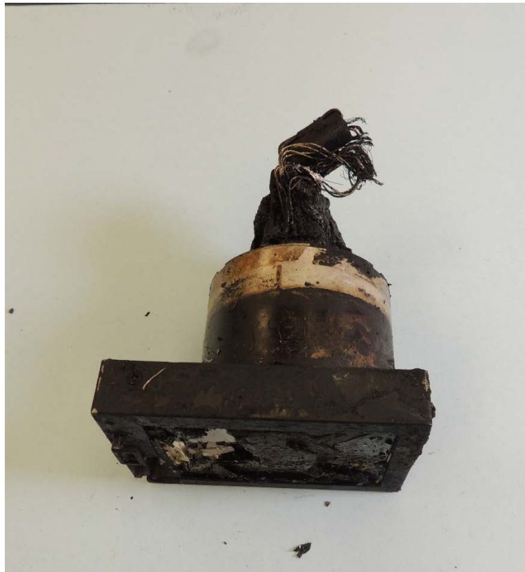
Figure 1. Heat and fire damage to the EDM-730.
