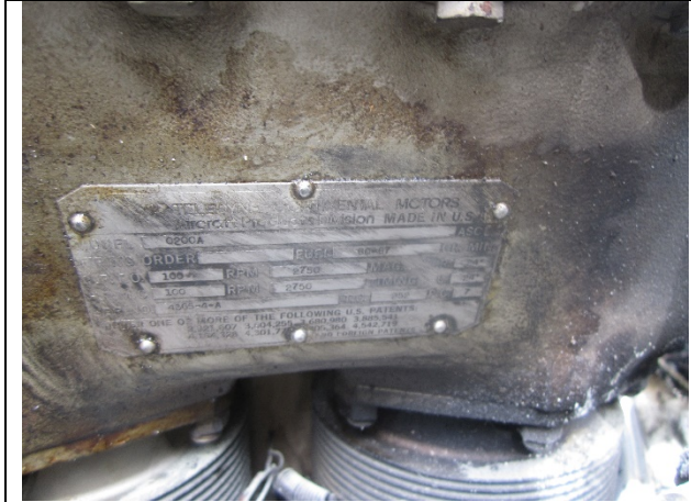
Engine identification plate: Continental O-200A
