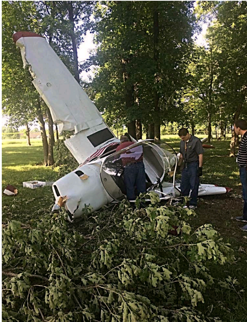
Photo 1 – The wreckage of N622DP rests on its left side after striking trees and impacting the ground between the 16th and 18th holes at the Silo Ridge Golf and Country Club, Bolivar, Missouri.
