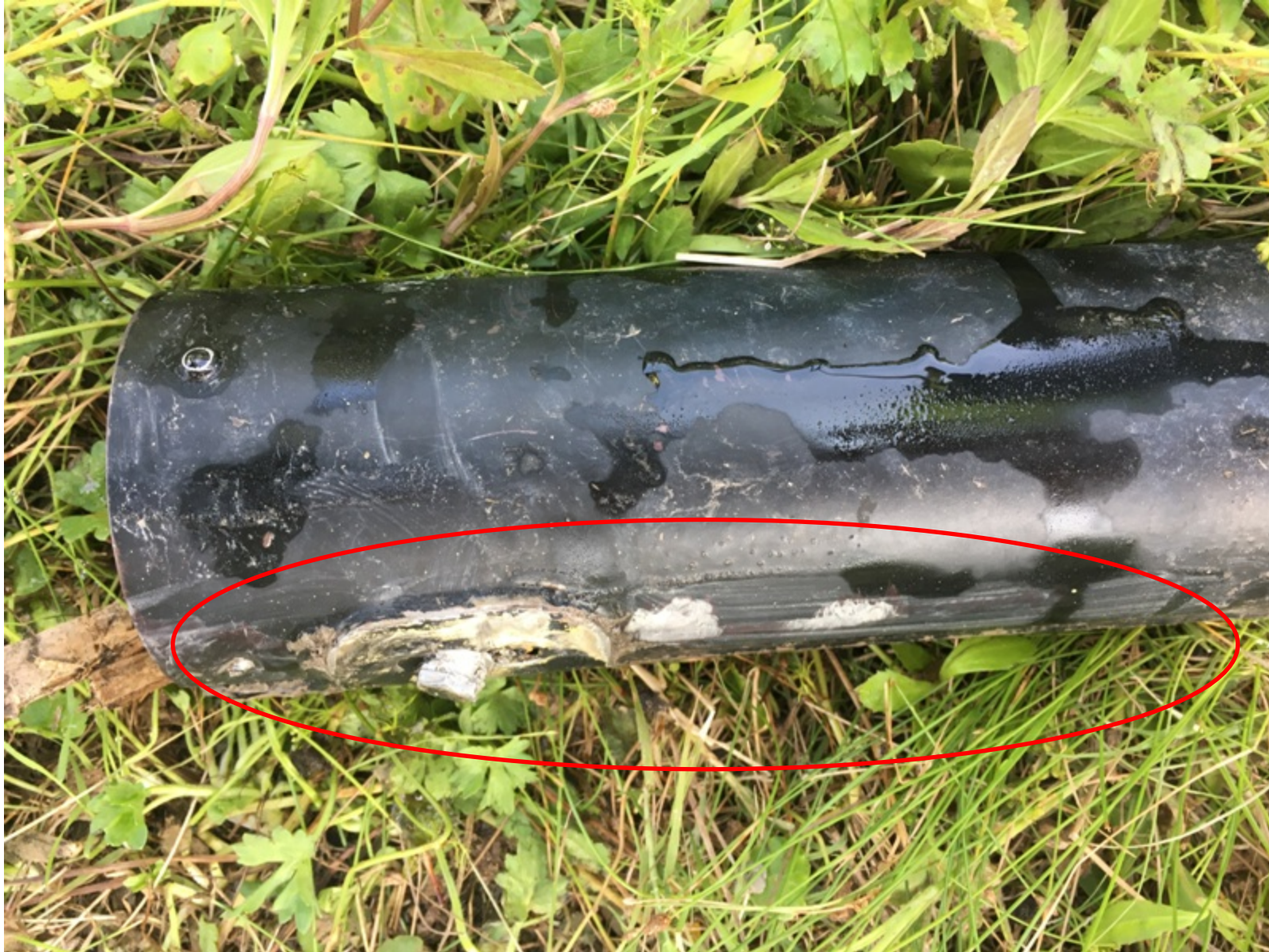
View of aft left side showing damage to the skid shoe bolt and paint scrapes.
