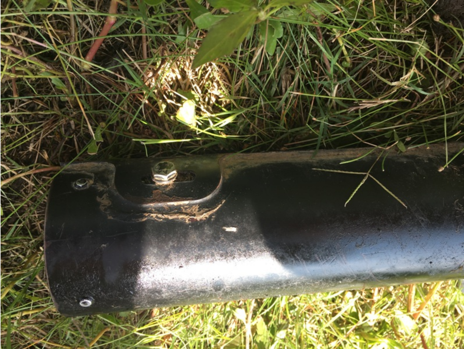
View of right aft skid showing no damage.
