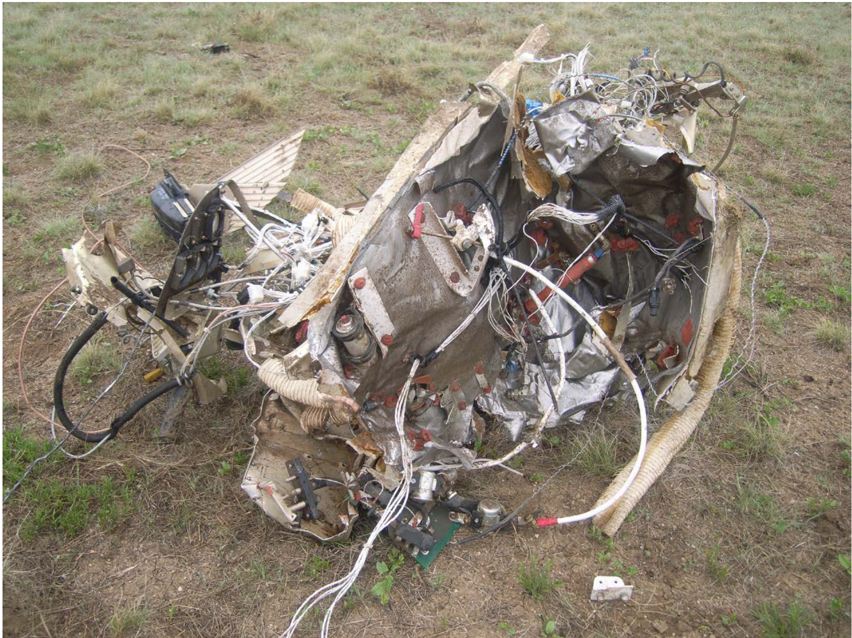
Photograph 7 – Firewall and Instrument Panel
