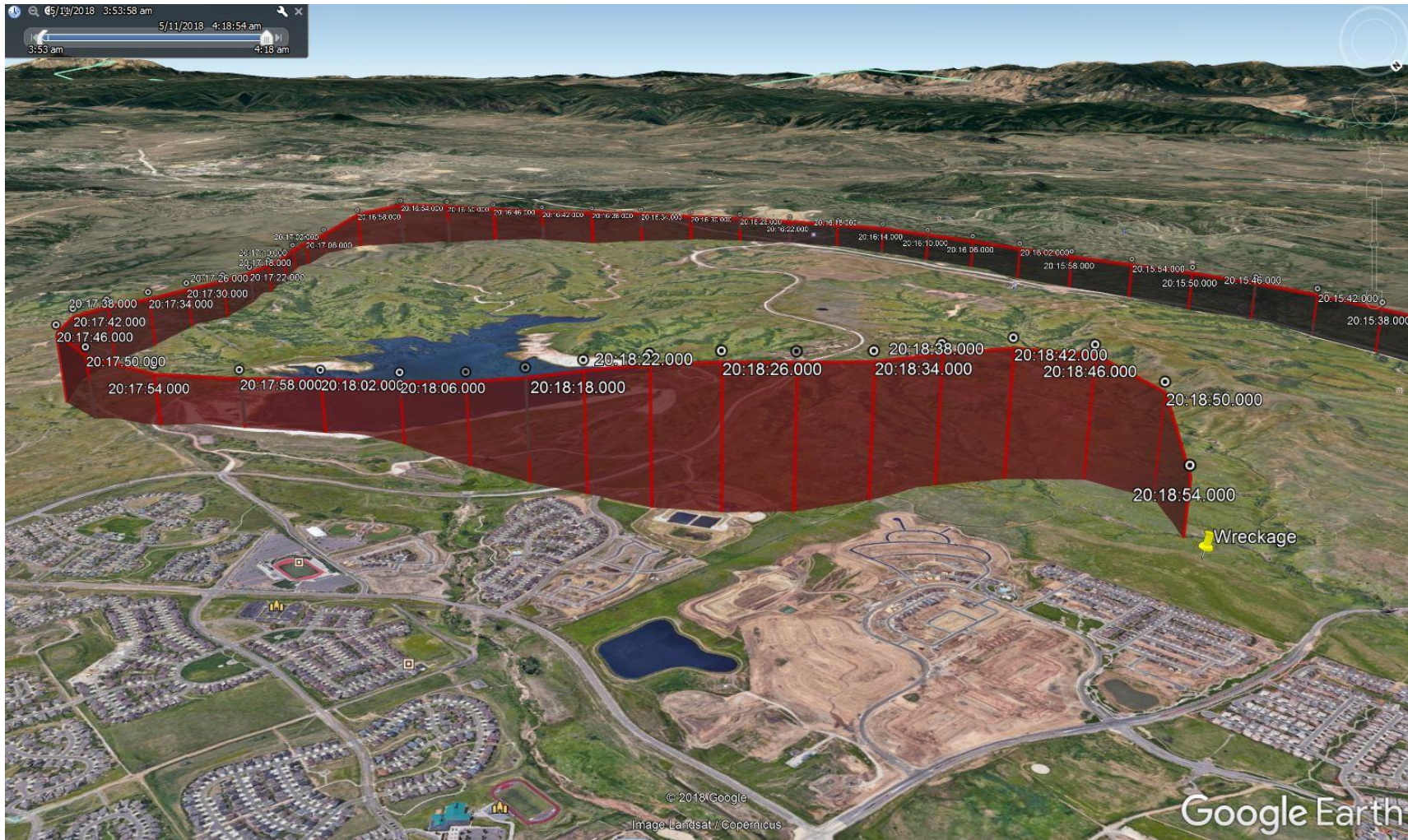
Figure 6. An overlay of recorded GPS data for the final portion of flight. The wreckage location is depicted as a yellow pin. The view is oriented looking southwest.
