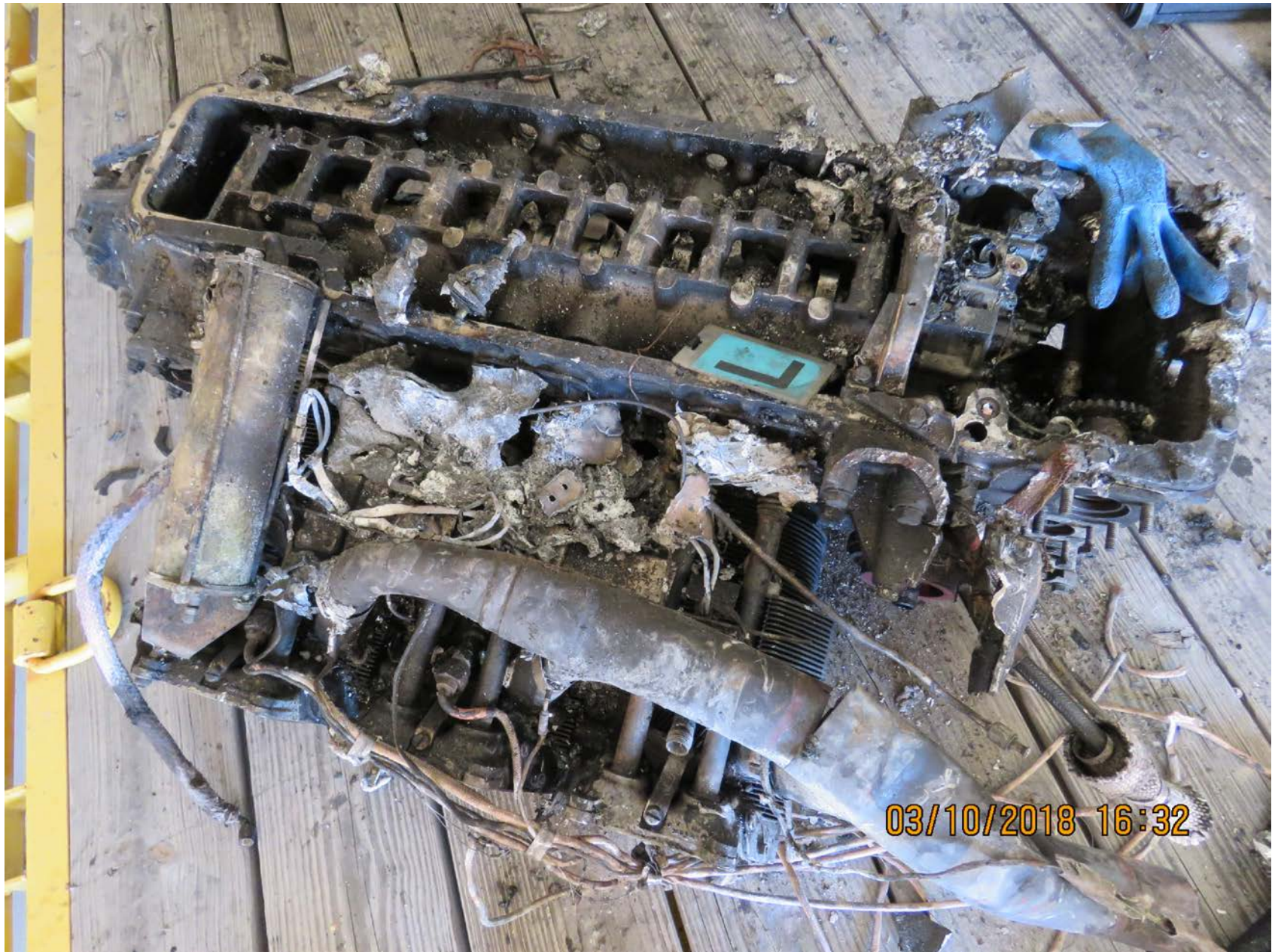
Photo 4 – Left side engine: Fire and impact damage
