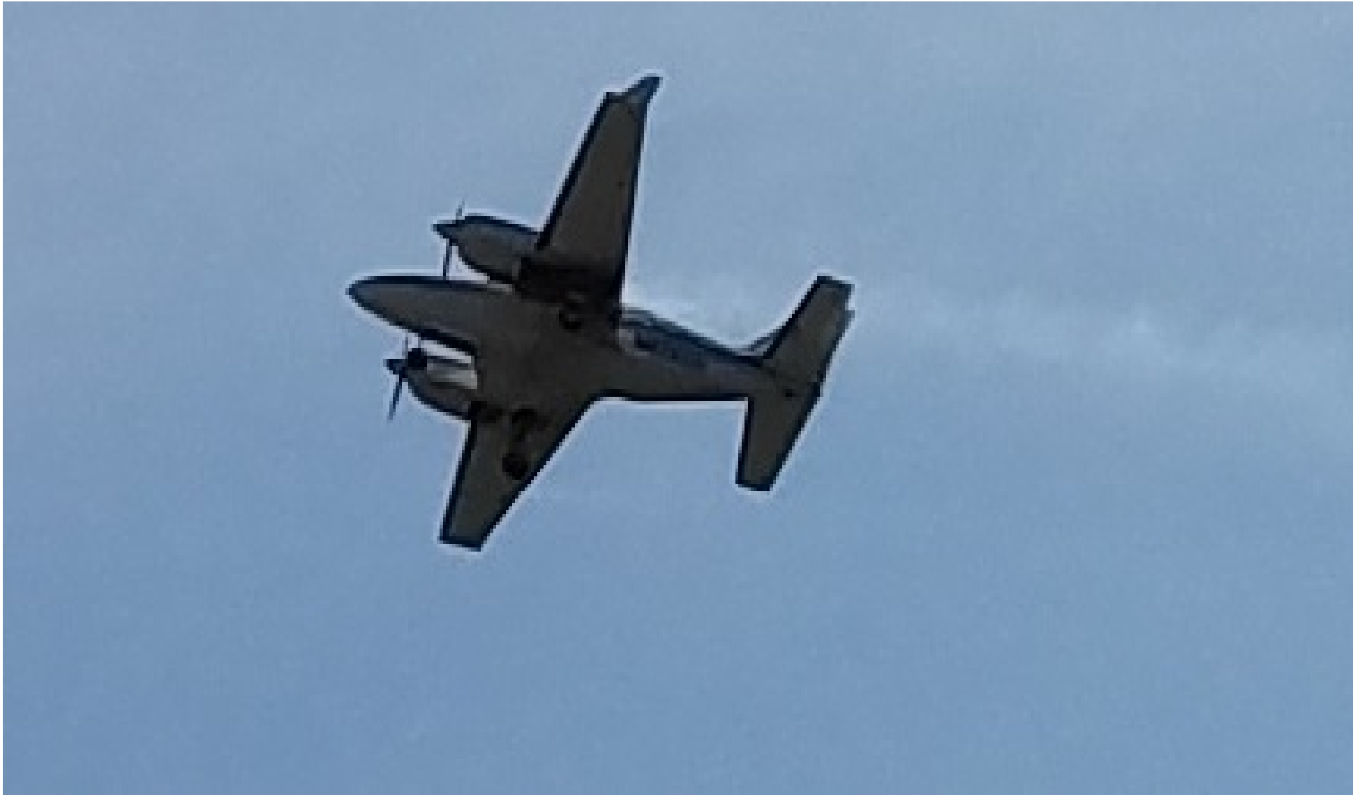
Photo 7 – Close-up view of the airplane; area under the left engine is dark. The landing gear is down. Witness photo, courtesy of FAA
