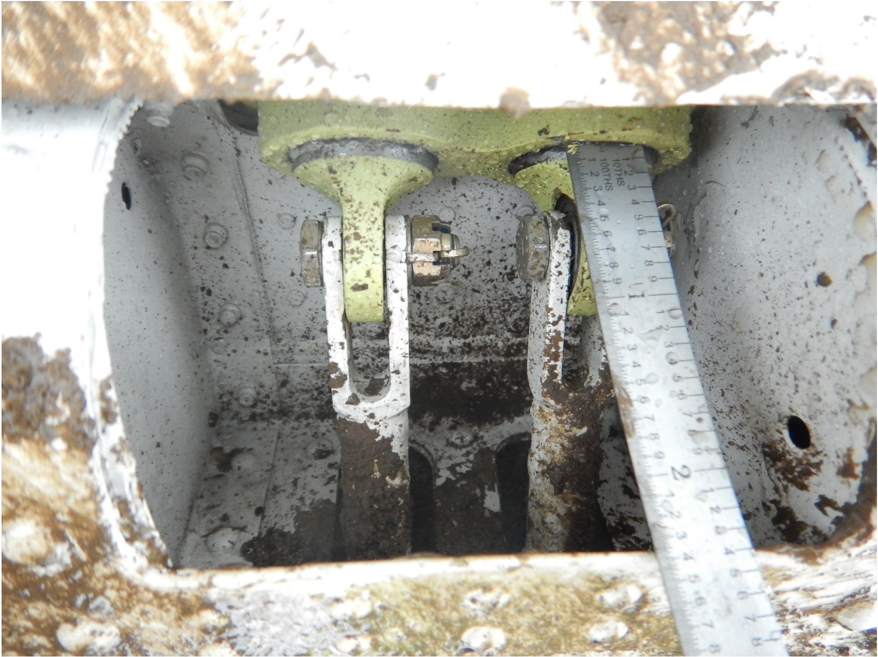
Photo 10 – Right Elevator Trim Actuator
