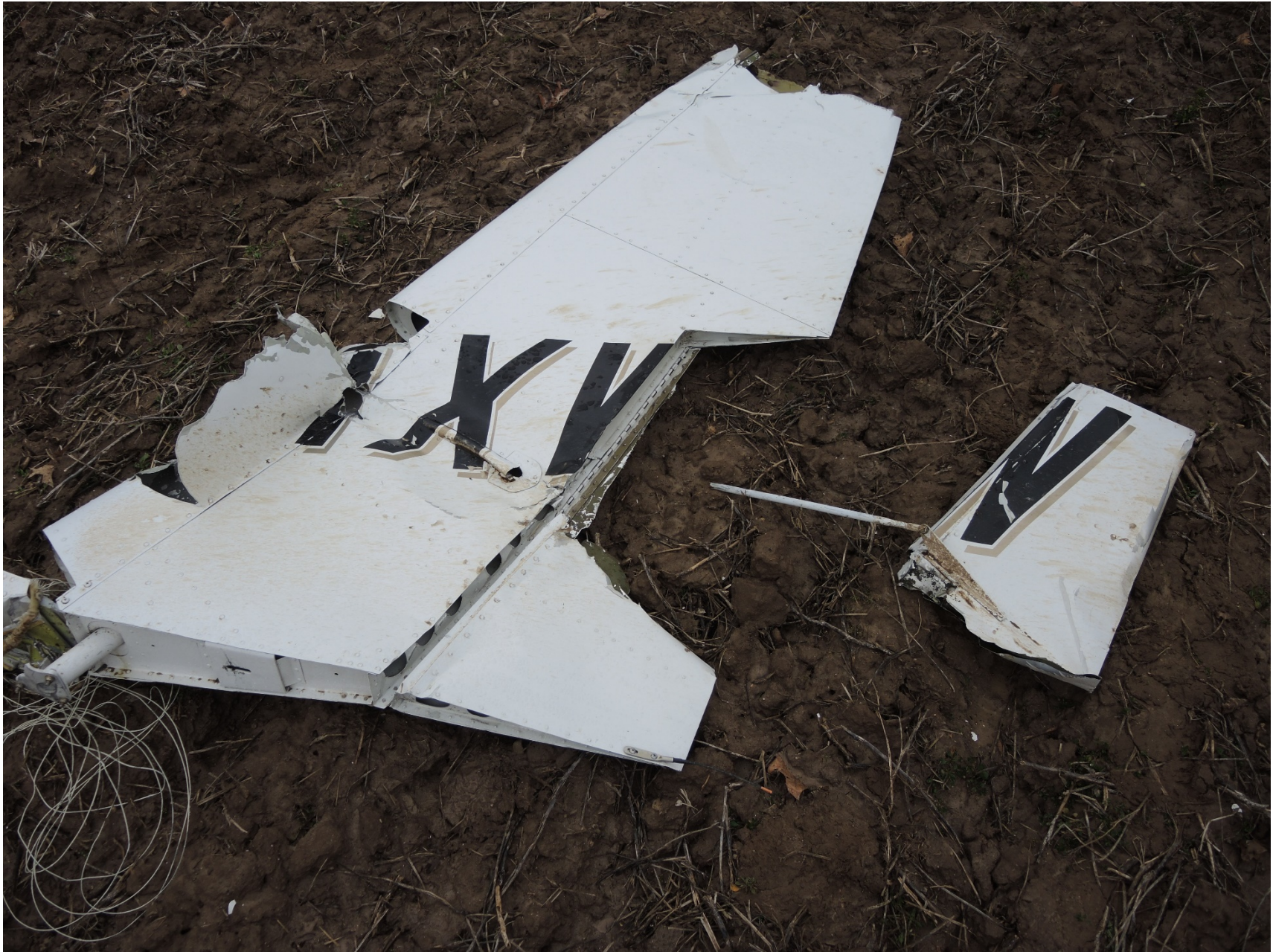
Photo 11 – Rudder and Rudder Trim Tab
