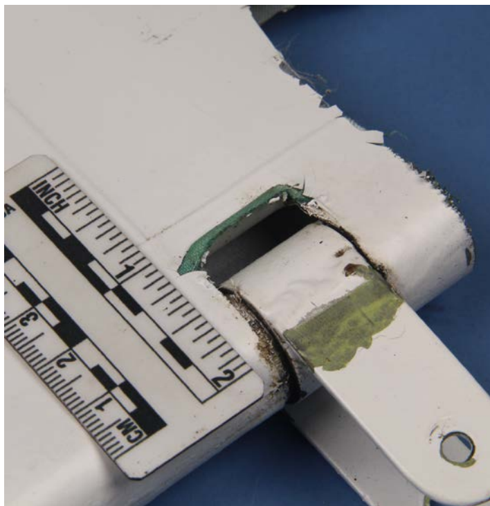
Figure 5: Top and bottom views of the right elevator inboard hinge.
