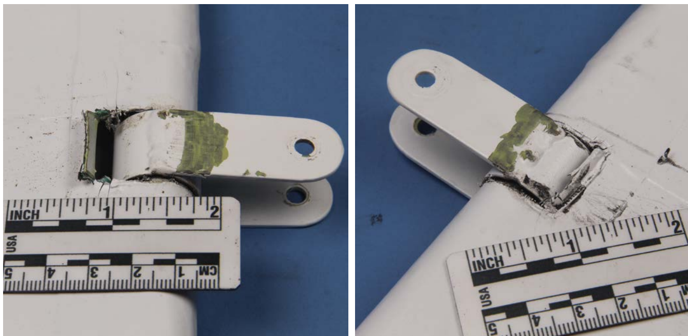
Figure 4: Top and bottom views of the right elevator outboard hinge.
