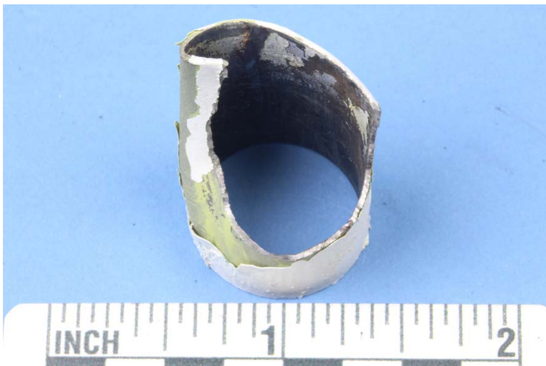
Figure 3: Portion of right elevator's tubular frame with fracture surface.
