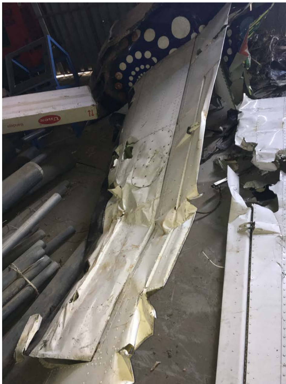
Photo 9 – Right Horizontal Stabilizer and Elevator
