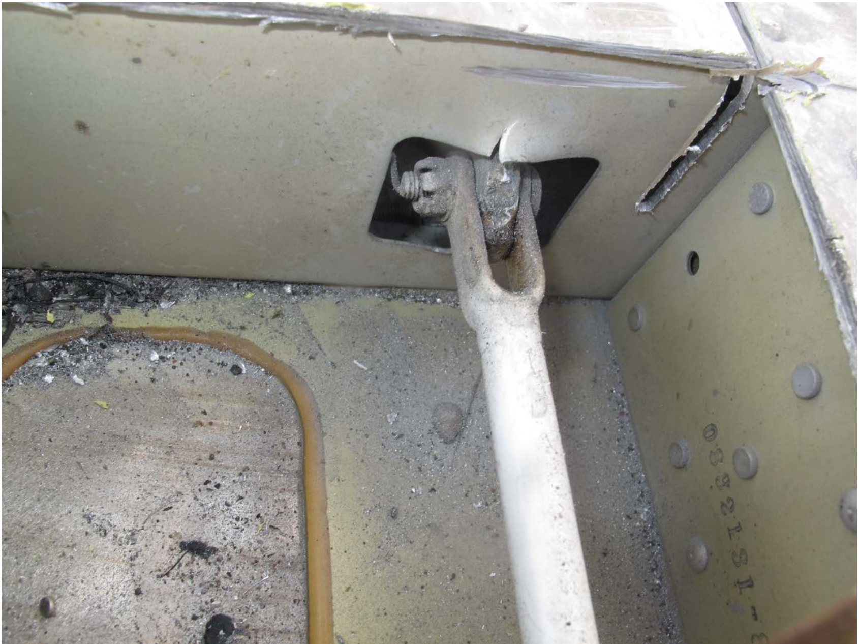
Photo 13 – Elevator Trim Control Rod
