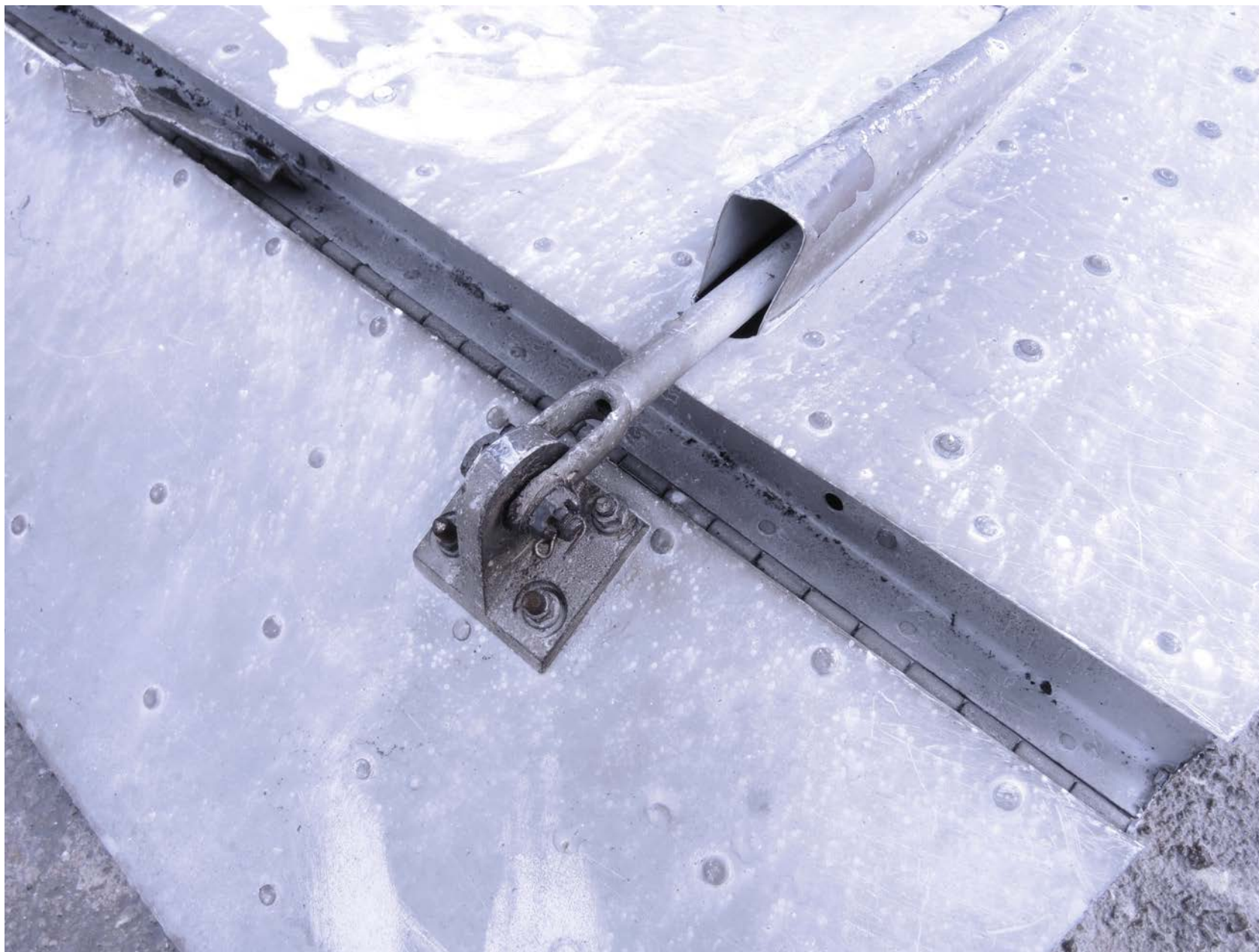
Photo 11 – Elevator Trim Control Rod
