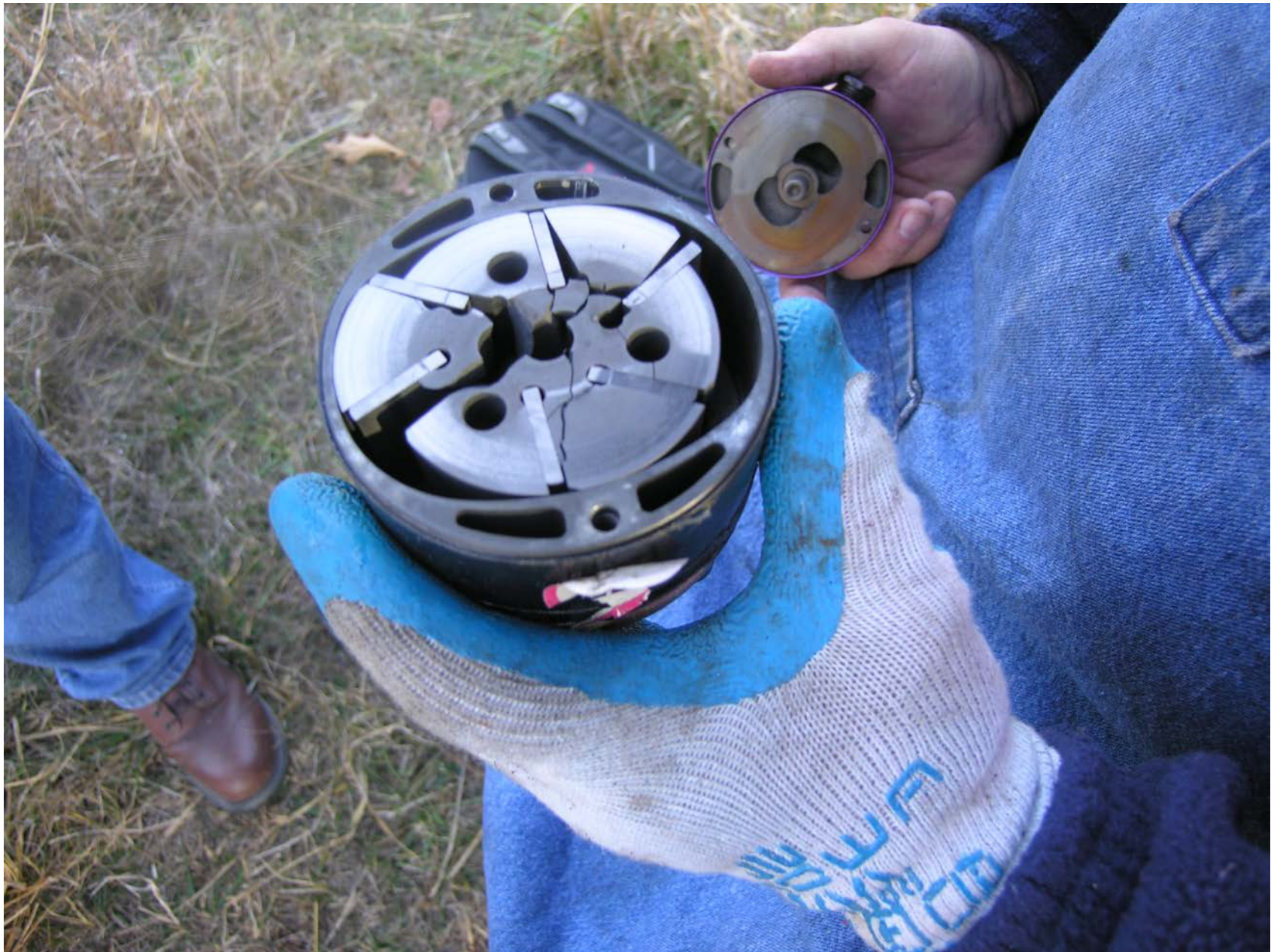
Photo 6 – Broken vacuum pump
