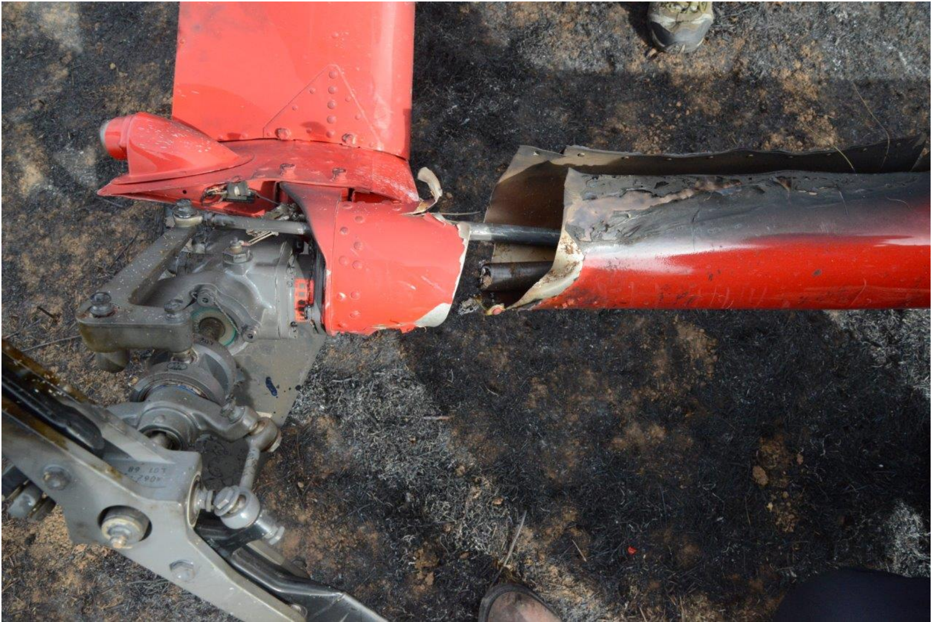
Photo 12 - View of the separation of the aft section of tailboom.
