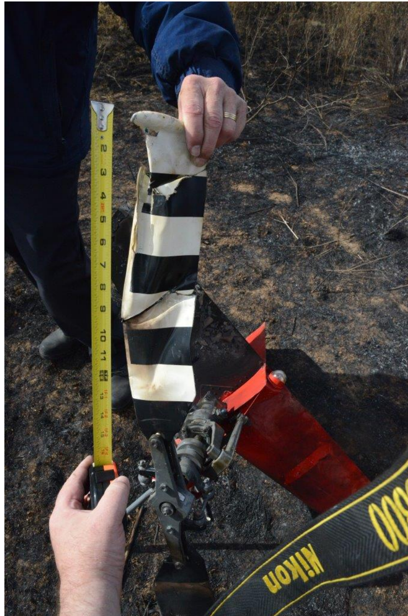
Photo 15 - View of a tail rotor blade with its liberated blade tip.
