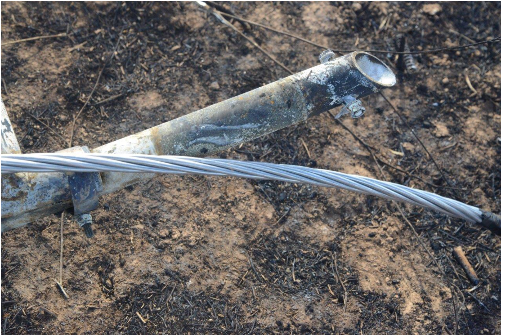
Photo 14 - View of a crosstube with a witness mark and an exemplar section of powerline.
