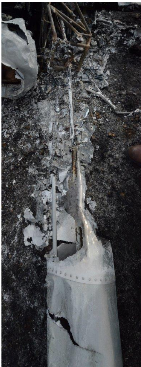
Photo 3 - View of a section of tailboom that was consumed by fire.
