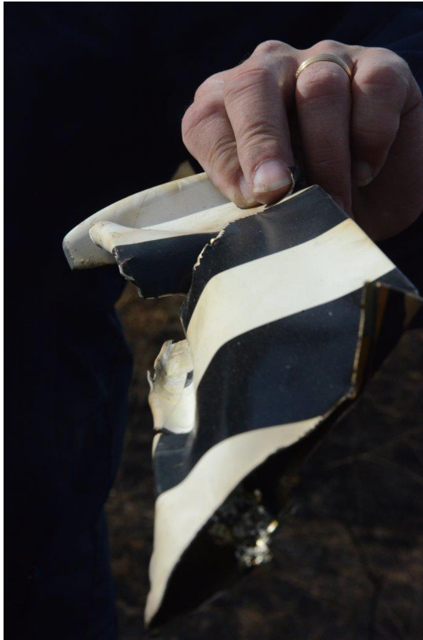
Photo 16 - Side view of a tail rotor blade with its liberated blade tip.
