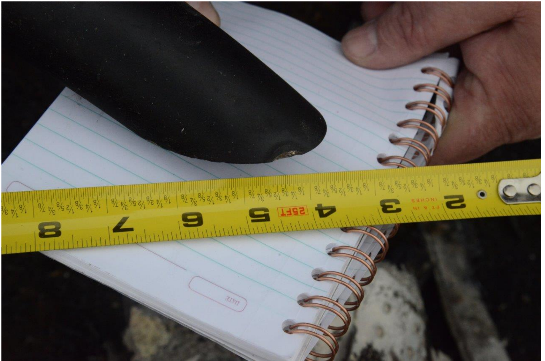
Photo 13 - View of a skid tip with a semicircular witness mark.
