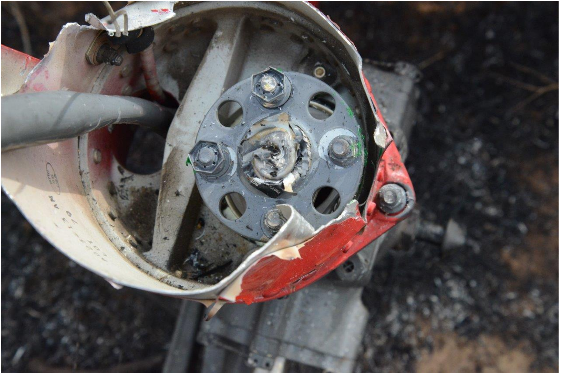
Photo 11 - Close up view of the tail rotor drive shaft.
