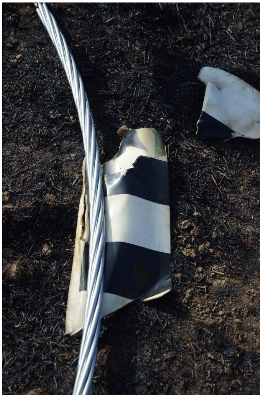
Photo 17 - View of a tail rotor blade with an exemplar section of powerline.
