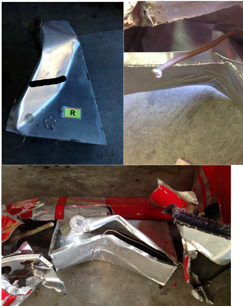
Photograph 9 – Right Auxiliary Fuel Tank
