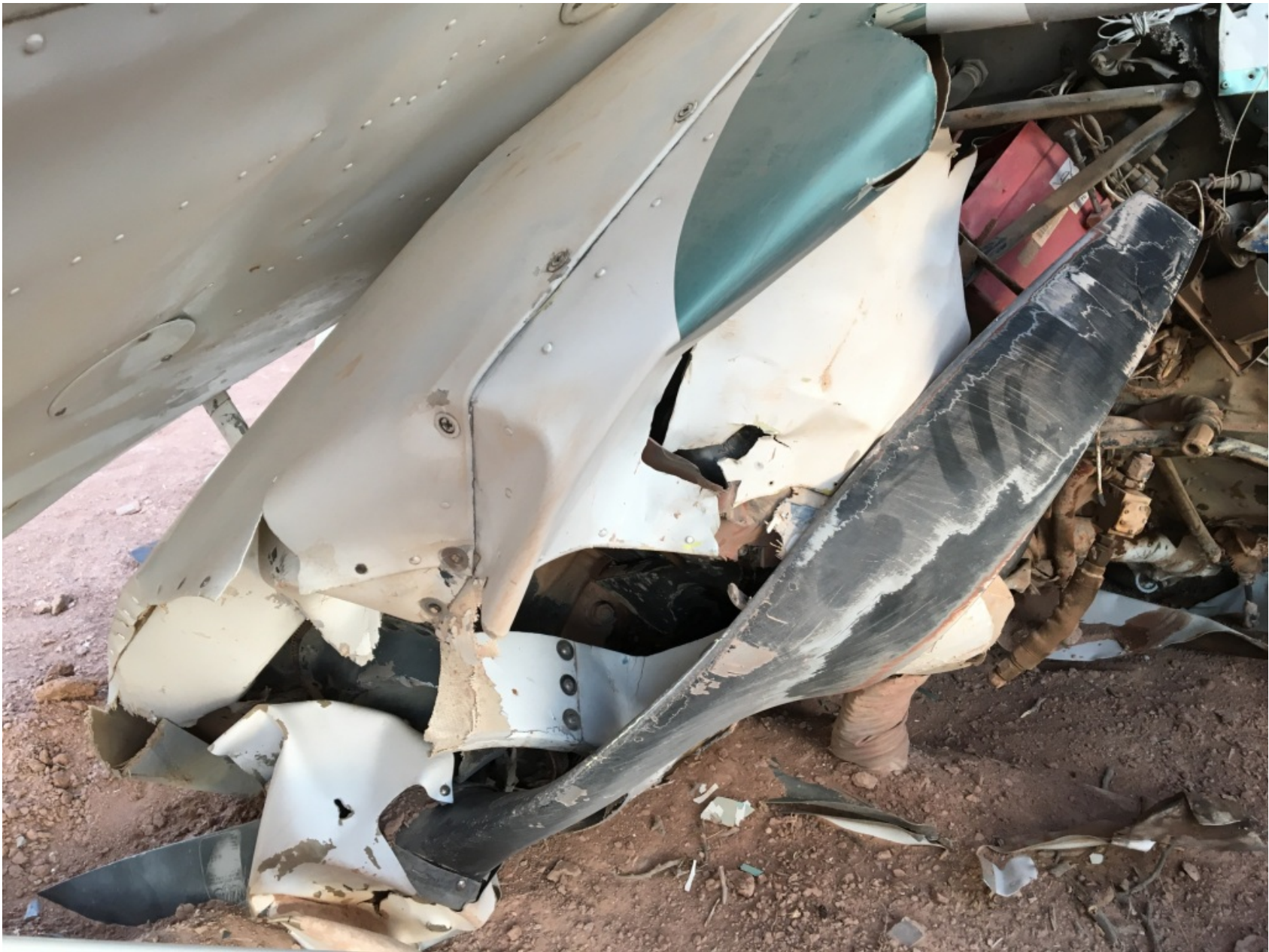
Photo 12 – View of the propeller still attached to the wreckage
