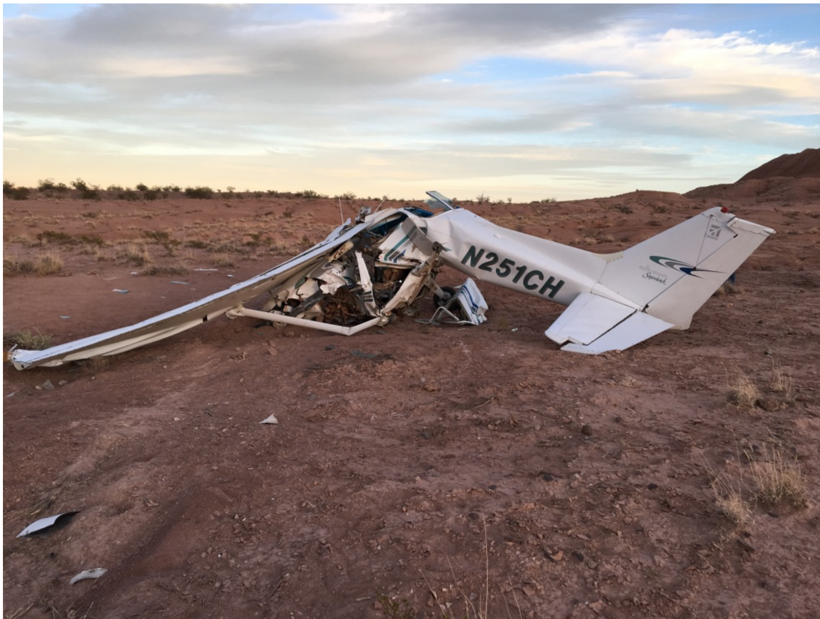
Photo 5 – A view of the left side the airplane with ground scars visible
