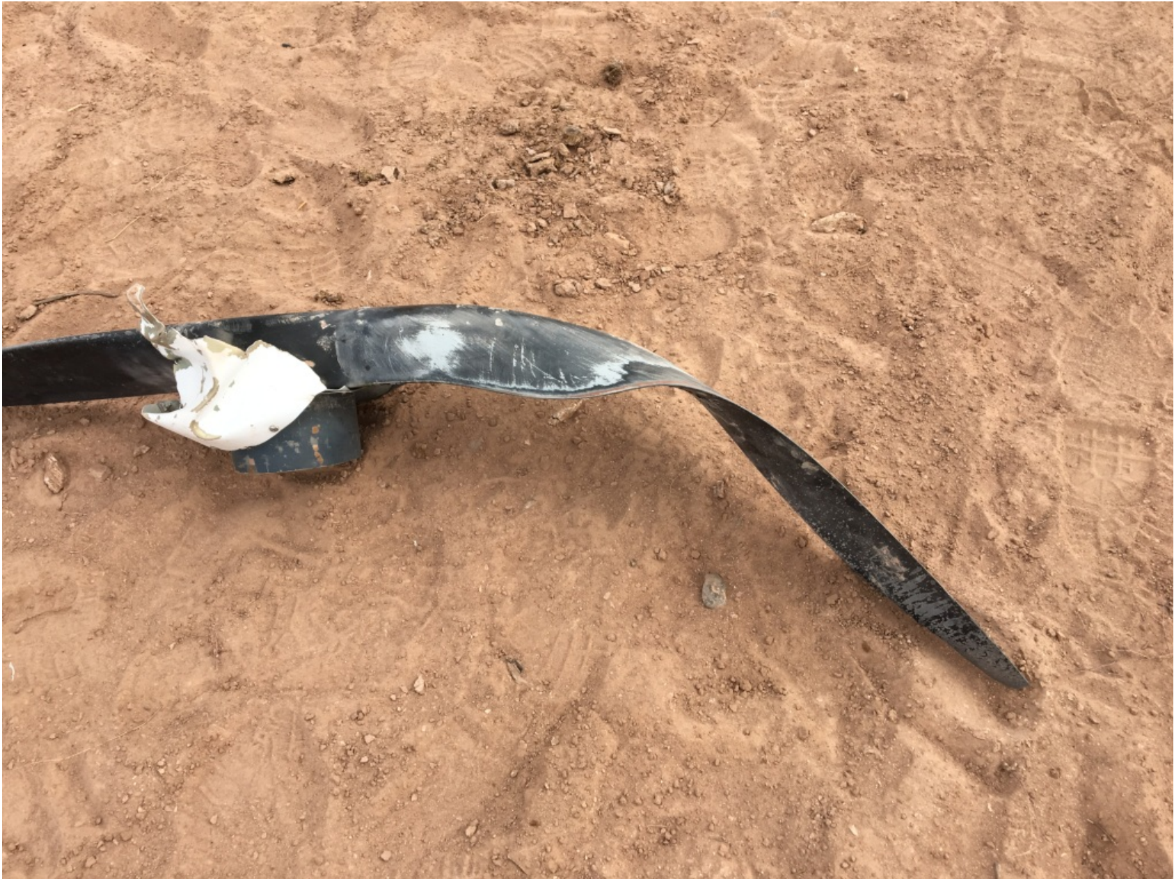
Photo 14 – A view of one of the propeller blades with blade twist and bending
