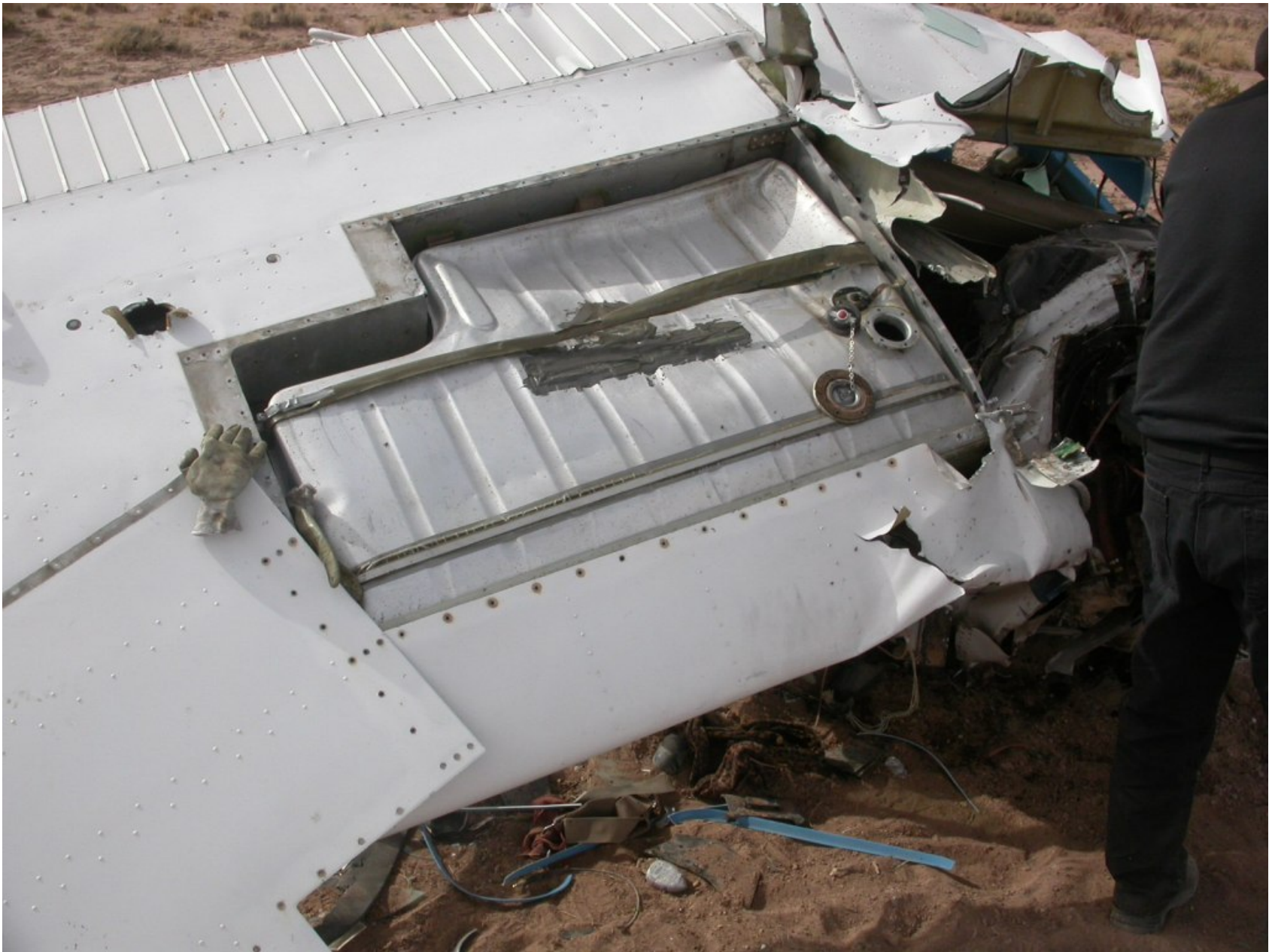
Photo 8 – View of the metal right wing fuel tank
