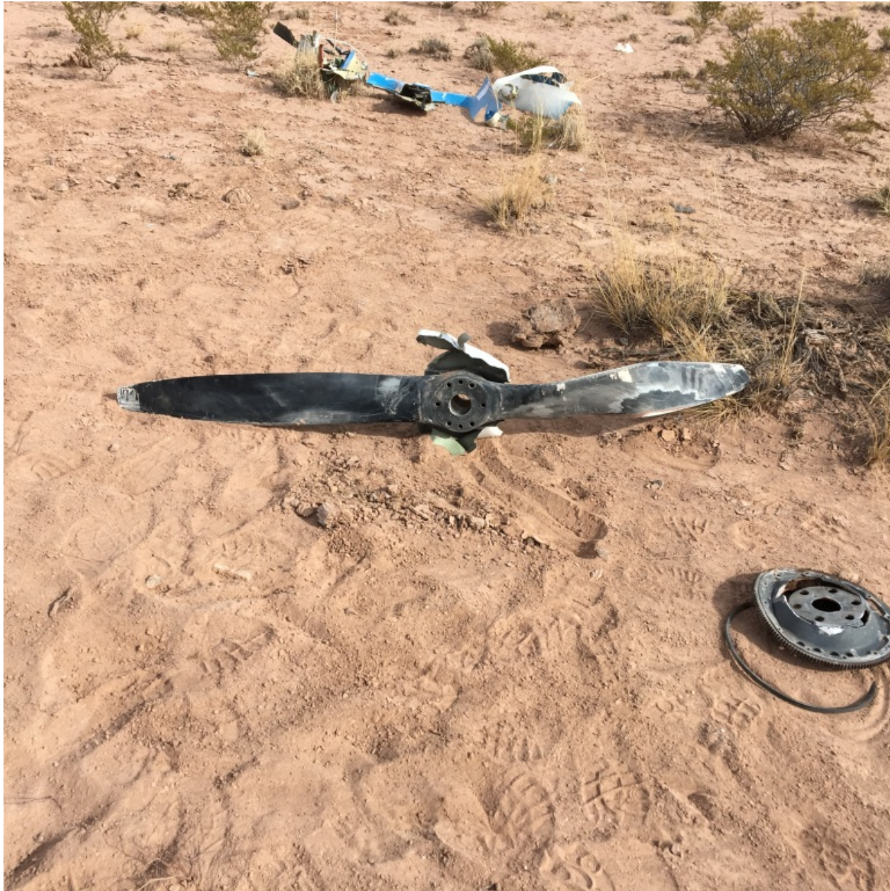
Photo 13 – A view of the propeller separated from the engine
