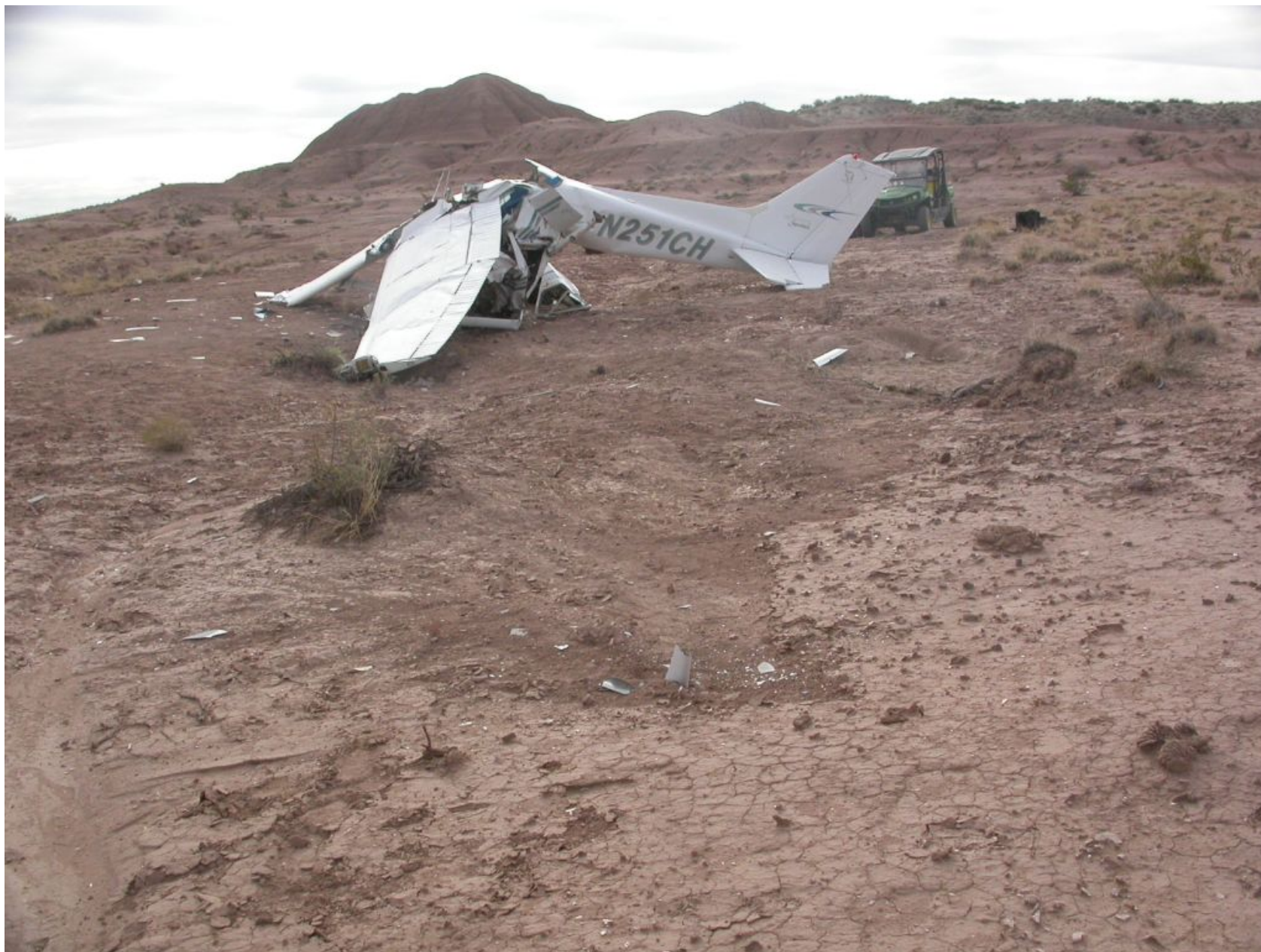
Photo 4 – View on ground impact marks on the left side of the airplane
