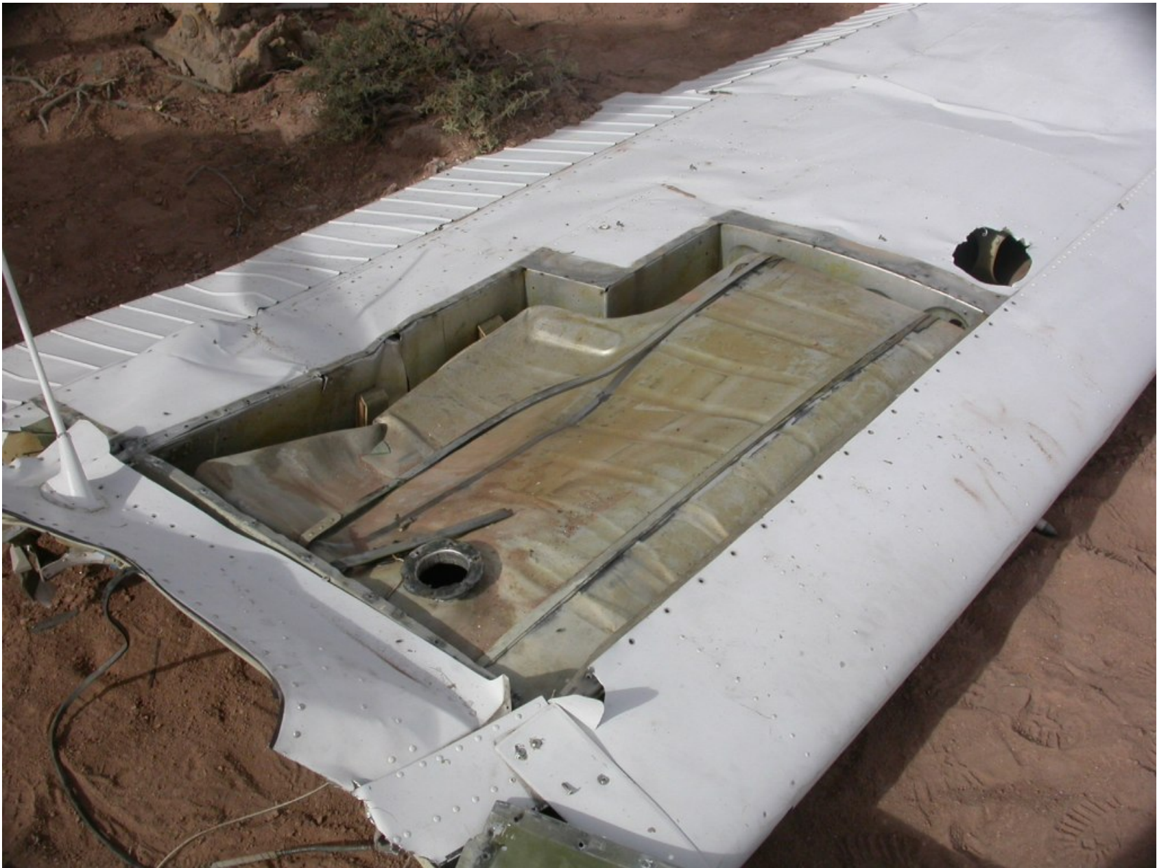
Photo 9 - Photo 9 – View of the metal left wing fuel tank
