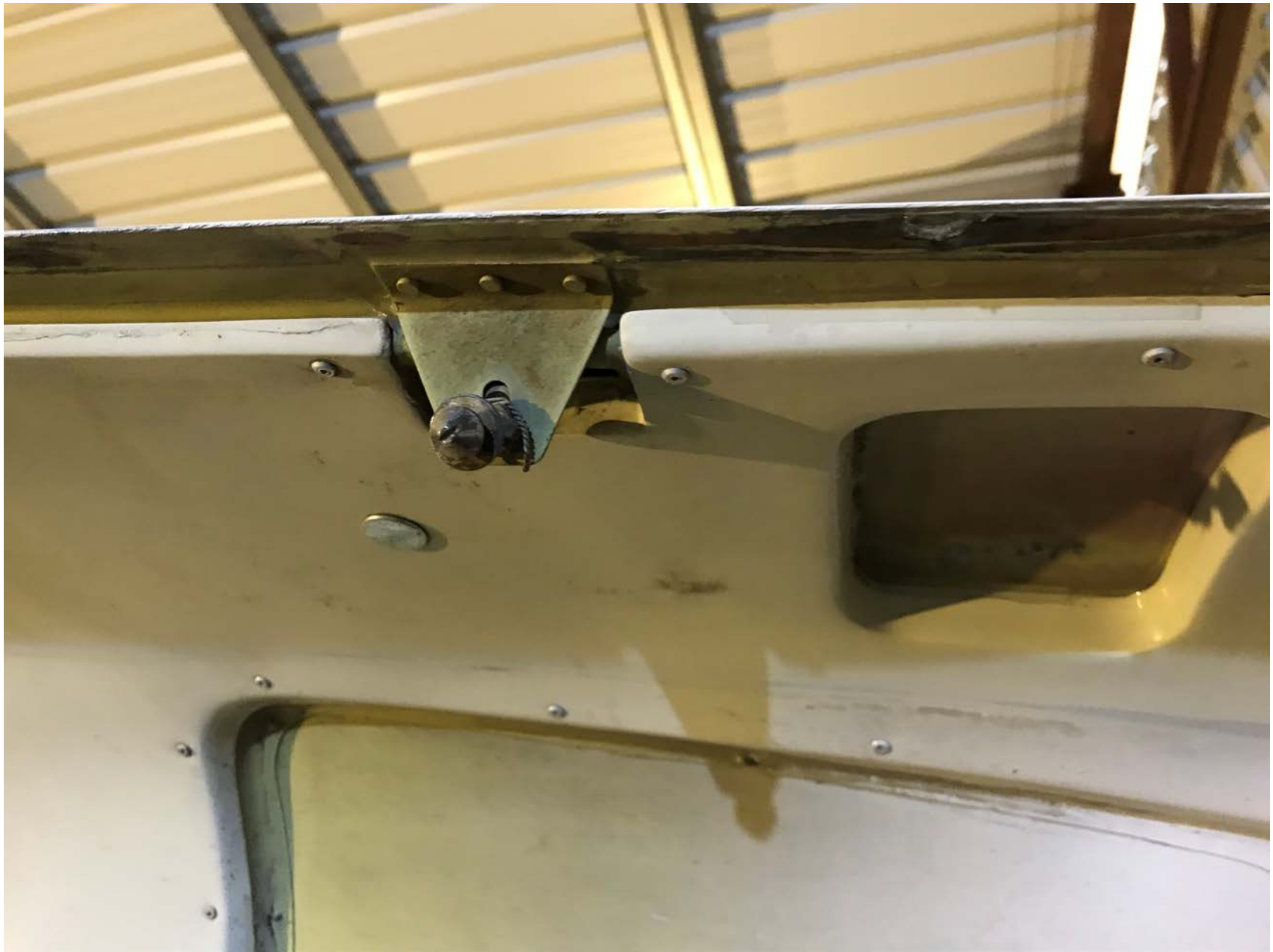
Photo 3 – Bayonet fitting with engine cowling open
