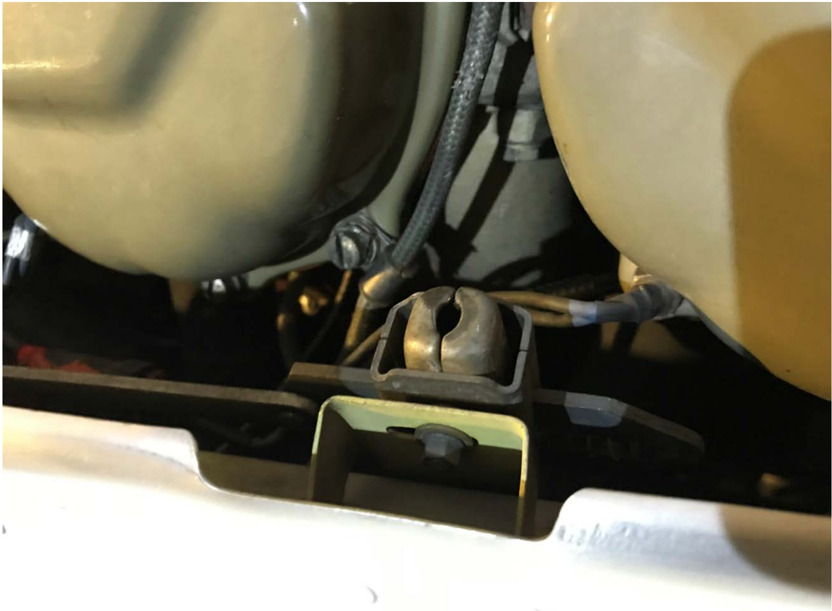
Photo 2 – Latch in the closed position (with engine cowling open)
