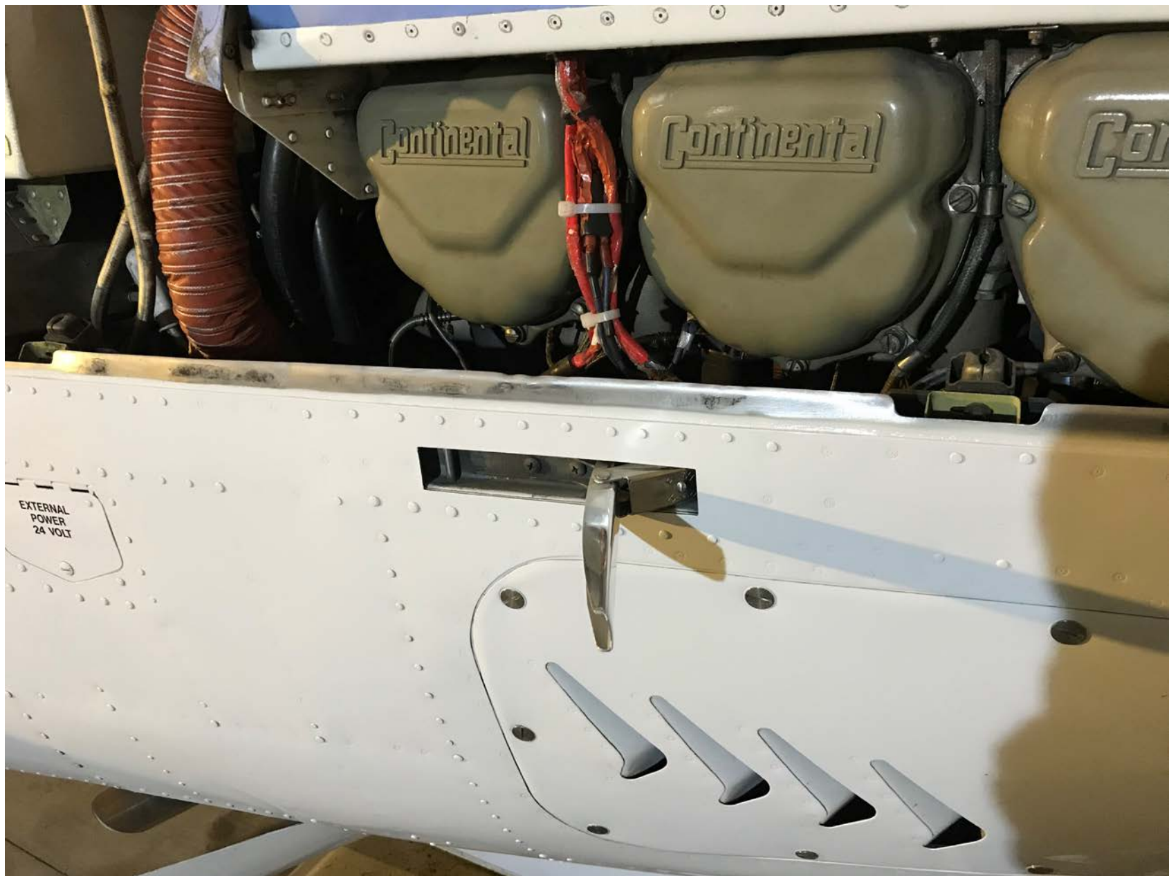
Photo 1 – Exterior Handle in the Open Position
