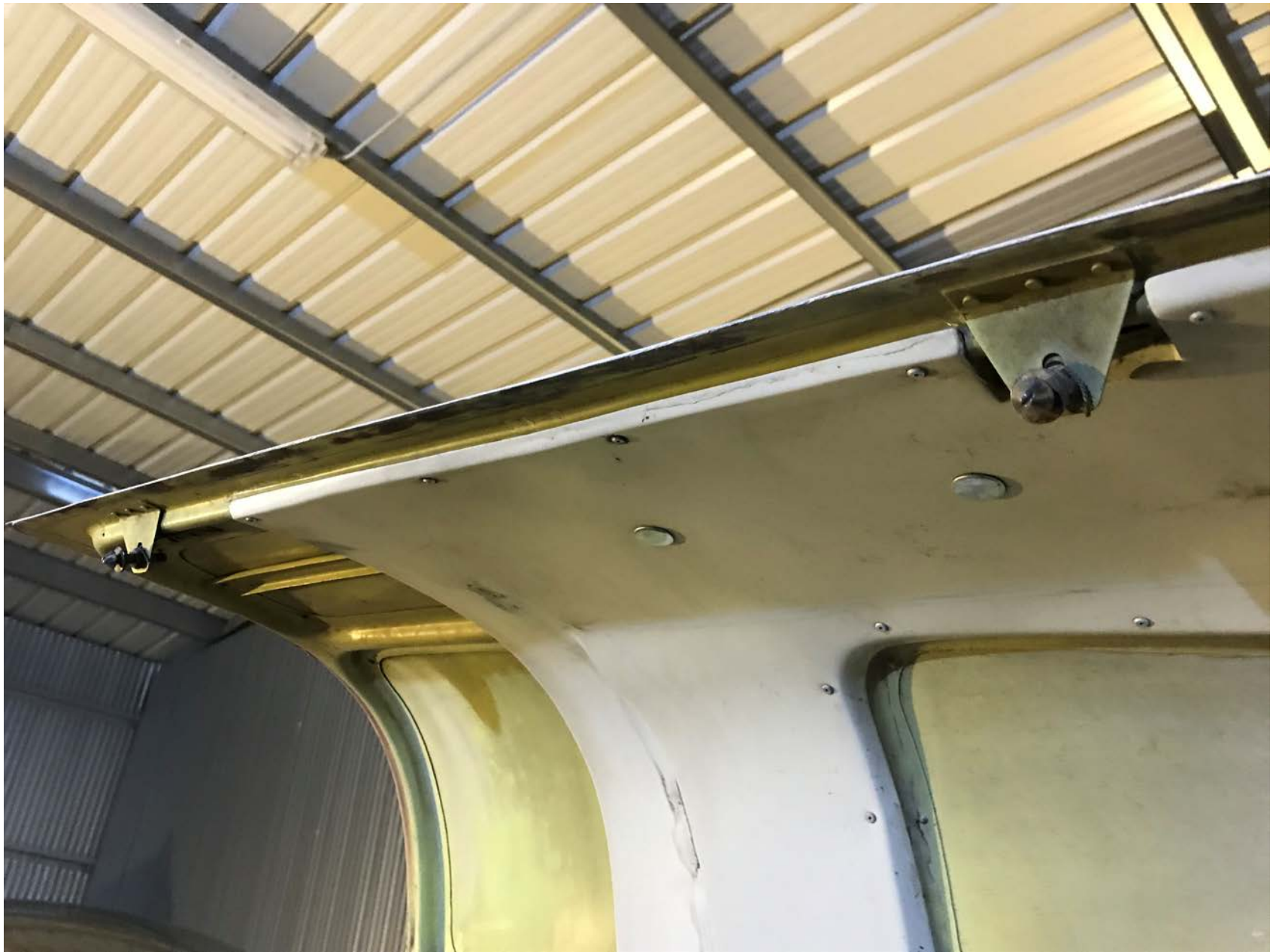
Photo 4 – Bayonet fittings with engine cowling open
