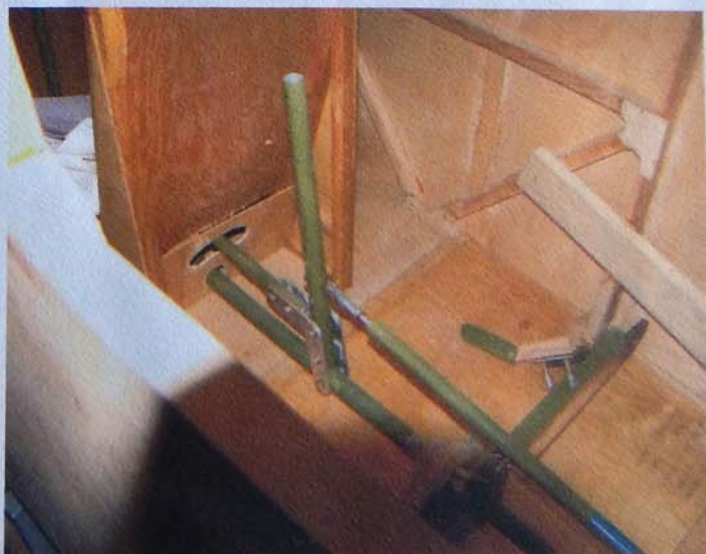
Fuel tank enclosure after glassing, prior to installation of the tank top.
