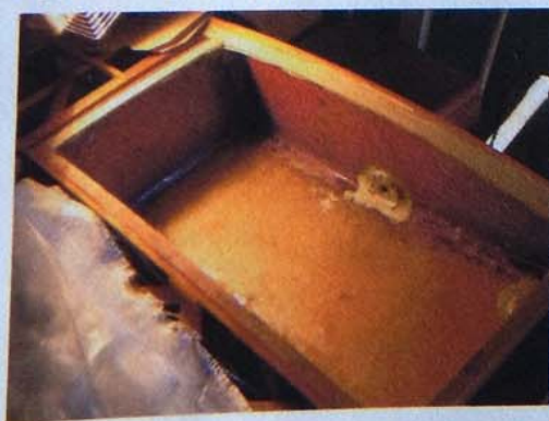
Fuel tank enclosure after glassing, prior to installation of the tank top.
