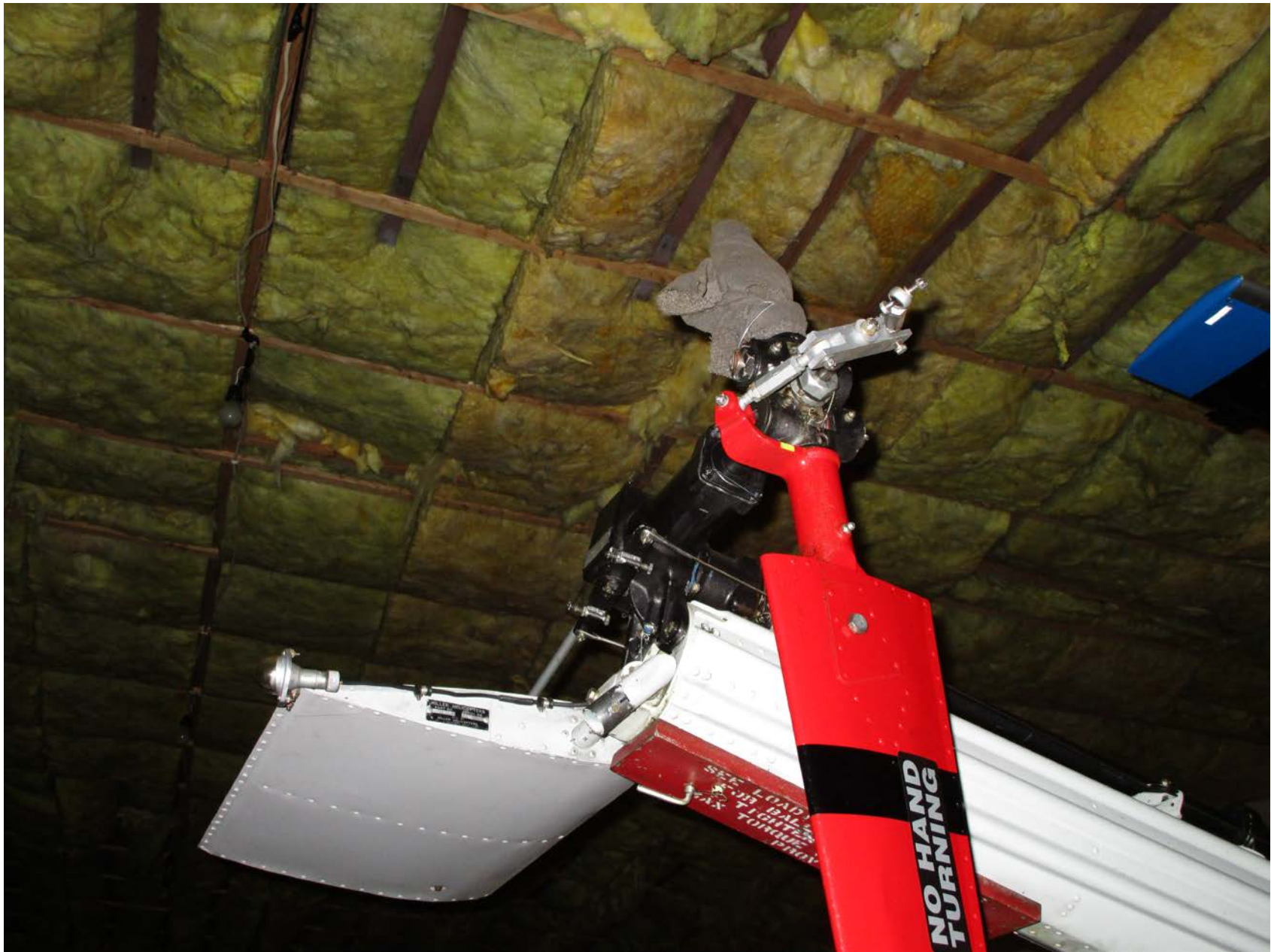
Photo 1 – Damaged Tail Rotor Assembly
