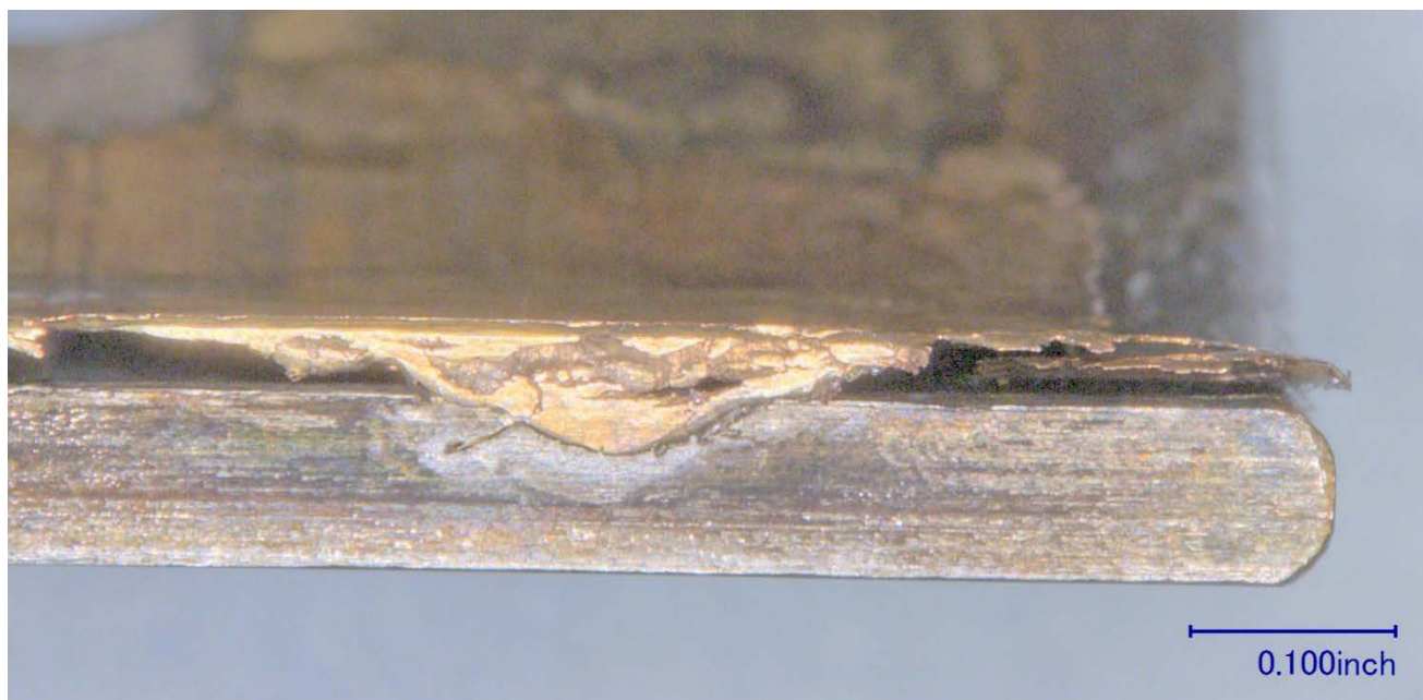
Figure 20 – The side of aft portion of Bearing A, showing material smeared over the bearing edge.
