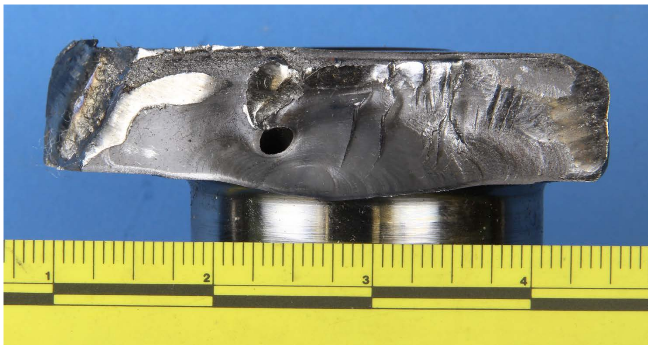
Figure 3 – View of the aft mating fracture surface of the crankshaft, as received.
