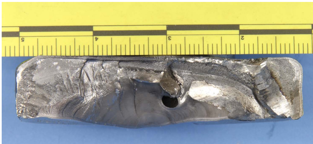
Figure 4 – View of the forward mating fracture surface of the crankshaft, after sectioning and cleaning with acetone.
