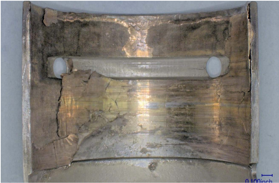
Figure 18 – The aft side of the internal surface of Bearing A, showing circumferential wear and material smearing and spalling.
