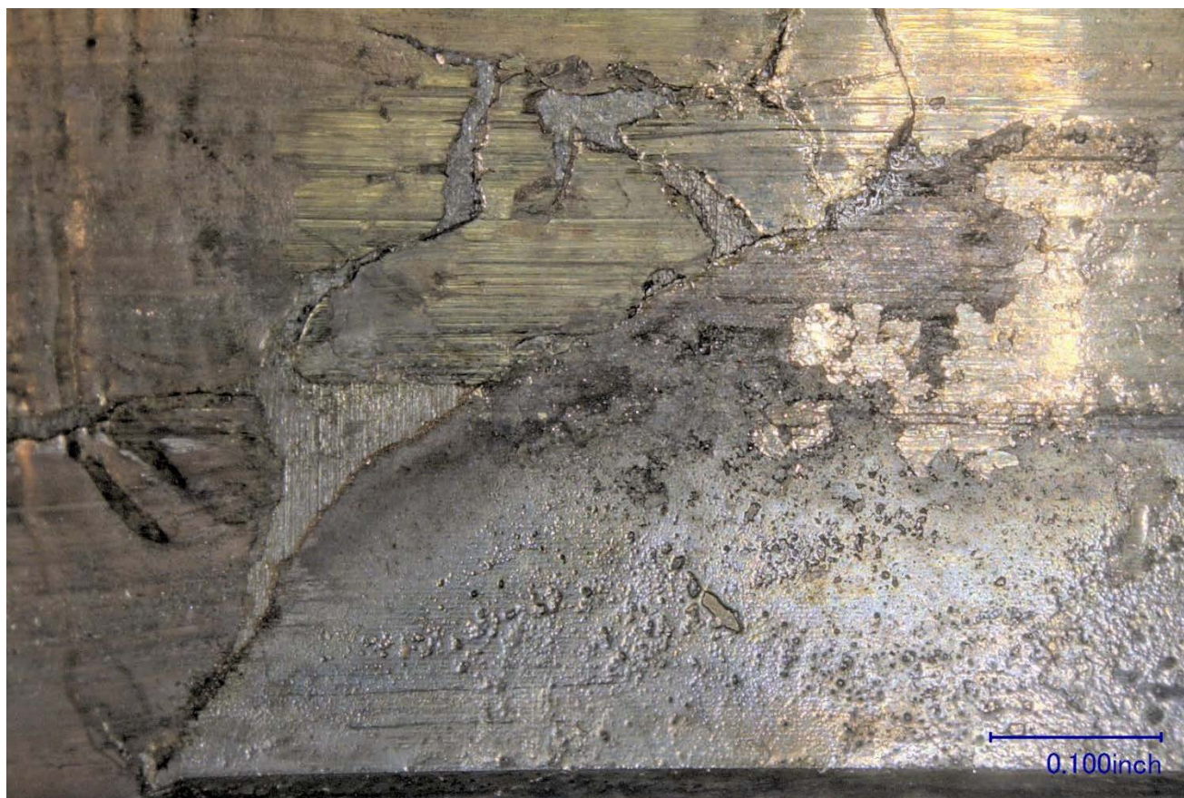
Figure 21 – Closer view of the smearing damage, spalling, and fatigue cracking on the aft side of the Bearing A internal surface.
