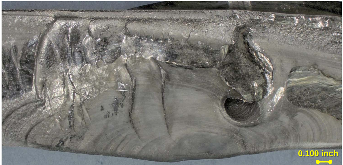
Figure 5 – Closer view of the crack initiation site of the forward fracture surface in Figure 4.
