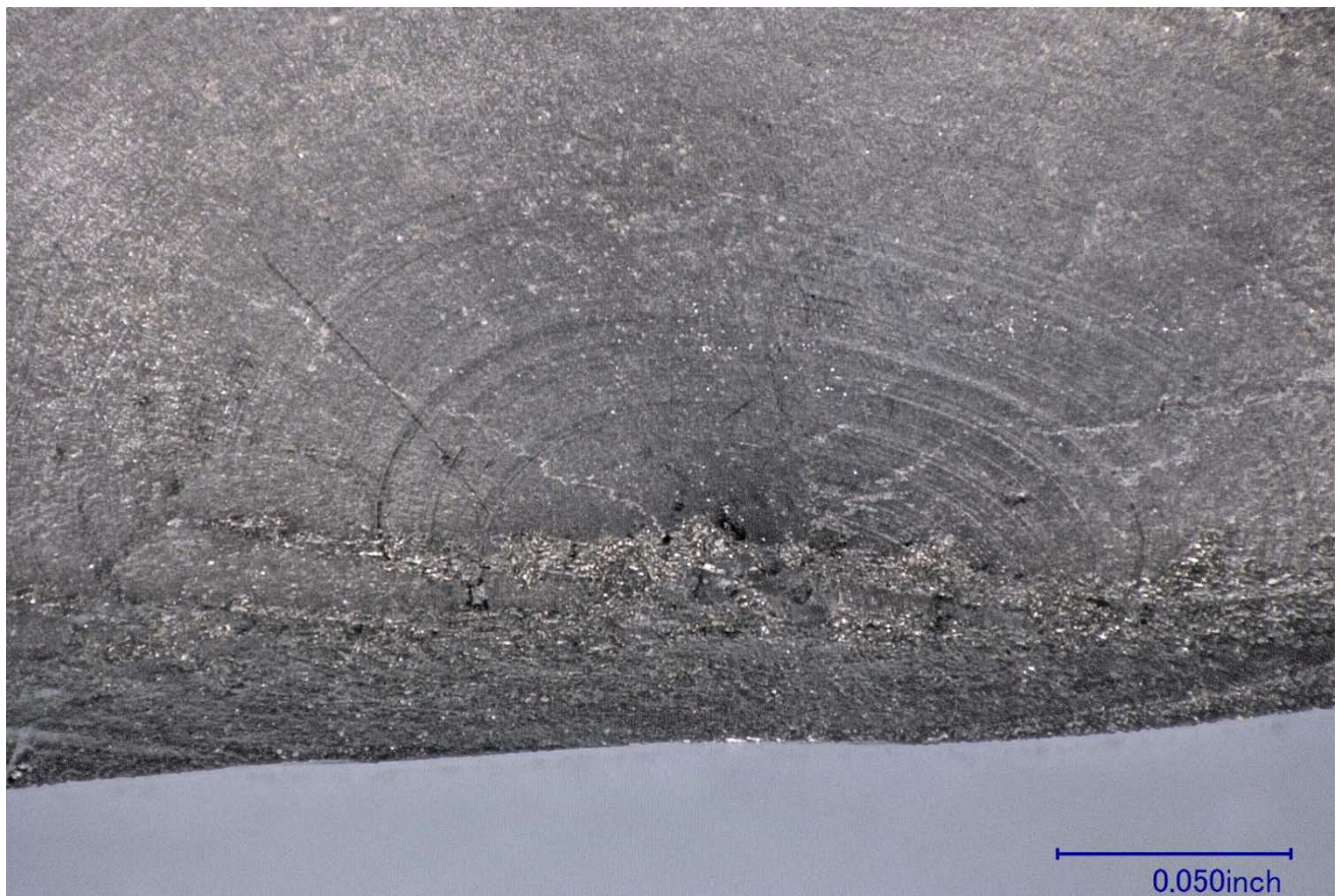
Figure 6 – Closer view of the crack initiation site from Figure 5.
