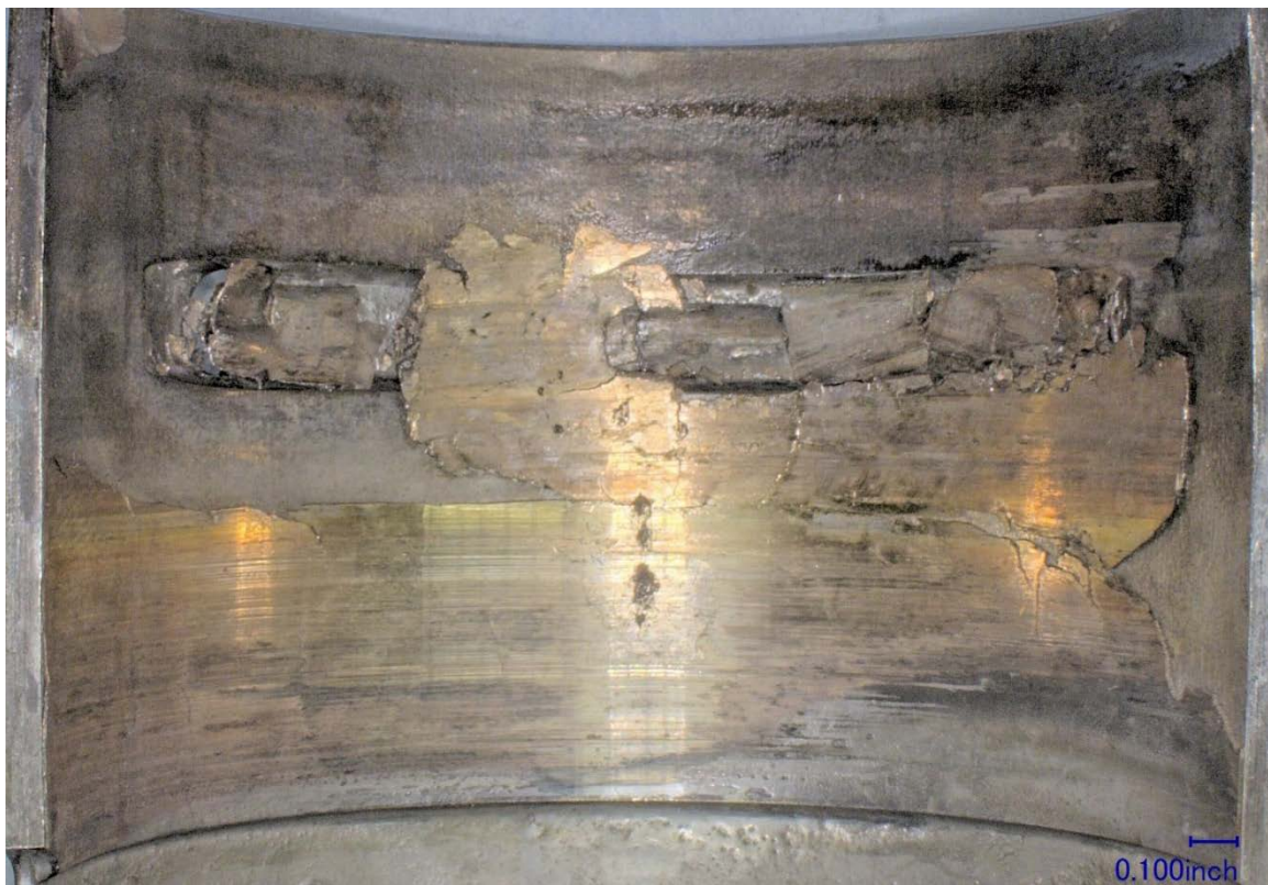
Figure 23 – The aft side of the internal surface of Bearing B, showing circumferential wear and material smearing and spalling.
