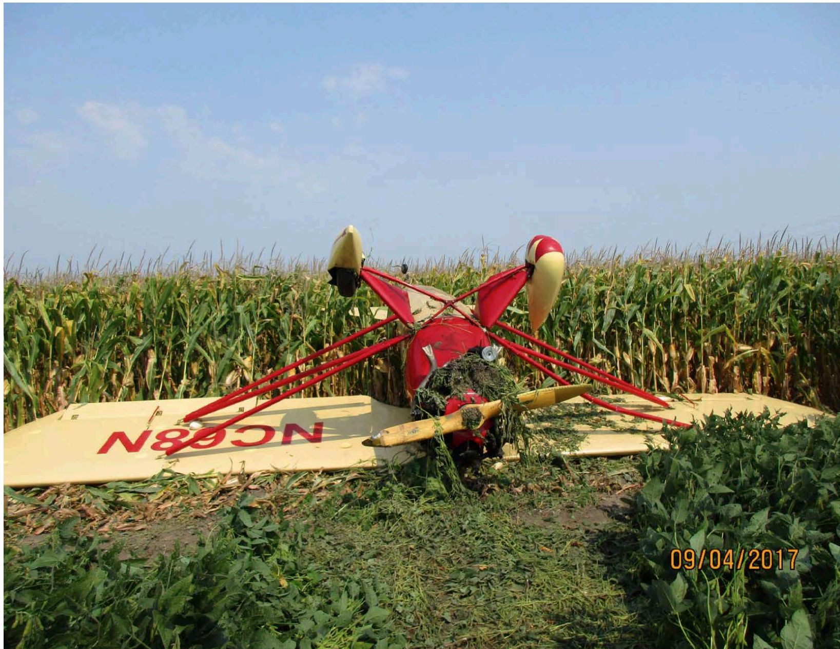
Photo 1 – Inverted NC68N in the cornfield after its forced landing. Note vegetation wrapped around engine cowling.
