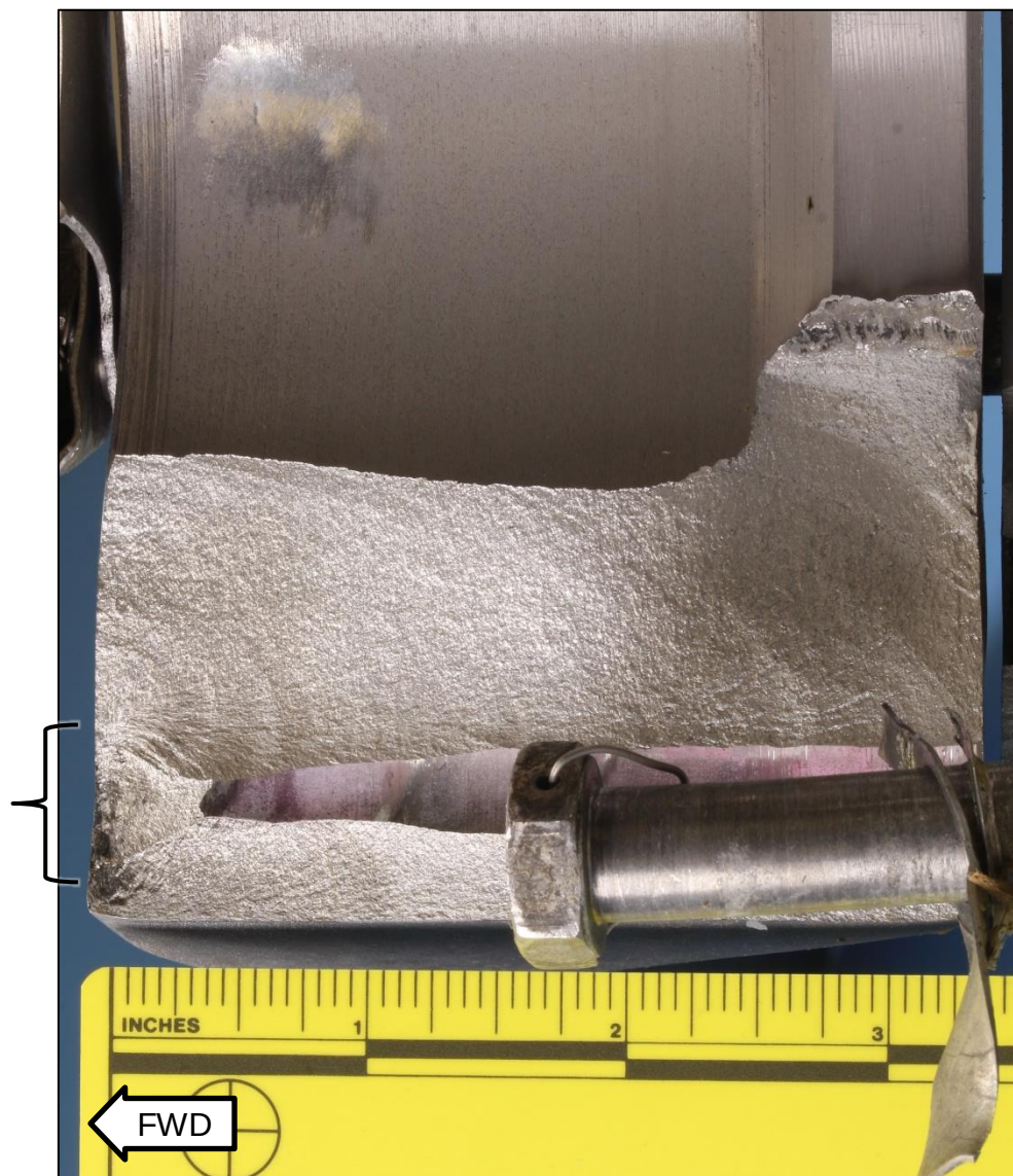
Figure 6. Blade 2 side of the fracture at bolt 5. A bracket indicates the area of multiple origins located at the forward face of the propeller.
