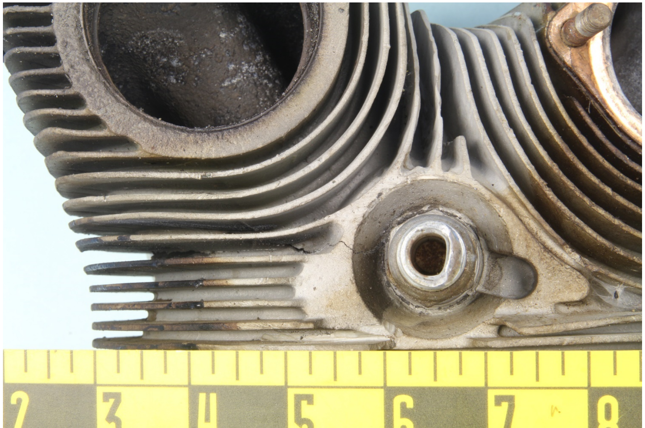
Figure 4 – View of the aft spark plug, showing denting damage and the end of the crack between two cooling fins.
