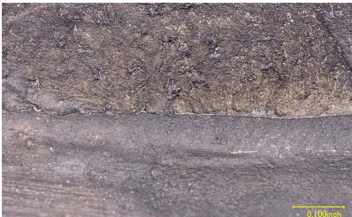
Figure 15 – Closer view of the crack initiation sites tilted at an angle, showing the cooling fin valley.
