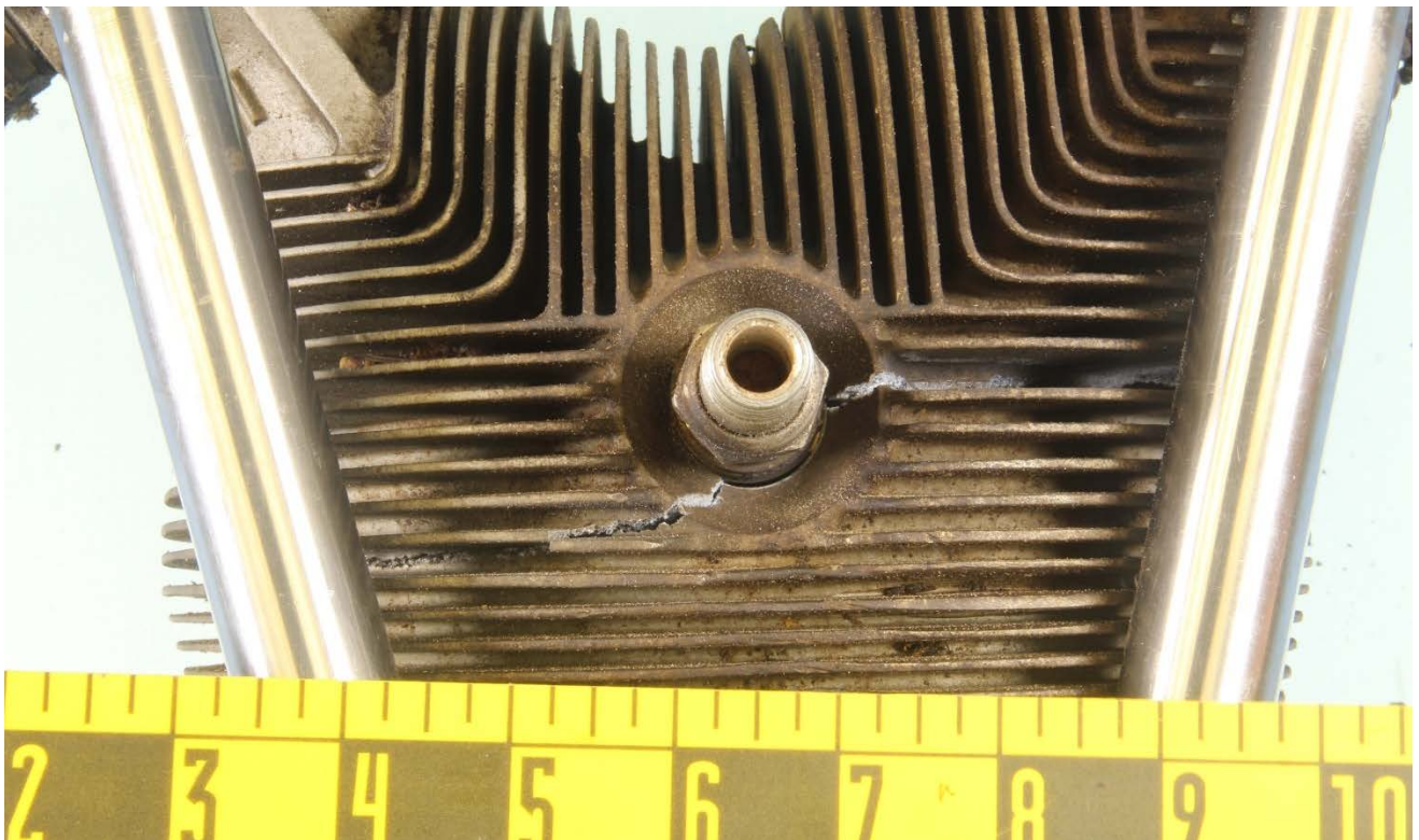
Figure 6 – The cylinder crack, viewed from the forward side (or rotated 90 from Figure 5).
