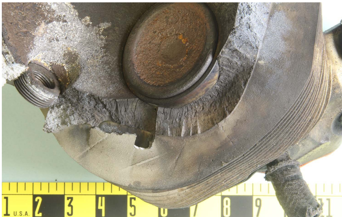
Figure 10 – The progressive area of the outboard fracture surface, using oblique lighting.
