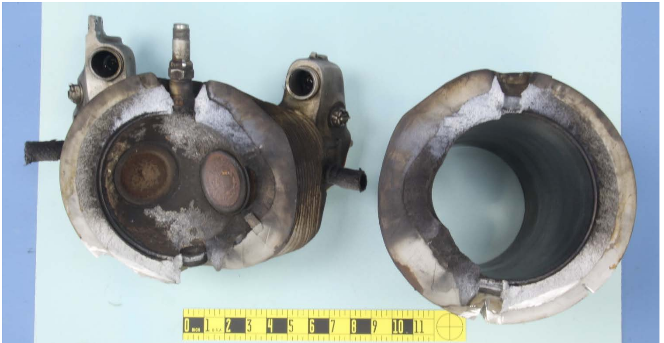
Figure 8 – View of the fracture surfaces of the cylinder crack, after laboratory opening.
