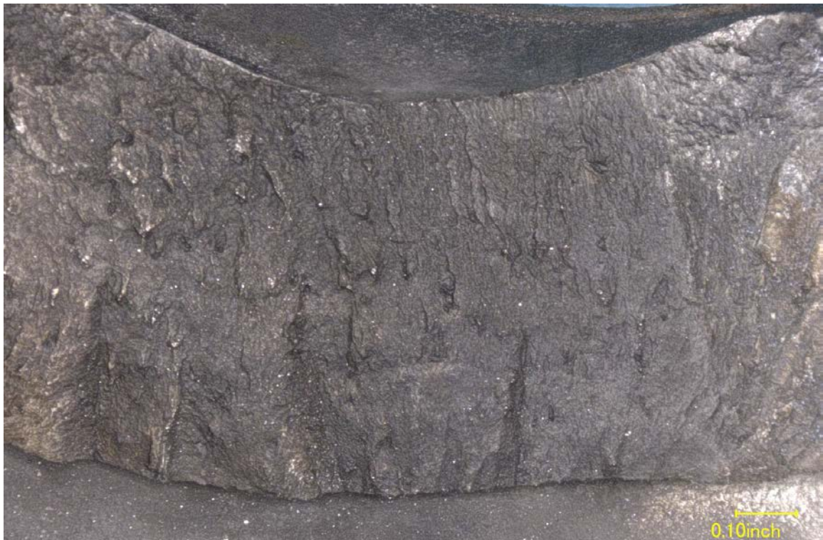
Figure 14 – Closer view of the crack initiation sites, showing ratchet marks and crack arrest marks.
