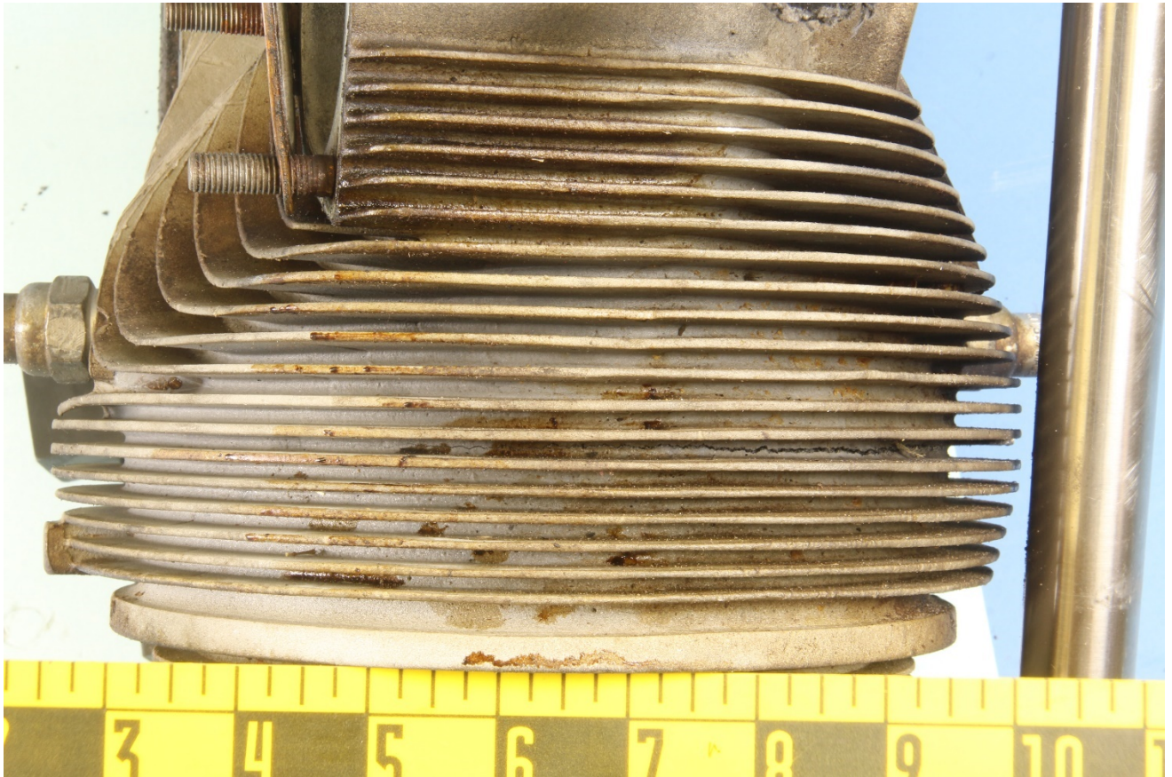
Figure 7 – View of the other end of the cylinder crack, rotated 90° from Figure 6.
