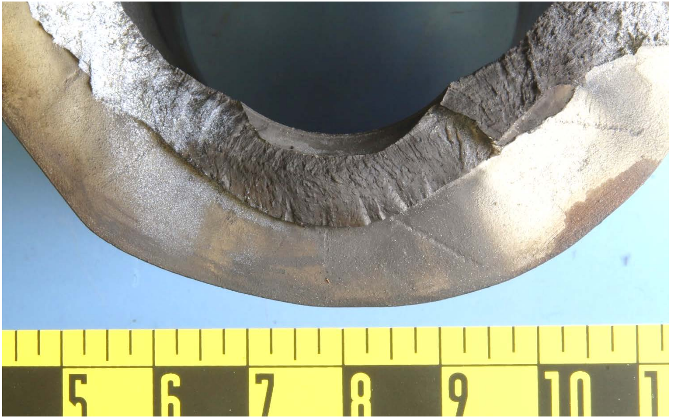
Figure 13 – The fatigue area of the outboard fracture surface, using oblique lighting.
