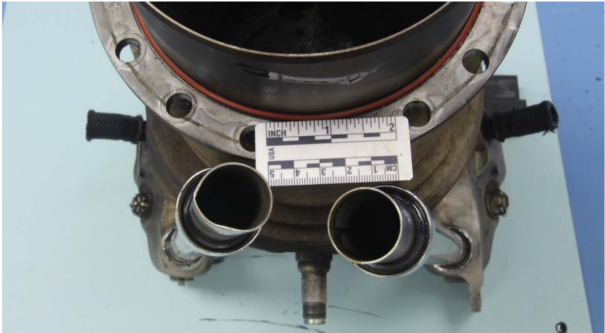
Figure 3 – The pushrod tubes on the forward side of the engine, showing denting damage.
