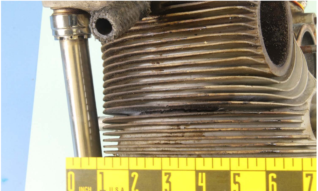
Figure 5 – The crack in the cylinder, rotated 90 from Figure 4, showing the largest opening.
