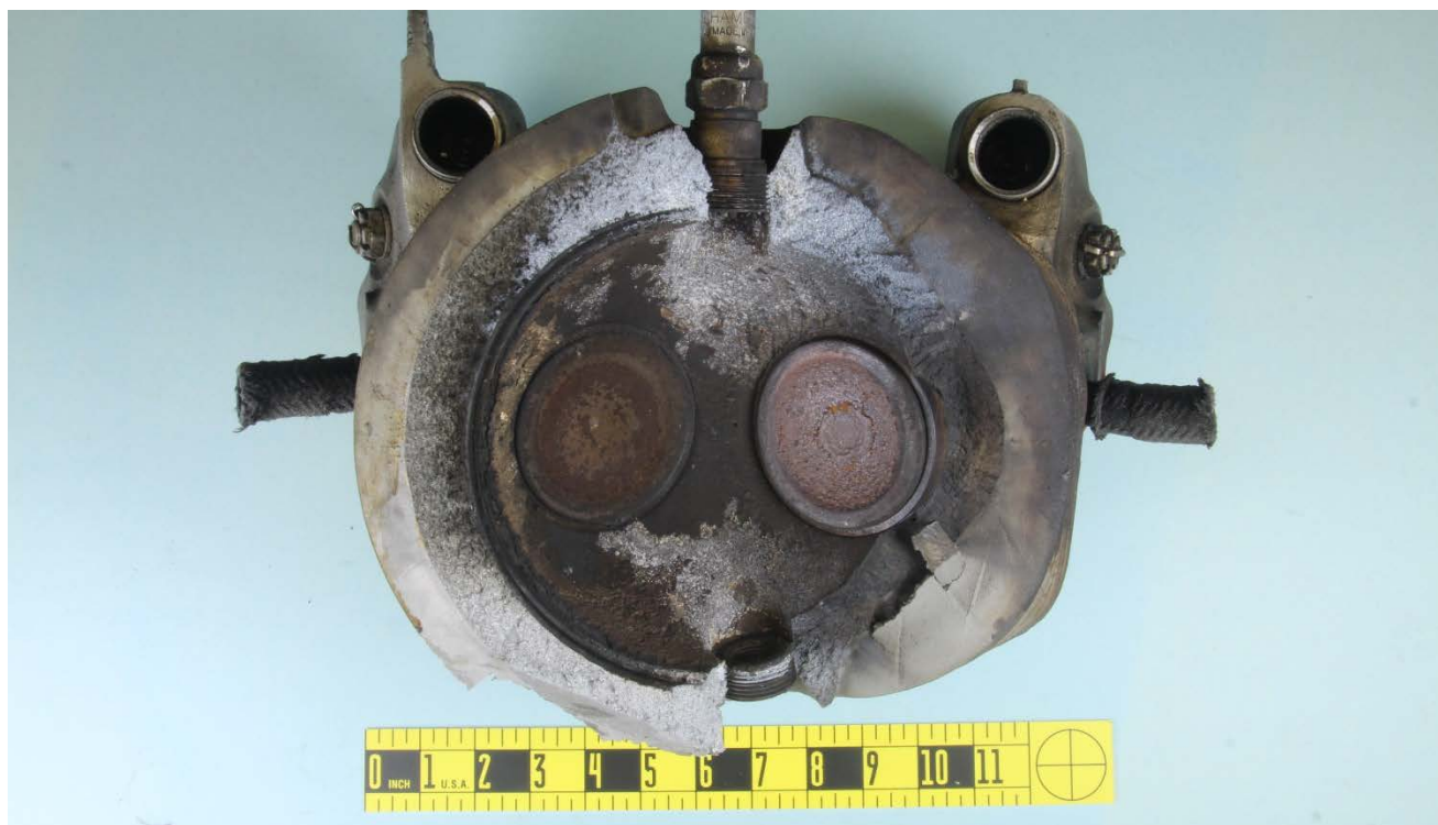
Figure 9 – The outboard mating fracture surface, annotated to show the different fracture regions.
