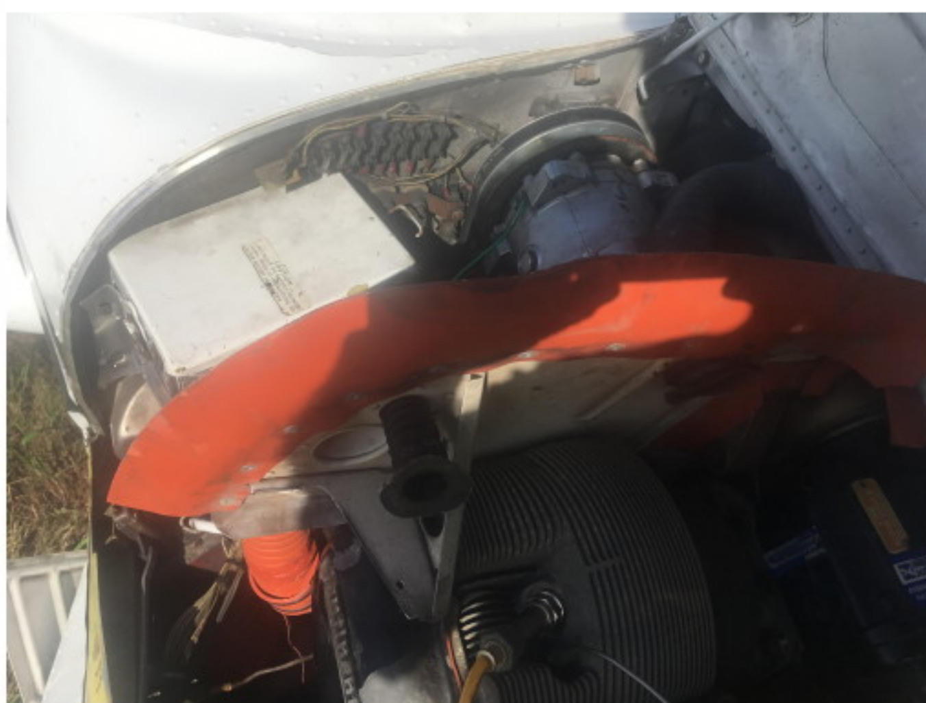
Firewall and all supporting structure crushed inward
