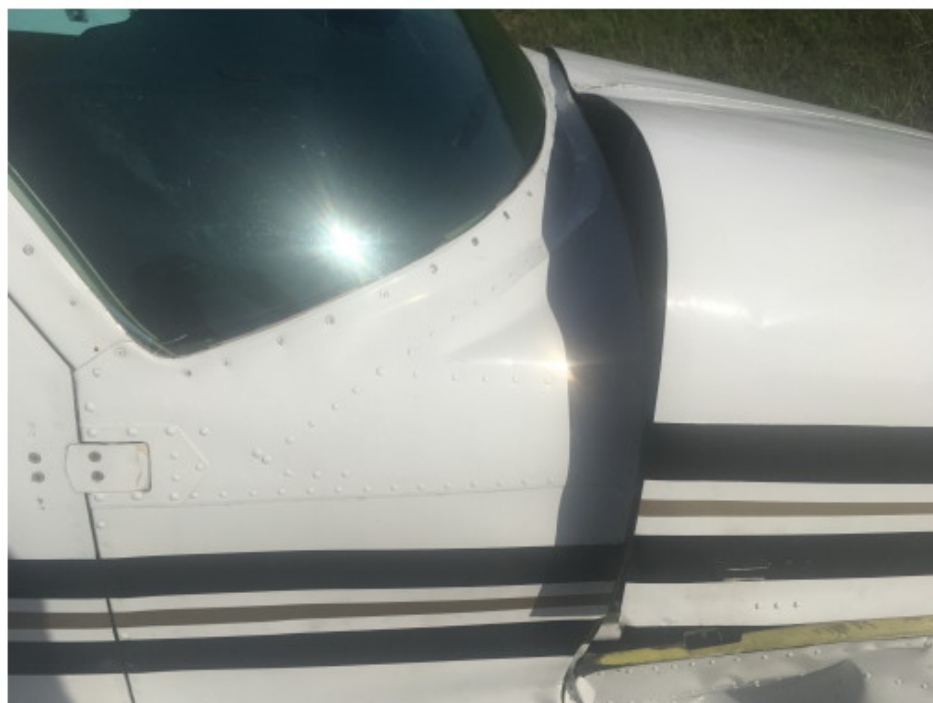
Boot cowl crushed
