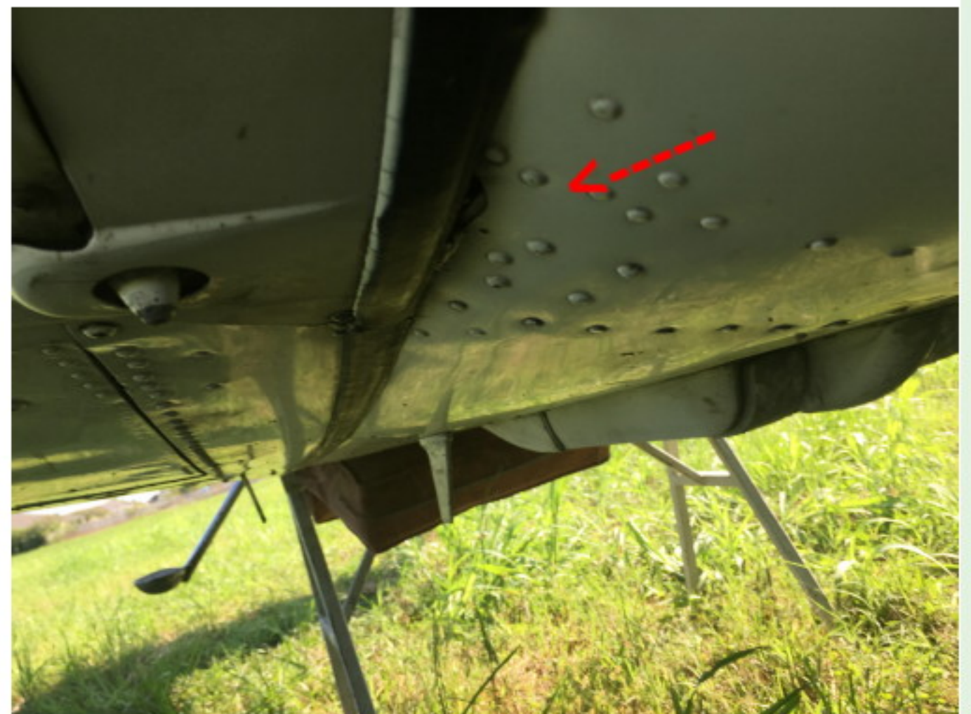
Buckle in fitting support structure
