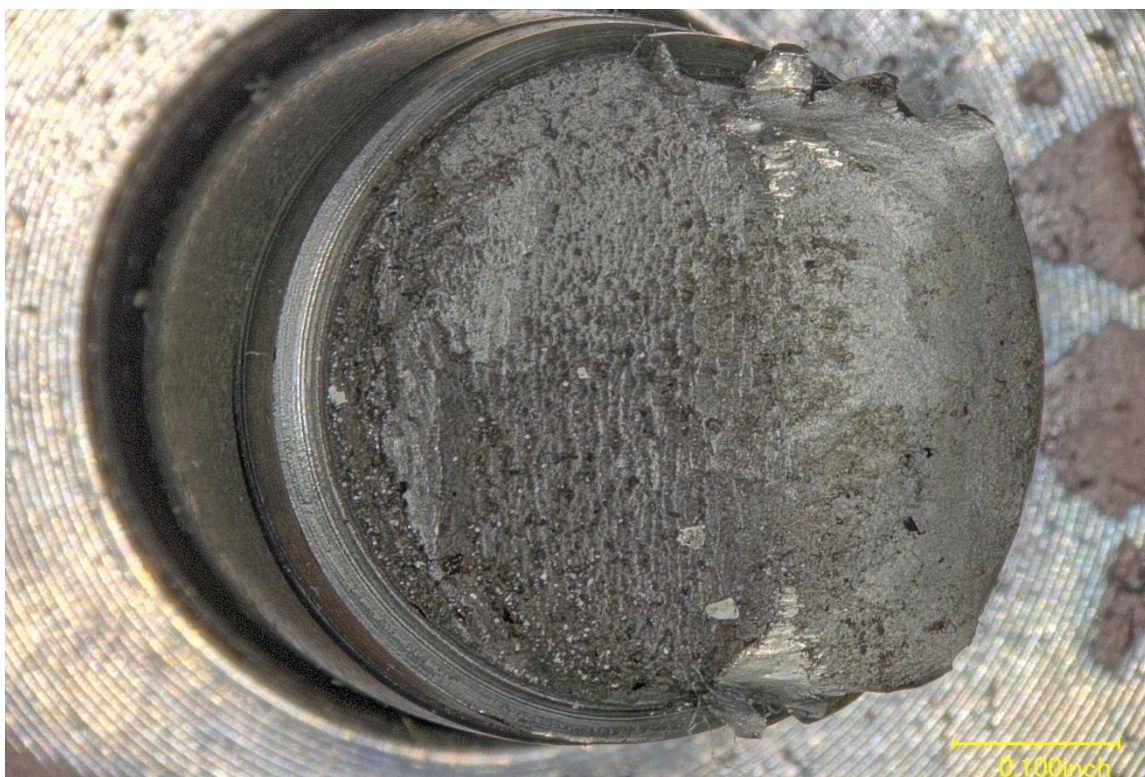
Figure 11 – Closer view of the piston rod fracture surface, with arrows showing the fracture direction.
