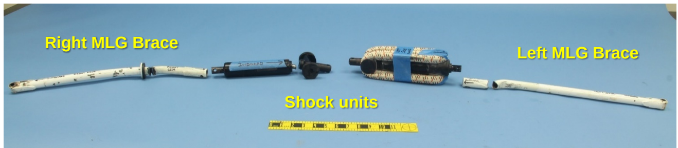
Figure 1 – The left and right main landing gear braces and the shock units, as received.
