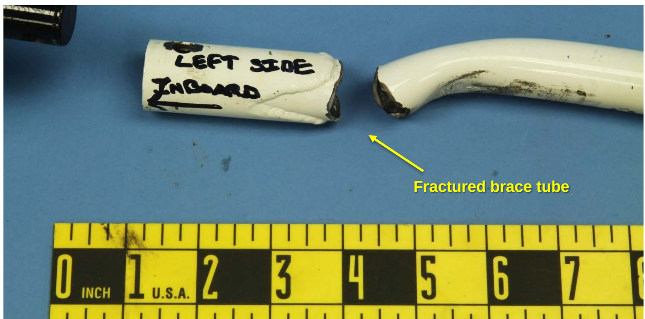
Figure 3 – The fractured left brace tube fragments, as received.
