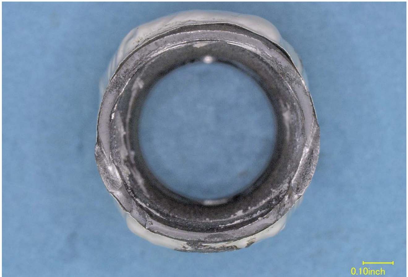
Figure 4 – The inboard fracture surface of the left landing gear brace.
