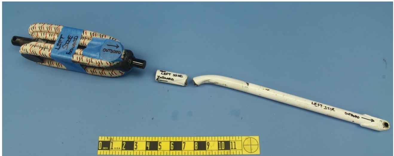
Figure 2 – The left side shock unit and main landing gear brace, as received.
